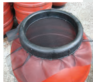
For barrels with a removable lid, unscrew the retainer ring and separate it from the inner lid, place screen over barrel opening, replace just the retainer ring to hold the screen in place, and trim excess screen material around the outside of retainer ring.
