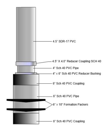
GEOHYDROLOGIC DATA PACKER ASSEMBLY PLAN THORNHILL RANCH LFA 1 MONITOR WELL
