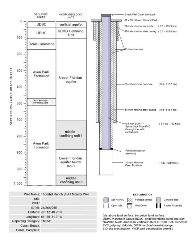
Figure 4 Diagram for the 4.5-inch x 10-inch Packer Assembly
