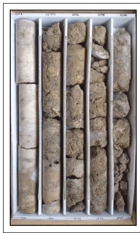
Description: 1590-1600 - Brown dolostone (crystalline). Poorly (1592-1600) to well indurated (1590-1592). Intensely fractured and highly dolomitized 1592-1600. Moldic and pinpoint porosity, sucrosic texture with vugs from 1592-1600. Sandy seams from 1592-1600. Bivalves.
