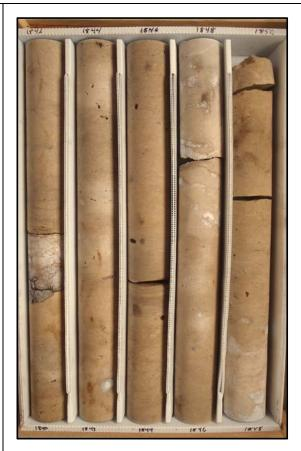
Description: 1840-1850 - Light brown to brown dolostone (crystalline) with medium bedded white to opaque gypsum and anhydrite 1840.7-1841. Lignite laminations at 1840.7 and 1841. Well indurated, very low perm., low poros. Intercrystalline porosity, little moldic poros. Voids infilled with gypsum and anhydrite. Slightly fractured, horizontal fractures 1847.5-1848.75, gypsum and anhydrite infilled. Apparent natural breaks at 1841 and 1844.75. Some horizontal laminations 1844.25-1845.25.
