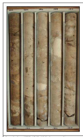
Description: 1800-1810 - Light brown to brown dolostone (wackestone-crystalline) with medium bedded white to opaque gypsum and anhydrite 1808.1-1808.8, thinly bedded 1804.7-1804.8. Well indurated, low permeability and porosity. Moldic porosity. Massive to somewhat sucrosic from 1800-1802.5. Some shell 1800-1802, bivalves. Voids infilled with gypsum and anhydrite. Apparent natural breaks at lignite laminations at 1804.15 and 1808.25.
