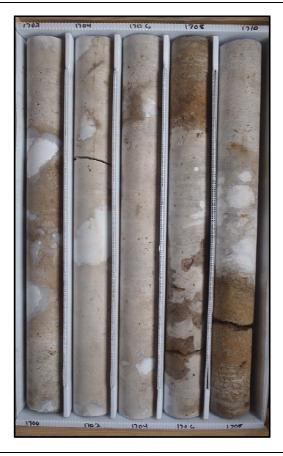
Description: 1700-1710 - Light brown to gray dolostone (crystalline) with thinly bedded white to opaque gypsum and anhydrite 1701.3-1701.5. Well indurated, low permeability. Moldic and intercrystalline porosity, massive. Horizontal and vertical fractures 1701 and 1709.75, gypsum and anhydrite infilled. Voids infilled with gypsum and anhydrite.
