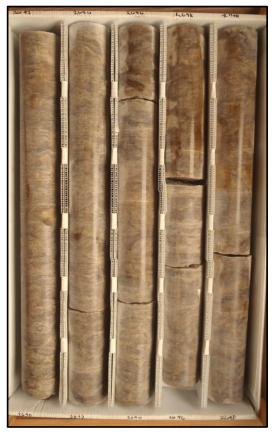
Description: 2690-2700 - Thickly bedded light brown to gray dolomitic finely crystalline anhydrite with some white gypsum laminations throughout. Irregular bedded light brown dolomitic limestone (mudstone) laminations throughout. Well indurated. Granular to massive texture. Slightly to moderately fractured. Very low porosity and permeability. Fracture and intercrystalline porosity.
