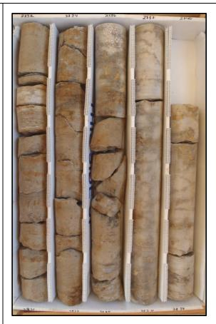
Description: 2830-2840 - 2830-2835.5 Thickly bedded light brown dolomitic limestone (mudstone), 2835.5-2840 laminated to medium bedded white-light brown-light to dark gray dolomitic anhydrite and gypsum (irregular bedding). Mod. to well indurated. Moderately to intensely fractured. Low to v. low porosity and perm. Fracture, intergranular, intercrystalline and little moldic porosity. Some nodular and void infilling gypsum and anhydrite 2830-2835.5.
