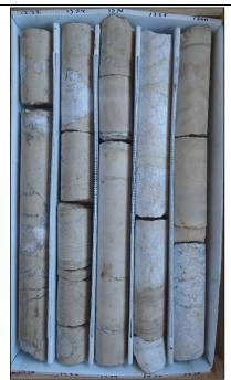
Description: 1330-1340 - Light brown dolomitic limestone (1330-1331.5 wackestone, 1331.5-1340 mudstone). Moderately well indurated, low permeability. Moldic and intergranular porosity with gypsum infilling. White to opaque gypsum seams and thin beds from 1330-1334, medium bedded at 1336, highly fractured with gypsum infilling 1336.5-1338, medium bedded from 1338-1339.
