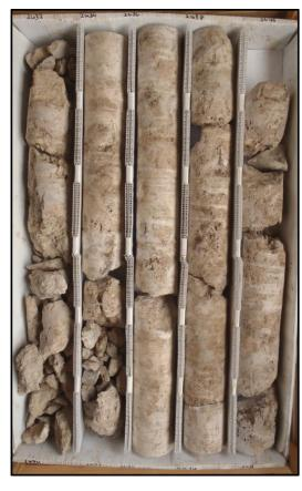
Description: 2630-2640 - Tan to light brown thickly bedded dolomitic limestone (mudstone to wackestone). Granular texture, moderately well indurated. Moderately fractured, fracture zone 2630-2631 and 2631.75-2633. Moderately low porosity and permeability. Fracture, moldic, intergranular and some pinpoint porosity. Some vugs and secondary porosity developed 2630-2633 and 2637-2640.
