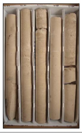
Description: 2180-2190 - Tan to light brown limestone (wackestone). Moderately well indurated, granular texture, somewhat chalky. Moderately low permeability and porosity. Intergranular and some moldic porosity, slightly fractured. Some bivalves and bivalve molds. Some gray-green clay (glauconitic) at 2180.75.
