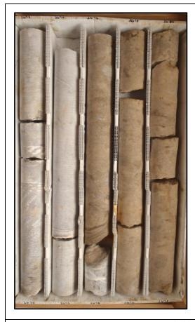
Description: 2670-2680 - 2670-2674.25 thickly bedded light brown-gray-white anhydrite with some light brown dolomitic infilling irregular fractures and voids, 2674.25-2680 light brown dolomitic limestone (mudstone). Mod. well to well indurated. Granular to massive texture. Somewhat brecciated 2674.25-2680 with gray-white-opaque gypsum and anhydrite infilling primary/secondary poros. Very low porosity and permeability.
