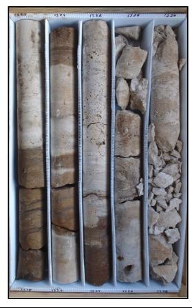
Description: 1520-1530 - Brown dolostone (wackestone-crystalline) 1520-1526, light brown to gray dolomitic limestone 1526-1530. Poorly to well indurated, low to moderate permeability. Moldic and pinpoint porosity, some vugs and somewhat sucrosic 1520-1524.5. Intensely fractured 1526-1530. Lignite laminations 1520-1521.
