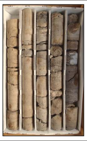
Description: 2540-2550 - Thickly bedded light brown to gray dolomitic limestone (mudstone-wackestone), gray med. bedded dolostone 2548.5-2549.25 and med. bedded white to opaque gypsum and anhydrite 2549.2-2549.4. Poorly to mod. well indurated. Granular to crystalline texture. Mod. to intensely fractured, fracture zone at 2546. Mod. low poros. and perm. Fracture, moldic and intergranular porosity. Some vugs and secondary porosity developed 2545-2549.
