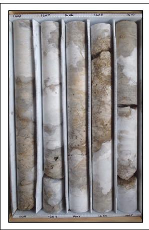
Description: 1600-1610 - Brown to gray dolostone (crystalline) with thickly bedded white to opaque gypsum and anhydrite from 1601.5-1604.5 and 1607.75-1609.1, medium bedded from 1606.25-1606.75. Well indurated, low permeability. Pinpoint and intercrystalline porosity with somewhat sucrosic texture from 1606.75 to 1607.75.
