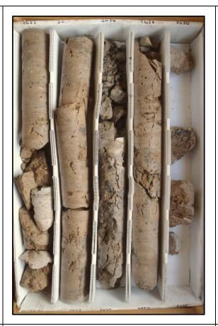
Description: 2620-2630 - Light brown to gray thickly bedded dolostone (mudstone-wackestone). Moderately well to well indurated. Granular to massive texture. Moderately to very intensely fractured, fracture zones 2620-2621.75 and 2625.75-2626.25. Some gray lean clay 2625-2626.25. Moderate porosity and permeability. Fracture, moldic and intergranular porosity. Some vugs and secondary porosity developed throughout.
