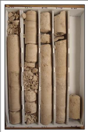
Description: 2170-2180 - Tan to light brown limestone (wackestone). Poorly to moderately well indurated, granular texture, somewhat friable and chalky. Moderately low permeability and porosity. Fracture and intergranular porosity, moderately to very intensely fractured Some gray-green/green clay at 2177.5-2180 (glauconitic/ glauconite). Dark brown lignite lamination at 2179.75.
