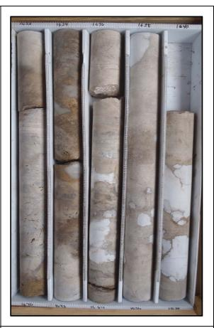
Description: 1630-1640 - Light brown to brown dolostone (crystalline) with medium bedded white to opaque gypsum and anhydrite from 1638.7-1639. Well indurated, low permeability. Intercrystalline and moldic porosity. Pinpoint porosity and somewhat sucrosic texture from 1633-1634. Horizontal and vertical fracturing and voids completely infilled with gypsum and anhydrite.
