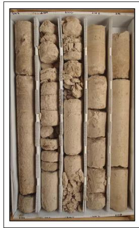
Description: 2100-2110 - Tan to light brown limestone (wackestone-packstone). Granular texture, poorly to moderately well indurated, somewhat friable. Intergranular and fracture porosity, moderately low permeability and porosity. Moderately to very intensely fractured. Some green clay (glauconite) at 2006.5.
