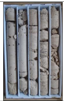
Description: 1280-1290 - Light brown dolomitic limestone (wackestone). Moderately well indurated, moderately low permeability. Moldic, intergranular and pinpoint porosity, some vugs from 1280-1281, some calcite and gypsum void infilling. Some horizontal laminations from 1285.5-1299.5. Poorly indurated seams of dolosilt at 1282.5 and between 1288.8-1299.5.
