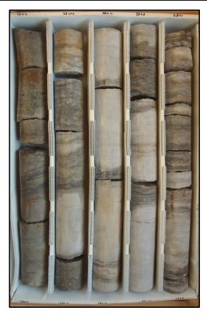
Description: 2800-2810 - 2800-2802.3 thickly bedded light brown to gray dolomitic limestone (mudstone), 2802.3-2810 thickly bedded gray to light brown dolomitic anhydrite with irregular bedding. Granular to massive texture. Moderately fractured. Moderately to well indurated. Low porosity and permeability. Fracture, intergranular and intercrystalline porosity, some moldic porosity. Some white gypsum laminations 2802.3-2810.
