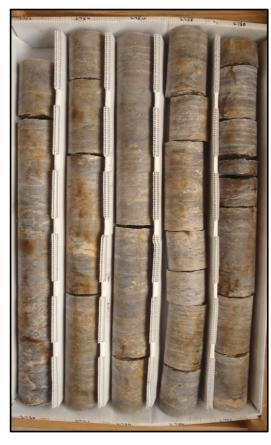
Description: 2750-2760 - Thickly bedded light brown to gray dolomitic finely crystalline anhydrite with some white gypsum laminations throughout. Irregular bedded light brown dolomitic limestone (mudstone) laminations throughout. Well indurated. Granular to massive texture. Slightly to moderately fractured. Very low porosity and permeability. Fracture and intercrystalline porosity.
