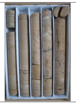
Description: 1430-1440 - Light brown dolomitic limestone (mudstone-wackestone). Moderately well indurated, low permeability. Moldic, pinpoint and intergranular porosity, gypsum infilling. Thinly bedded white to opaque gypsum at 1436.5. Lignite laminations from 1431.5-1433 and at 1439.2. Small vertical fracture <1 millimeter, infilled with gypsum from 1429-1429.2.
