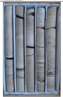
Description: 1340-1350 - Light brown dolomitic limestone (1340-1349 mudstone, 1349-1350 wackestone. Moderately well indurated, low permeability. Moldic, intergranular and pinpoint porosity with white to opaque gypsum infilling. White to opaque thin bedded gypsum at 1341, 1347.75 and 1348.5. Vertical fracture from 1343-1345.5 infilled with gypsum.
