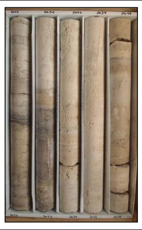
Description: 2030-2040 - Tan to light gray limestone (mudstone-wackestone) with light brown to gray dolostone from 2032-2033.1, somewhat dolomitic 2030-2032. Granular-chalky and massive texture. Moderately well to well indurated, low to moderately low perm. and porosity. Moldic, fracture and intergranular porosity. Somewhat soft and chalky 2033.25-2038.5. Some dark apparent solution surfaces (stylolites) and dark laminations.
