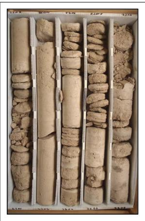
Description: 2200-2210 - Tan to light brown limestone (wackestone-packstone). Poorly-moderately well indurated, granular texture, somewhat chalky and friable. Moderately low permeability and porosity. Intergranular, fracture and some moldic porosity. Moderately to intensely fractured. Some fossil molds infilled with white to opaque gypsum 2208-2208.5. Dark, irregular stylolite and some thinly to medium bedded gray dolomitic limestone at 2209. Some bivalve molds.
