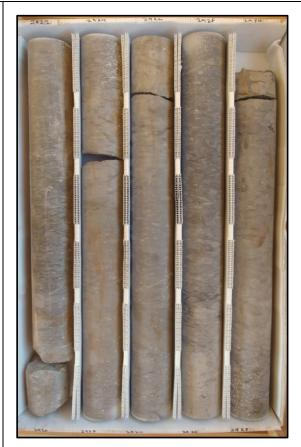
Description: 2920-2930 - Laminated to thickly bedded light to dark gray to yellow-brown limestone (wackestone). Some dark somewhat irregular laminations with some organics throughout. Unfractured to slightly fractured. Fracture surfaces appear fresh and do not appear natural. Granular texture. Moderately well to well indurated. Very low porosity and permeability. Intergranular porosity. Bivalve fragments.
