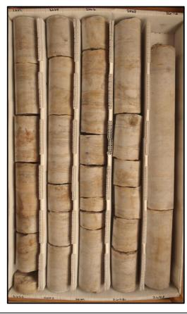
Description: 2660-2670 - Laminated to medium interbedded light brown dolomitic limestone (mudstone) and gray to white to opaque anhydrite. Granular to crystalline texture. Well indurated. Moderately fractured. Very low porosity and permeability. Fracture and intercrystalline porosity. Fracturing along bedding planes does not appear natural and may be caused by mechanical action of wireline coring.
