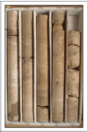
Description: 1930-1940 - Light brown to tan limestone (mudstone-wackestone), granular with light brown crystalline dolostone 1930-1930.5, massive. Well indurated, low porosity and permeability. Intergranular porosity. Voids infilled with white to opaque gypsum and anhydrite. Dark gray thinly bedded friable micrite with some organics 1931.5-1931.6, some dark gray laminations throughout. Somewhat chalky and friable 1937.65-1937.75. Pseudophragmina and bivalve fragments.
