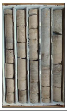
Description: 2330-2340 - 2330-2336.75 and 2338-2340 medium to thickly bedded tan to light brown limestone and dolomitic limestone (mudstone-wackestone), 2336.75-2338 thickly bedded brown crystalline dolostone. Well indurated. Granular to crystalline texture. Low permeability and porosity. Fracture and intergranular/intercrystalline porosity. White to opaque gypsum infilling fossil molds and voids. Dark brown lignite laminations 2331-2331.5 and 2338-2338.5.
