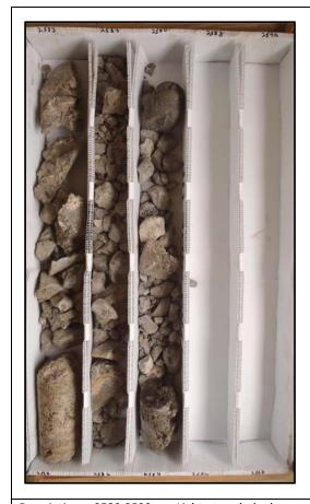
Description: 2580-2590 - Light to dark brown dolomitic limestone (mudstone-wackestone) with medium bedded green fat clay (CH) at bottom of core (most of the clay likely washed out during coring). Poorly to moderately well indurated. Very intensely fractured. Moderate to high porosity and permeability. Fracture, intergranular, some moldic porosity. Some vugs and secondary porosity developed 2580-2580.5 and 2587.5-2588.
