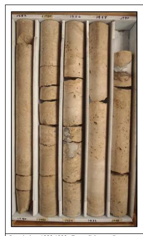
Description: 1980-1990 - Tan to light gray limestone (mudstone-wackestone) with thinly bedded white to opaque gypsum and anhydrite 1989.45-1989.50 and thinly bedded dark brown lignite 1989.4-1989.45. Granular to massive texture. Moderately well indurated, low porosity and moderately low permeability. Fracture, intergranular and moldic porosity. Voids and fossil molds infilled with gypsum and anhydrite from 1980-1985.75.
