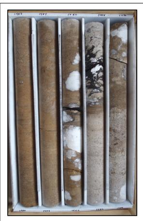
Description: 1480-1490 - Light brown to brown dolostone (mudstone to wackestone) with thinly bedded gypsum and anhydrite and anhydrite 1489.75-1490. Moderately to well indurated, low permeability. Somewhat sucrosic texture, pinpoint and moldic porosity, gypsum infilling. Fractured with laminations to thinly bedded lignite, gypsum and anhydrite infilling from 1487.25-1487.75.
