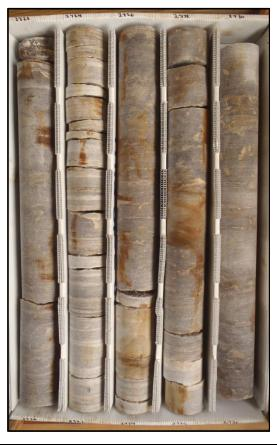
Description: 2720-2730 - Thickly bedded light brown to gray dolomitic finely crystalline anhydrite with some white laminated to thinly bedded gypsum throughout. Irregular bedded light brown dolomitic limestone (mudstone) laminations throughout. Well indurated. Granular to massive texture. Slightly to moderately fractured. Very low porosity and permeability. Fracture and intercrystalline porosity.
