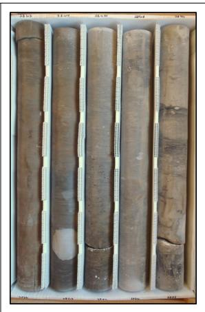
Description: 2860-2870 - Laminated to thickly bedded light to dark gray to brown dolomitic limestone (mudstone). Moderately well indurated. Slightly fractured. Fracture surfaces appear fresh and do not appear natural. Very low porosity and permeability. Some moldic and intergranular porosity. Some dark brown organic rich laminations 2863.5-2864.5 and 2867.5-2869.5. Some white to opaque nodular gypsum. Bivalve molds.
