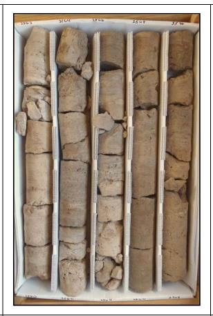
Description: 2560-2570 - Laminated to thickly bedded light brown to gray dolomitic limestone (mudstone-wackestone), more intensely dolomitized 2561-2565. Moderately well indurated. Granular texture. Moderately to very intensely fractured, fracture zone 2564-2564.5. Moderately low to moderate porosity and moderate permeability. Fracture, moldic and intergranular porosity. Some vugs and secondary porosity developed in more dolomitized sections of core 2561-2566 and 2569-2569.
