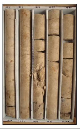
Description: 1970-1980 - Tan to light gray limestone (mudstone-wackestone), granular. Moderately well indurated, low porosity and moderately low permeability. Fracture, intergranular and some moldic porosity. Some dark gray to brown lignite laminations throughout. Some gastropod and bivalve fragments. Slightly fractured 1970-1974, moderately to intensely fractured 1974-1980. Soft and friable at 1974.5.
