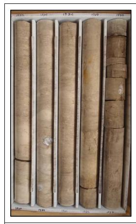
Description: 1920-1930 - Light brown to tan limestone (wackestone), granular. Well indurated, low porosity and permeability. Intergranular porosity. Voids infilled with gypsum and anhydrite. Abundant Pseudophragmina.
