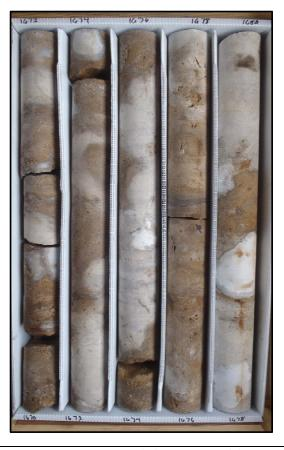
Description: 1670-1680 - Light brown to gray dolostone (crystalline) with thinly bedded white to opaque gypsum and anhydrite 1678.5-1678.7. Well indurated, low permeability. Moldic, pinpoint and intercrystalline porosity, somewhat sucrosic 1670-1676, massive 1676-1680. Some sandy seams from 1670-1674.5. Voids infilled with gypsum and anhydrite.
