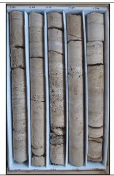
Description: 1290-1300 - Light brown dolomitic limestone (wackestone to mudstone). Moderately well to well indurated, moderately low to low permeability. Highly dolomitized with succrosic texture from 1380-1283. Moldic and intergranular porosity with some calcite and white to opaque gypsum infilling. Some horizontal laminations throughout, lignite laminations at 1294.5, 1297.5 and 1298.5.
