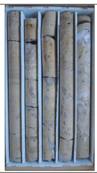
Description: 1370-1380 - Light brown dolomitic limestone (wackestone). Moderately well indurated, low permeability. Moldic, pinpoint and intergranular porosity, gypsum infilling. White to opaque gypsum seams at 1370, 1370.5 and 1373.5. Thin bedded gypsum 1379-1380. Horizontal and vertical fractures from 1373-1373.5 infilled with gypsum.
