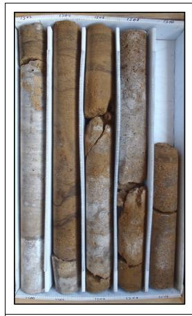
Description: 1500-1510 - Brown dolostone (wackestone-crystalline) with thinly bedded white to opaque gypsum and anhydrite from 1500-1500.5. Moderately to well indurated, low to moderately low permeability. Moldic and pinpoint porosity, vuggy with sucrosic texture from 1501.5-1510. Soft and somewhat friable from 1504-1507.5. white evaporite staining 1500.5-1501.5 and 1504-1505. Bivalve molds.
