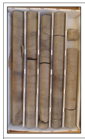
Description: 2910-2920 - Laminated to thickly bedded light to dark gray to yellow-brown limestone (mudstone-wackestone). Some dark somewhat irregular laminations throughout with some organics. Unfractured to slightly fractured. Horizontal fracture surfaces (2) appears fresh and do not appear natural. Granular texture. Moderately well to well indurated. Very low porosity and permeability. Intergranular porosity. Bivalve fragments.
