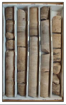
Description: 2300-2310 - Thickly bedded tan-light brown limestone (mudstone-wackestone) 2300-2301.5 and 2308.5-2310, light brown laminated-med. bedded dolomitic limestone (mudstone-wackestone) 2301.5-2303.5 2305.5-2306.75 and 2308-2308.75, thickly bedded brown crystalline dolostone 2303.5-2305.5 and 2306.75-2308. Brown lignite laminations 2301.5-2302.5, 2303.5-2306 and 2308-2308.75. Some white-opaque gypsum infilling vugs. Slightly to moderately fractured.
