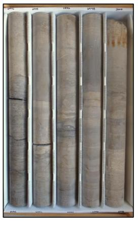
Description: 2990-3000 - Laminated to thickly bedded gray to light gray to yellow-brown limestone (mudstone-wackestone). Slightly fractured, fracture surfaces appear fresh. Granular texture. Some dark laminations with some organics throughout. Moderately well to well indurated. Low porosity and permeability. Intergranular, fracture and some moldic porosity. Some bivalve molds. Some white nodular gypsum throughout.
