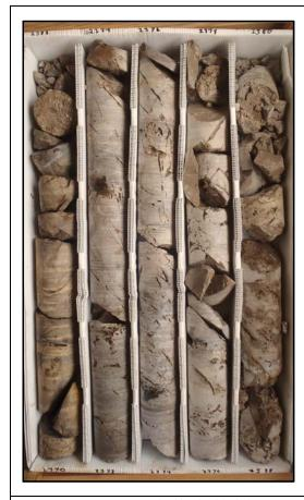
Description: 2370-2380 - Thickly bedded brown to gray crystalline dolostone. Very well indurated. Massive texture. Moderately fractured, fracture zones 2377-2380 (dolostone somewhat brecciated, healed with gypsum), abundant fractures at oblique angles to drill string. Some white to opaque gypsum infilling oblique fractures. Moderate porosity and low to moderate permeability. Fracture, moldic and intercrystalline porosity. Lignite lamination 2370.25.
