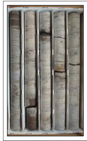
Description: 2340-2350 - Medium to thickly bedded brown to gray crystalline dolostone. Very well indurated. Crystalline texture. Very low porosity and permeability. Fracture and some moldic and pinpoint porosity. White to opaque gypsum and anhydrite infilling horizontal and vertical fractures and some fossil molds. Dark brown thinly bedded lignite 2345.75 and lignite lamination at 2347. Some iron staining 2340-2347.
