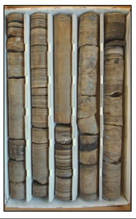
Description: 2780-2790 - Laminated to thickly bedded light-dark gray to yellow-brown dolomitic limestone (mudstone). Mod. well to well indurated. Moderately to intensely fractured. Granular texture. White-light blue-opaque nodular gypsum/anhydrite throughout infilling primary/secondary porosity, thinly bedded gypsum 2781.3, 2783.75, 2784.1, 2784.5. Some dark brown lignite laminations throughout. Low porosity and perm. Fracture, intergranular and some moldic porosity.
