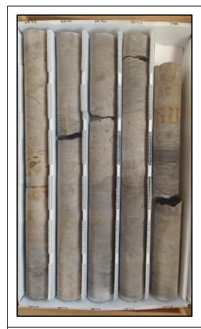
Description: 2970-2980 - Laminated to thickly bedded gray to light gray to yellow-brown limestone (mudstone-wackestone). Slightly to moderately fractured, fracture surfaces appear fresh. Some dark laminations with some organics throughout. Granular texture. Moderately well to well indurated. Low porosity and permeability. Intergranular, fracture and some moldic porosity. Some bivalve molds. Some white nodular gypsum throughout.
