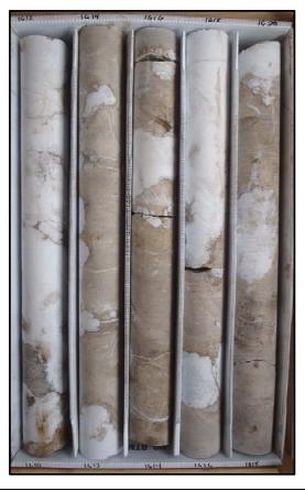
Description: 1610-1620 - Brown to gray dolostone (crystalline) with thinly bedded white to opaque gypsum and anhydrite at 1613.25, medium bedded from 1615.25-1615.6 and 1616.25-1616.6, thickly bedded from 1610.25-1612 and 1617-1618.75. Well indurated, very low permeability. Intercrystalline porosity. Some voids and some horizontal and vertical fracturing, infilled with gypsum and anhydrite.
