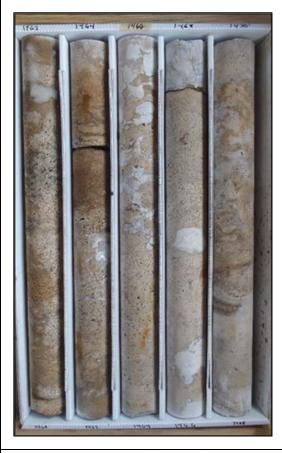
Description: 1460-1470 - Light brown to brown dolostone (mudstone to wackestone) with medium bedded white to opaque gypsum and anhydrite from 1461.9-1462.05 and 1467.8-1468.15 (fractured with micritic infilling). Well indurated, low permeability. Moldic, vuggy, pinpoint and intergranular porosity, gypsum infilling. White evaporite staining.
