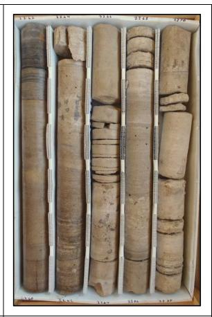
Description: 2260-2270 - Brown thickly bedded dolostone (crystalline) 2260-2262, tan to brown thinly bedded dolomitic limestone (wackestone) 2262-2263, tan to light brown to light gray thinly-medium bedded limestone (wackestone) 2263-2270. Slightly to intensely fractured, limestone soft, granular and somewhat chalky and friable. Moldic, intergranular/intercrystalline and fracture porosity, moderately low porosity and permeability. Some moldic porosity infilled with gypsum and anhydrite.
