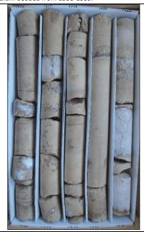
Description: 1350-1360 - Light brown dolomitic limestone (mudstone). Moderately well indurated, low permeability. Moldic, intergranular and pinpoint porosity, gypsum infilling. Thin bedded white to opaque gypsum at 1351 and 1353.5, medium bedded from 1358-1359.5 and thin bedded at 1357.5.
