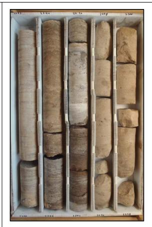
Description: 2290-2300 - Thickly bedded brown crystalline dolostone 2290-2292.5 and 2294-2295.75, thickly bedded light brown dolomitic limestone (wackestone) 2292.5-2294, thickly bedded light brown limestone (mudstone) 2295.75-2300. Moderately fractured. Moderately well to well indurated. Moderately low porosity and permeability. Fracture, intergranular and intercrystalline porosity, some vugs. Granular to crystalline texture. Some gypsum infilling of vugs 2294-2295.75.
