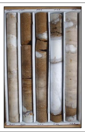
Description: 1720-1730 - Light brown to brown dolostone (wackestone-crystalline) with thickly bedded white to opaque gypsum and anhydrite from 1726.15-1728.2, medium bedded 1722-1722.3, thinly bedded 1720.85-1721 and 1721.1-1721.6. Well indurated, low to moderately low permeability. Massive to sucrosic texture from 1722.5-1728.5. Some shell 1722.5-1728.5. Bivalves. Void infilling gypsum and anhydrite.
