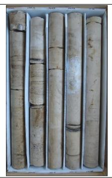
Description: 1400-1410 - Light brown dolomitic limestone (1400-1403.5 mudstone, 1403.5-1410 wackestone). Moderately well indurated, low permeability. Moldic, pinpoint and intergranular porosity, gypsum infilling. Medium bedded gypsum at 1407. Lignite laminations at 1403 and thinly bedded lignite at 1406.5.
