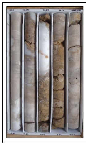
Description: 1620-1630 - Light brown to brown dolostone (crystalline) with medium bedded white to opaque gypsum and anhydrite 1620-1620.5 and 1625-1625.8. Well indurated. Moldic and intercrystalline porosity, massive 1620-1623.5 and 1628-1630, low perm. Moldic and pinpoint porosity with sucrosic texture from 1623.5-1627.75, moderate perm., moderately to intensely fractured. Horizontal and vertical fracturing, gypsum infilling.
