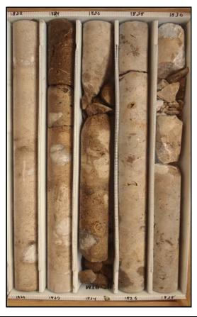
Description: 1820-1830 - Light brown to brown to gray dolostone (wackestone crystalline -). Poorly to well indurated, very low to moderate (fracture) permeability. Very intensely fractured 1824-1824.4, 1825.4-1825.8 and 1829.5-1829.8. Somewhat sandy and friable with trace amounts of lignite 1823.5-1824.4. Moldic, intercrystalline and fracture porosity. Some iron staining 1823-1825.8. Gypsum and anhydrite void infilling. Some shell, bivalves.
