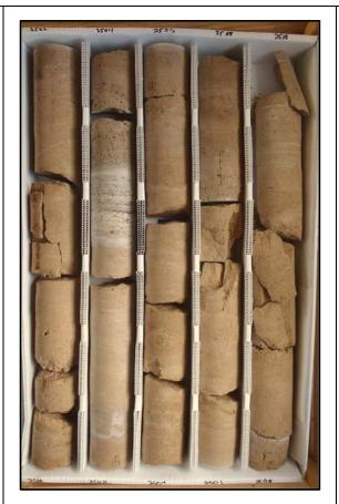
Description: 2500-2510 - Thickly bedded light brown dolomitic limestone (wackestone), gray and more intensely dolomitized 2503-2504. Moderately well indurated. Granular texture. Moderately fractured. Low porosity and moderately low permeability. Fracture and intercrystalline/intergranular porosity.
