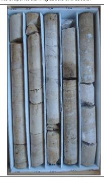
Description: 1380-1390 - Light brown dolomitic limestone (wackestone). Moderately well indurated, low permeability. Moldic, pinpoint and intergranular porosity, gypsum infilling. White evaporite staining 1384-1388. Horizontal fractures with white to opaque gypsum infilling at 1381.5, 1385-1386 and 1388-1390. Gypsum seam at 1385. Lignite lamination at 1286.
