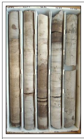
Description: 2280-2290 - Tan to brown medium bedded dolomitic limestone (wackestone) 2280-2281.5, brown to gray thickly bedded crystalline dolostone 2281.5-2290. Slightly fractured. Some moldic, intergranular and intercrystalline porosity. Very low porosity and permeability. Some iron staining 2284.25-2285.15 and 2287.5-2287.85. White-opaque gypsum infilling some of the fossil molds. Some organic-rich laminations.
