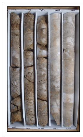
Description: 1650-1660 - Light brown to brown dolostone (crystalline) with thinly bedded white to opaque gypsum and anhydrite 1655-1655.2 and 1658-1658.25. Well indurated. Sucrosic texture with sandy seams, pinpoint and intercrystalline poros. 1650-1655, low to moderately low perm. Massive 1655-1670, intercrystalline and moldic poros., very low perm. Horizontal and vertical fracturing and voids completely infilled with gypsum and anhydrite.
