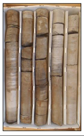
Description: 2810-2820 - Laminated-thickly bedded light brown-gray dolomitic limestone (mudstone-wackestone) 2810-2810.3 and 2811.5-2816.75, laminated-med. bedded dolomitic gypsum and anhydrite 2810.3-2811.5 and 2816.75-2820. Granular to massive texture. Mod. well-well indurated. Slightly-mod. fractured. Low poros. and perm. Fracture, intergranular/intercrystalline and some moldic poros. Some anhydrite infilling vugs/molds 2814-2816.75.
