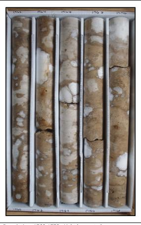
Description: 1760-1770 - Light brown to brown dolostone (wackestone-crystalline). Moderately to well indurated, low permeability. Moldic and intergranular/intercrystalline porosity, massive texture. Some shell 1762.75-1770, bivalves. Voids infilled with gypsum and anhydrite.
