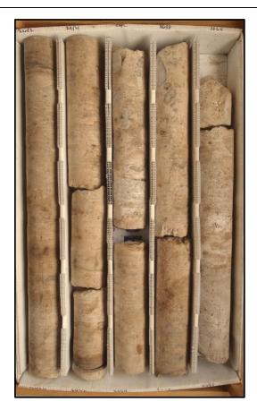
Description: 2650-2660 - Tan to light brown laminated to thickly bedded dolomitic limestone (mudstone-wackestone). Some dark brown lignite laminations 2650.75-2653. Granular texture. Moderately well to well indurated. Low porosity and permeability. Fracture, moldic and intergranular porosity. Some gray to white gypsum and anhydrite infilling primary/secondary porosity 2655-2660.
