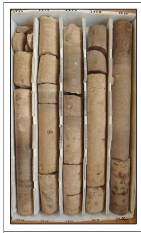
Description: 2250-2260 - Tan to light brown limestone (wackestone), light brown dolomitic limestone from 2250-2251, 2255-2256 and 2257.5-2260. Poorly to well indurated, granular texture. Limestone is somewhat chalky. Slightly to very intensely fractured (fracture zone 2255.5-2255.75). Moldic, intergranular and fracture porosity. Moderately low porosity and permeability. Some white-opaque gypsum and dark gray anhydrite infilling some fossil molds.
