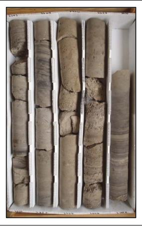
Description: 2600-2610 - Gray-light brown thickly bedded limestone (mudstone-wackestone) 2600-2602, 2602.75-2606 and 2607.75-2610, Gray-light brown med. to thickly bedded dolomitic limestone (mudstone-wackestone) 2602-2602.75 and 2606-2607.75. Mod. well indurated. Mod. fractured. Mod. low poros. and mod. low to mod. perm. Fracture, intergranular and some moldic porosity. Some vugs and secondary porosity developed 2602-2602.5 and 2604.75-2607.75.
