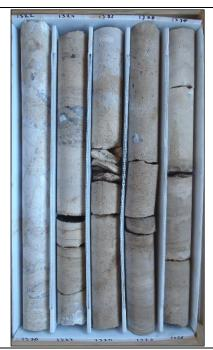
Description: 1320-1330 - Light brown dolomitic limestone (1320-1323 mudstone, 1323-1330 wackestone). Highly fractured (vertical and horizontal) with gypsum infilling 1320-1322.25. Moderately well indurated, low permeability. Pinpoint and moldic porosity, some vugs, gypsum infilling. Horizontal and vertical fractures infilled with gypsum from 1321.25-1330.
