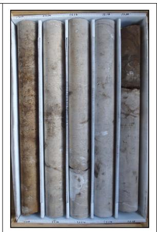
Description: 1510-1520 - Brown to gray dolostone (wackestone-crystalline) with medium bedded white to opaque gypsum and anhydrite from 1514.25-1514.5. Moderately to well indurated, low to moderately low permeability. Moldic and pinpoint porosity, vuggy with sucrosic texture 1520-1524.5, some gypsum infilling. Lignite laminations from 1519-1520. Some horizontal fracturing with gypsum infilling from 1512-1519. Bivalve molds.
