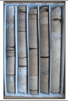
Description: 1310-1320 - Light brown dolomitic limestone (mudstone) with opaque-white mediumthick bedded white to opaque gypsum from 1310.2-1310.4, 1311.4-1312.5, 1318.75-1318.95 and 1319.5-1320. Moderately well indurated, low permeability. Intergranular and moldic porosity, infilled with gypsum.
