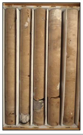
Description: 1850-1860 - Light brown to brown dolostone (crystalline) with thinly bedded white to blue anhydrite and brown chert 1852-1852.25 and thinly bedded white to opaque gypsum and anhydrite 1854.3-1854.5. Well indurated, very low permeability, low porosity. Intercrystalline porosity, little moldic porosity. Voids infilled with gypsum and anhydrite. Slightly fractured. Some horizontal laminations throughout.
