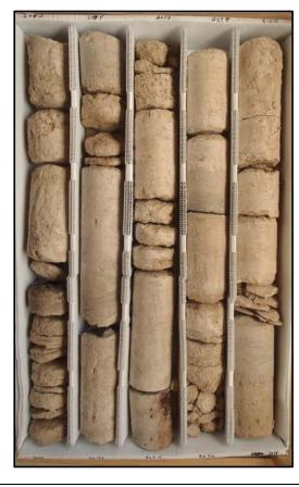
Description: 2070-2080 - Light brown to gray dolomitic limestone (wackestone) 2070-2072 and 2075-2078.75, granular, tan to light brown limestone (mudstone-wackestone) 2072-2075 and 2078.75-2080, granular, soft and somewhat chalky. Mod. well to well indurated, mod. low to mod. perm. and poros. Moldic, fracture and intergranular poros. Some graygreen clay 2070-2072 (glauconitic).
