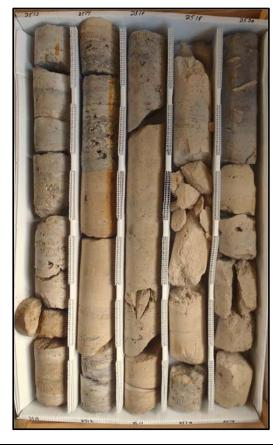
Description: 2510-2520 - Medium to thickly interbedded light brown dolomitic limestone and light gray dolostone (wackestone-crystalline). Moderately well indurated. Granular-crystalline texture. Moderately fractured. Low porosity and moderately low to moderate permeability. Fracture and intercrystalline/intergranular porosity. Some secondary porosity developed throughout. Dark brown lignite lamination 2514.5.
