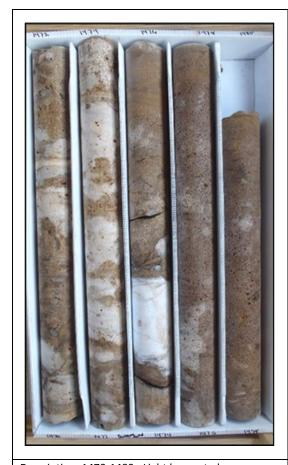
Description: 1470-1480 - Light brown to brown dolostone (mudstone to wackestone) with medium bedded white to opaque gypsum and anhydrite from 1474.4-1474.8 (massive). Well indurated, low permeability. Moldic, vuggy, pinpoint and intergranular porosity, gypsum infilling. Lignite laminations from 1474-1476.
