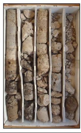
Description: 2570-2580 - Med. to thickly bedded light brown-gray dolomitic limestone (mudstone-wackestone), intensely dolomitized and light-dark gray-brown 2570.5-2573.75. Mod. well indurated. Granular-crystalline texture. Mod. to very intensely fractured, fracture zone 2572.5-2573.5, 2573.7-2574, 2574.5-2576 and 2578.5-2580. Mod. to high porosity and perm. Fracture, Moldic and intergranular porosity. Some vugs and secondary porosity developed throughout.
