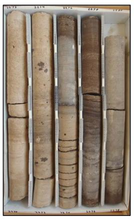
Description: 2270-2280 - Tan to thinly to thickly bedded light brown limestone (wackestone) 2270-2275.25, Drown dolostone (crystalline) 2275.25-2280. Slightly to intensely fractured at 2274-2275. Moldic, intergranular/crystalline, and fracture porosity. Low porosity and permeability. White to opaque gypsum infilling some fossil molds. Limestone has granular somewhat chalky texture.
