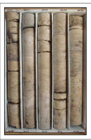
Description: 2020-2030 - Tan to light gray limestone (mudstone-wackestone) with brown to gray dolostone from 2026.5-2029.5. Granular-chalky and massive texture. Moderately well to well indurated, low to moderately low permeability and porosity. Moldic, fracture and intergranular porosity. Somewhat soft and chalky 2023.75-2024.75 and 2025.5-2026.5. Some dark laminations 2026.75-2030. Reworked 2028.9-2029.3. Dark gray, clayey with some organics 2021-2022.
