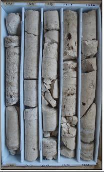
Description: 1210-1220 - Light brown dolomitic limestone (wackestone). Moderately well indurated, low permeability. Moldic and pinpoint porosity with some calcite infilling.
