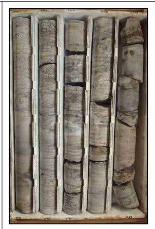
Description: 2350-2360 - Medium to thickly bedded light to dark brown to gray crystalline dolostone. Slightly to moderately fractured and very well indurated. Crystalline, massive texture. Low porosity and permeability. Fracture, moldic (somewhat vuggy) and intercrystalline porosity. Vertical and horizontal fractures throughout infilled with white to opaque gypsum (some selenite).
