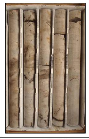
Description: 2430-2440 - Thickly bedded light brown crystalline dolostone. Very well indurated. Massive texture. Slightly to mod. fractured. Mod. low porosity and moderate permeability. Fracture, moldic and intercrystalline porosity. Some apparent secondary porosity developed 2439-2440 (losing circulation). Some iron staining 2439-2440. White to opaque gypsum and anhydrite (nodular to medium bedded fracture infilling) 2430-2430.5, 2438-2439.
