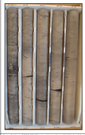
Description: 2930-2940 - Laminated to thickly bedded light to dark gray to yellow-brown limestone (mudstone-wackestone). Some dark somewhat irregular laminations with some organics 2930-2932 and 2934.5. Unfractured to slightly fractured. Fracture surfaces appear fresh and do not appear natural. Granular texture. Moderately well to well indurated. Very low porosity and permeability. Intergranular porosity. Bivalve fragments.
