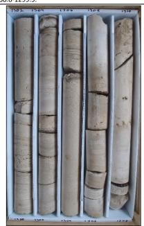
Description: 1300-1310 - Light brown dolomitic limestone (wackestone 1300-1302, mudstone 1302-1310). Moderately well to well indurated, low permeability. Intergranular and moldic porosity 1300-1302. Vertical fractures from 1302.5-1302.8, 1303.1-1303.75 and 1306.3-1307.5. Voids/fractures partially or completely infilled with white to opaque gypsum.
