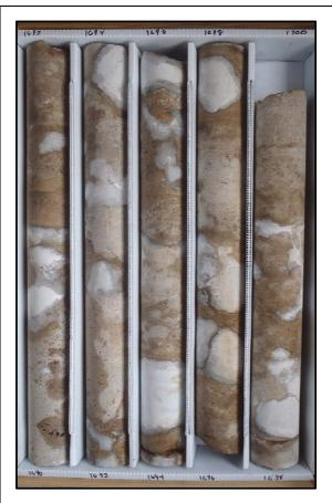
Description: 1690-1700 - Light brown to brown dolostone with thinly bedded white to opaque gypsum and anhydrite 1680.25-1680.5, medium bedded 1689.4-1689.9. Well indurated, low permeability. Moldic and intercrystalline porosity, massive. Horizontal and vertical fractures 1694.5-1695.25, gypsum and anhydrite infilled. Voids infilled with gypsum and anhydrite.
