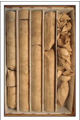
Description: 1900-1910 - Light brown to tan limestone (mudstone-wackestone), granular. Poorly to well indurated, low to moderately low permeability and porosity. Intergranular and fracture porosity. Moderately fractured 1900-1900.5, slightly fractured 1901-1907, very intensely fractured 1900.5-1901 and 1907-1910. Voids infilled with white to opaque gypsum and anhydrite. Apparent natural break and somewhat chalky and friable at 1900.75. Bivalve fragments. Core is very dry.
