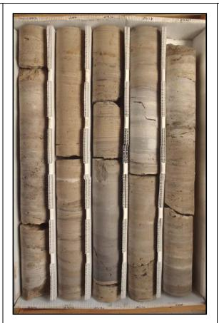
Description: 2410-2420 - Medium to thickly interbedded light brown to gray dolostone and dolomitic limestone (wackestone-crystalline). Well indurated. Granular to massive texture. Slightly to moderately fractured. Some gray laminations 2412-2413. Some gray clay lenses 2415-2417. Low porosity and permeability. Fracture, moldic and intergranular/ intercrystalline porosity.
