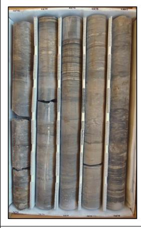
Description: 2870-2880 - Laminated to medium bedded light to dark gray to brown limestone (mudstone). Slightly fractured. Fracture surfaces appear fresh and do not appear natural. Moderately well indurated. Some dark brown lignite laminations and organic rich banding throughout. Very low porosity and permeability. Intergranular porosity.
