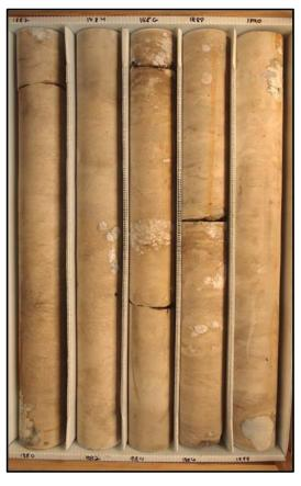
Description: 1880-1890 - 1880-1888.75 Light brown dolostone (crystalline), massive, 1888.75-1890 light brown to tan limestone (mudstone-wackestone), granular. Well indurated, very low permeability and porosity. Moldic and intergranular and intercrystalline porosity. Voids infilled with white to opaque gypsum and anhydrite. Apparent natural breaks at sandy/clayey seams at 1885.9 and 1887.2. Some bivalve molds.
