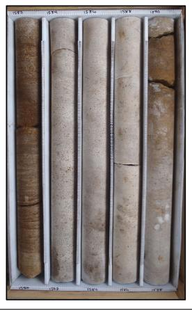
Description: 1580-1590 - Brown dolostone (crystalline). Well indurated, low permeability. Moldic and pinpoint porosity, somewhat vuggy with sucrosic texture from 1580-1582 and 1589-1590. Some gypsum infilling. Some iron staining from 1580-1582 1589-1590. Some shell and bivalves.
