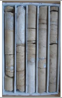
Description: 1410-1420 - Light brown dolomitic limestone (mudstone). Moderately well indurated, low permeability. Moldic, pinpoint and intergranular porosity, gypsum infilling. Medium bedded white to opaque gypsum at 1411.5 and thick bedded gypsum from 1413-1414.5. Lignite laminations at 1417.5 and 1419.5.
