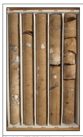
Description: 1830-1840 - Light brown to brown dolostone (crystalline). Thinly bedded (0.02') lignite at 1833.6. Well indurated, low permeability. Intercrystalline porosity, little moldic porosity. Voids infilled with gypsum and anhydrite. Slightly to moderately (1838.75-1840) fractured.
