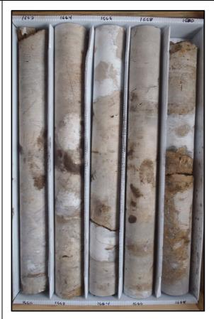
Description: 1660-1670 - Light brown to gray dolostone (crystalline) with medium bedded white to opaque gypsum and anhydrite 1665.5-1666.1 and 1669.1-1669.5. Well indurated, low permeability. Moldic, pinpoint and intercrystalline porosity, massive, but somewhat sucrosic 1661.9-1662.1, 1664.25-1664.9, 1668.25-1669.75. Horizontal and vertical fracturing 1660-1663, gypsum and anhydrite infilled. Voids infilled with gypsum and anhydrite.
