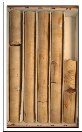
Description: 1890-1900 - Light brown to tan limestone (mudstone-wackestone), granular. Well indurated, low permeability and porosity. Voids infilled with white to opaque gypsum and anhydrite. Intergranular porosity. Pseudophragmina and bivalve fragments.
