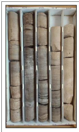
Description: 2310-2320 - Thickly bedded tan-light brown limestone (wackestone) 2310-2311 and 2317-2320, thinly to med. bedded tan-light brown dolomitic limestone (wackestone) 2311-2312.25 and 2314-2317 and brown crystalline dolostone 2312.25-2314. Mod. well to well indurated. Granular to crystalline texture. Mod. low porosity and permeability. Fracture, moldic, intergranular/intercrystalline and some pinpoint porosity.
