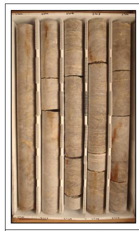
Description: 2700-2710 - Thickly bedded light brown to gray dolomitic finely crystalline anhydrite with some white gypsum laminations throughout. Irregular bedded light brown dolomitic limestone (mudstone) laminations throughout. Well indurated. Granular to massive texture. Slightly to moderately fractured. Very low porosity and permeability. Fracture and intercrystalline porosity.
