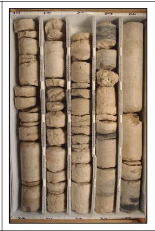
Description: 2110-2120 - Tan to light brown limestone (wackestone-packstone) with some thinly to medium bedded gray chert at 2117.5. Granular texture, poorly to moderately well indurated, somewhat friable. Intergranular and fracture porosity, moderately low permeability and porosity. Moderately to intensely fractured. Some lignite at 2110 and some green clay (glauconite) at 2110 and 2118.
