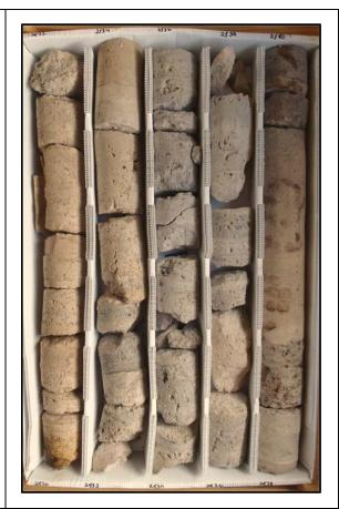
Description: 2530-2540 - Medium to thickly bedded light brown to gray dolomitic limestone (mudstone-wackestone). Poorly to mod. well indurated, soft 2531-2533 and 2534-2538. Granular texture. Mod. to intensely fractured with some fracturing along bedding planes. Mod. low porosity and moderately low to moderate permeability. Fracture, moldic and intergranular porosity. Some vugs and secondary porosity developed 2530-2538.5. Dark brown lignite laminations at 2532.4 and 2533.75.
