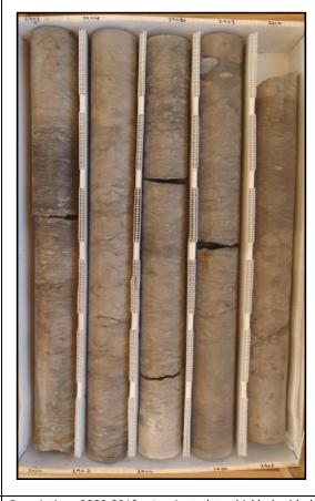
Description: 2880-2890 - Laminated to medium bedded light to dark gray to yellow-brown limestone (mudstone-wackestone). Unfractured to slightly fractured. Fracture surfaces appear fresh and do not appear natural. Moderately well to well indurated. Some dark organic laminations throughout. Some white to opaque nodular/void infilling gypsum 2876-2879. Very low porosity and permeability. Intergranular porosity. Bivalve fragments.
