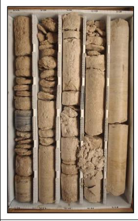
Description: 2120-2130 - Tan to light brown limestone (wackestone-packstone) with some gray to dark gray medium bedded gray chert at 2120.5. Poorly indurated, granular texture, friable. Low permeability and porosity, fracture and intergranular permeability. Moderately to very intensely fractured. Irregular dark pressure solution (stylolite) surfaces at 2021 and 2024.75.
