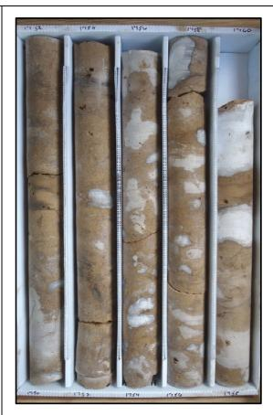
Description: 1750-1760 - Light brown to brown dolostone (wackestone-crystalline) with medium bedded white to opaque gypsum and anhydrite 1758.8-1759.1 and 1759.25-1759.65. Moderately to well indurated, low perm. Moldic and pinpoint poros., massive to somewhat sucrosic texture. Some shell 1750-1754, bivalves. Sandy seams at 1751.25, 1753.7, 1754.1, 1757.7, friable at 1751.25. Some calcite crystals with euhedral habit in fossil molds. Voids infilled with gypsum and anhydrite.
