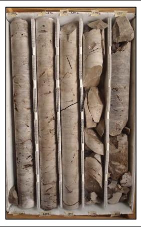
Description: 2390-2400 - Thickly bedded brown to gray crystalline dolostone. Very well indurated. Massive texture. Slightly fractured 2390-2396, moderately fractured 2396-2400, fracture zone 2399.5-2400, some fracturing at oblique angles to drill string. Moderately low porosity and moderately low permeability. Fracture, moldic and intercrystalline porosity.
