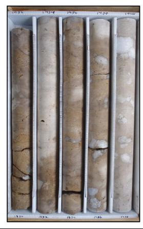
Description: 1730-1740 - Light brown to brown to gray dolostone (crystalline) with thin beds of white to opaque gypsum and anhydrite 1732.3-1732.7. Modwell indurated, low to mod. low perm. Moldic and pinpoint poros. Sandy seams and sucrosic texture 1732-1736 and 1738.5-1740, mod. to intense fracturing, somewhat friable. Some shell 1731.5-1740. Bivalves. Some calcite crystals with euhedral crystal habit in fossil molds. Voids infilled with gypsum and anhydrite
