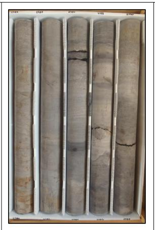
Description: 2980-2990 - Laminated-thickly bedded gray to light gray to yellow-brown limestone (mudstone-wackestone). Slightly fractured, fracture surfaces appear fresh. Granular texture. Mod. well to well indurated. Some dark laminations with some organics throughout. Low porosity and permeability. Intergranular, fracture and some moldic porosity. Some bivalve molds. Some white nodular gypsum throughout.
