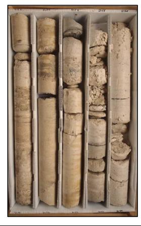
Description: 2130-2140 - Tan to light brown limestone (wackestone). Poorly to moderately well indurated, granular texture, friable. Moderately low permeability and porosity, fracture and intergranular permeability. Moderately to very intensely fractured. Apparent fracturing along bedding planes. Gypsum void and fossil mold infilling at 2133.5 and 2136-2138. Some green clay (glauconite) 2136-2138. Bivalve molds.
