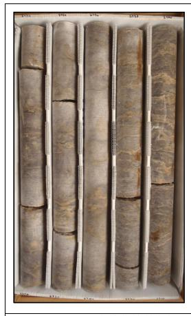
Description: 2730-2740 - Thickly bedded light brown to gray dolomitic finely crystalline anhydrite. Irregular bedded light brown dolomitic limestone (mudstone) laminations throughout. Well indurated. Granular to massive texture. Slightly to moderately fractured. Very low porosity and permeability. Fracture and intercrystalline porosity.
