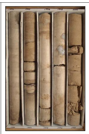
Description: 1990-2000 - Brown to Tan to light gray limestone (mudstone), granular-chalky to massive. Mod. well indurated, low porosity and low to mod. low perm. Fracture and intergranular poros. Some organics, brown 1990-1992.6, dark brown lignite laminations 1992.6-1992.9. Voids infilled with white to opaque gypsum and anhydrite. Friable and chalky 1994-1998.2. Very intensely fractured zones and somewhat friable 1998.2-1998.4 and 1999.8-2000. Some bivalve fragments.
