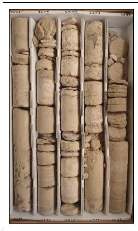
Description: 2220-2230 - Tan to light brown limestone (wackestone), some light brown to gray dolomitic limestone 2220-2222. Poorly to moderately well indurated, granular texture, somewhat chalky and friable. Fracture, intergranular, moldic porosity, moderate porosity and permeability. White-opaque gypsum (some selenite) and dark gray anhydrite infilling some fossil molds throughout.
