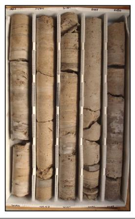
Description: 2480-2490 - 2480-2481.75 Thickly bedded light brown-gray crystalline dolostone, 2481.75-2490 thinly to thickly bedded light brown-gray dolomitic limestone (wackestone). Mod. well to very well indurated. Massive-granular texture. Mod. fractured, intensely fractured along bedding planes 2485-2487. Mod. low porosity and moderate perm. Fracture, moldic and intercrystalline/ intergranular porosity. Some apparent secondary porosity developed throughout.
