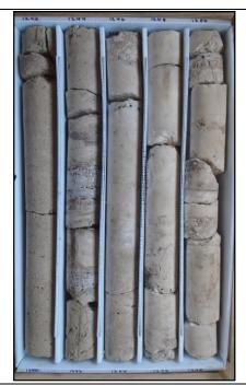
Description: 1240-1250 - Light brown dolomitic limestone (1240-1246 mudstone, 1246-1250 wackestone). Poorly to moderately well indurated, low permeability. Moldic and intergranular porosity with some calcite infilling. Evaporite staining gypsum 1240-1242.
