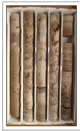
Description: 2490-2500 - 2490-2491.5 Light brown dolomitic limestone (wackestone), 2491.5-2500 laminated to thickly interbedded light brown to gray dolomitic limestone and crystalline dolostone. Mod. well to well indurated. Massive-granular texture. Slightly fractured. Mod. low poro. and mod. low to mod. perm. Fracture, moldic and intercrystalline/intergranular porosity. Some apparent secondary porosity developed 2495-2499.
