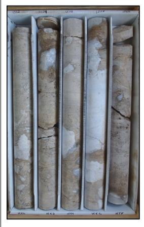
Description: 1550-1560 - Light brown to brown dolomitic limestone (crystalline) with thick bedded opaque to white gypsum and anhydrite from 1556-1557.25. Well indurated, low permeability. Moldic porosity, some voids, gypsum infilling.
