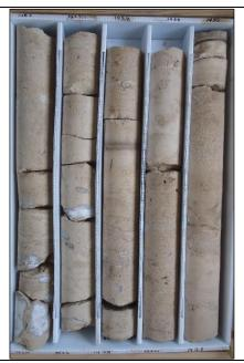
Description: 1420-1430 - Light brown dolomitic limestone (1420-1425.5 and 1427-1430 mudstone, 1425.5-1427 wackestone). Moderately well indurated, low permeability. Moldic, pinpoint and intergranular porosity, gypsum infilling. Lignite laminations at 1429.75. Some horizontal laminations
