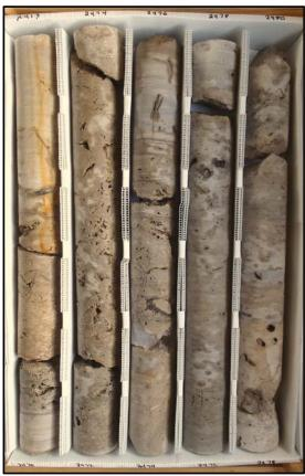
Description: 2470-2480 - Thickly bedded light brown to gray crystalline dolostone, 2470.5-2471.5 thickly bedded light brown dolomitic limestone (mudstone). Very well indurated. Massive-granular texture. Slightly to moderately fractured. Moderately low porosity and moderate permeability. Fracture, moldic and intercrystalline porosity. Some apparent secondary porosity developed throughout. Opaque gypsum fracture infilling 2464.5. Dark brown lignite lamination 2466.
