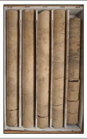
Description: 1940-1950 - Light brown to tan limestone (mudstone-wackestone), granular. Moderately well indurated, low porosity and moderately low permeability. Fracture, intergranular and little moldic porosity. Voids infilled with white to opaque calcite, fossil molds partially infilled. Some dark gray laminations with some organics throughout, abundant laminations 1949-1950. Pseudophragmina and bivalve fragments.
