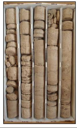
Description: 2240-2250 - Gray to tan to light brown limestone (mudstone-wackestone). Poorly to moderately well indurated, granular texture, somewhat friable and chalky. Fracture, intergranular, moldic porosity. Moderate porosity and permeability. White-opaque gypsum and dark gray anhydrite infilling some fossil molds 2249-2250.
