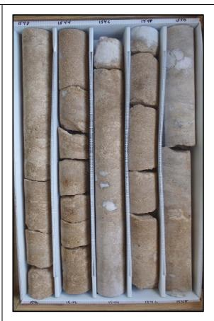
Description: 1540-1547.75 - Light brown to brown dolomitic limestone (wackestone), medium bedded white to opaque gypsum and anhydrite 1547.75-1548, brown to gray dolostone 1548-1550 (crystalline). Moderately to well indurated, low permeability. Pinpoint porosity with some vugs in more highly dolomitized areas. Horizontal fractures 1548.5-1550 with gypsum infilling. Friable at 1546. Some shell, bivalves and gastropods 1540-1547.75.
