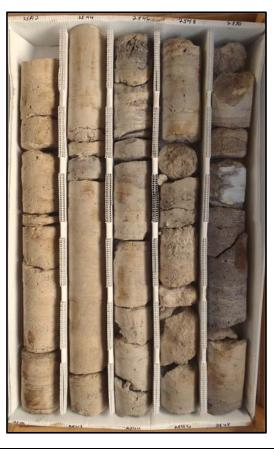
Description: 2540-2550 - Thickly bedded light brown to gray dolomitic limestone (mudstone-wackestone), gray med. bedded dolostone 2548.5-2549.25 and med. bedded white to opaque gypsum and anhydrite 2549.2-2549.4. Poorly to mod. well indurated. Granular to crystalline texture. Mod. to intensely fractured, fracture zone at 2546. Mod. low poros. and perm. Fracture, moldic and intergranular porosity. Some secondary porosity developed 2545-2549.
