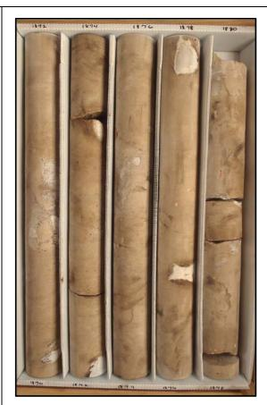
Description: 1870-1880 - Light brown dolostone (crystalline), massive. Well indurated, very low permeability and porosity. Intercrystalline porosity, little moldic porosity. Voids infilled with gypsum and anhydrite. Sandy/clayey laminations and apparent natural breaks at 1872.5, 1873.5, 1874, 1878.1, 1878.9, 1879.15.
