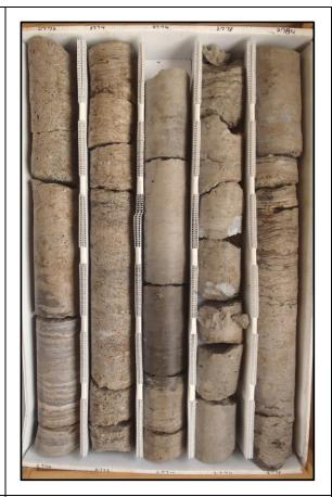
Description: 2770-2780 - 2770-2770.7 thickly bedded light brown-gray dolomitic finely crystalline anhydrite w/ some irregular bedded light brown dolomitic limestone (mudstone) laminations and thinly bedded-laminated white gypsum, 2770.7-2780 light brown-gray laminated-thickly bedded dolomitic limestone (mudstone-wackestone). Mod. well-well indurated. mod. fractured. Fracture, moldic, intergranular and some pinpoint poros. White nodular gypsum 2770.7-2774.5 and 2776.5-2779.5.
