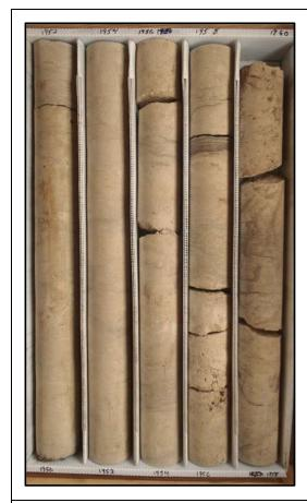
Description: 1950-1960 - Tan to light gray limestone (mudstone-wackestone), granular. Moderately well indurated, low porosity and moderately low permeability. Fracture, intergranular and little moldic porosity. Fossil molds partially infilled with calcite. Dark gray to brown thinly bedded friable micrite with some organics 1957.5-1957.6, some dark gray to brown laminations with some organics throughout. Pseudophragmina and bivalve fragments.
