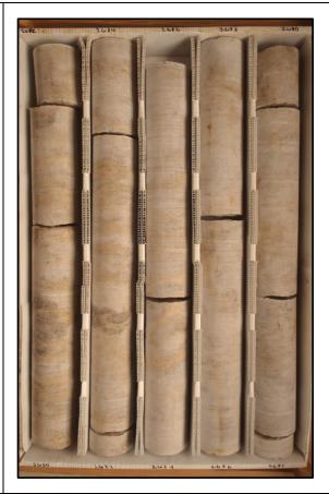
Description: 2680-2690 - Laminated to medium interbedded light brown dolomitic limestone (mudstone) and gray to white to light brown to opaque anhydrite. Granular to massive texture. Well indurated. Slightly to moderately fractured. Very low porosity and permeability. Fracture intergranular and intercrystalline porosity. Dolomitic limestone bedding is irregular and appears to have infilled fractures/voids in anhydrite.
