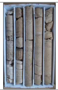
Description: 1230-1230.5 and 1236.5-1237.5 – light brown dolostone (mudstone). 1230.5-1236.5 and 1237.5-1240 – light brown dolomitic limestone (wackestone). Moderately well indurated, low permeability. Moldic and intergranular porosity with some calcite infilling.
