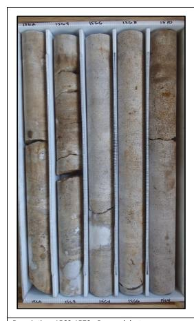
Description: 1560-1570 - Brown dolostone (crystalline) with medium bedded gypsum and anhydrite from 1561.9-1562.2 and 1564.25-1564.5. Well indurated, low permeability. Moldic and pinpoint porosity, somewhat vuggy from 1566.5-1570, partial gypsum infilling. Vertical fractures approximately 1 millimeter from 1564-1566.5, horizontal fracturing 1560-1563.5, gypsum infilling. Iron staining 1569-1570.
