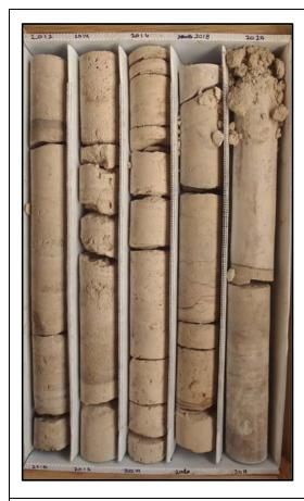
Description: 2010-2020 - Tan to light gray limestone (mudstone-wackestone), granular texture. Poorly to moderately well indurated, low to moderately low permeability and porosity. Moldic, intergranular and fracture porosity. Some blue to gray anhydrite 2016.5-2018.5. Clayey and intensely fractured 2019.5-2020. Dark lignite laminations 2010.25, 2011.4, 2012.15, 2016, 2016.5-2017 and 2018.
