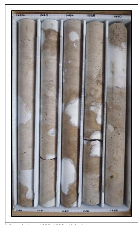
Description: 1680-1690 - Light brown to gray dolostone (crystalline) with thinly bedded white to opaque gypsum and anhydrite 1690.85-1690.95, 1695.8-1696 and 1696.7-1696.9, medium bedded 1694.1-1694.5. Well indurated, low permeability. Moldic and intercrystalline porosity, massive. Horizontal and vertical fractures 1682.75-1683.75, gypsum and anhydrite infilled. Voids infilled with gypsum and anhydrite.
