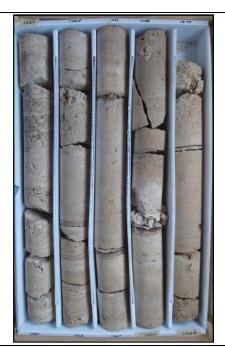
Description: 1260-1264.25 and 1265.75-1270 – light brown dolomitic limestone (wackestone). 1264.25-1265.75 – light brown dolostone. Moderately well to well indurated, moderately low horizontal permeability with solution channels (<0.5 centimeters) at 1267. Massive to moldic porosity with some vugs from 1260-1264.25. Some calcite infilling.
