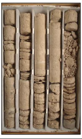
Description: 2210-2220 - Tan to light brown limestone (wackestone). Poorly-moderately well indurated, granular texture, somewhat chalky and friable. Moderate permeability and porosity. Intergranular, fracture and some moldic porosity. Moderately to very intensely fractured. Some fossil molds infilled with white to opaque gypsum 2210-2211, 2215.75-2216.5 and 2217.5-2218.5. Some gray thinly to medium bedded dolomitic limestone 2216-2216.5 and 2217.25-2217.5
