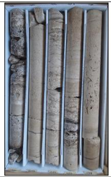
Description: 1250-1251 - brown dolostone (crystalline), massive with few vugs. 1251-1260 – light brown dolomitic limestone, highly dolomitized from 1251-1252 and 1256.25-1256.75. Moderately to well indurated, low permeability. Moldic and intergranular/intercrystalline porosity. Void infilling gypsum at 1255.5.
