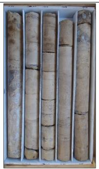
Description: 1360-1370 - Light brown dolomitic limestone (1360-1366 mudstone, 1366-1370 wackestone). Moderately well indurated, low permeability. Moldic, pinpoint and intergranular porosity, gypsum infilling. Gypsum seams from 1363-1366.5 and 1368.75, medium bedded 1369.5-1370. White evaporite staining 1366.5 and 1368.5.
