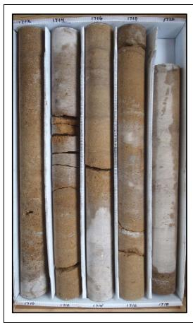
Description: 1710-1720 - Light brown to brown dolostone. Well indurated, low to moderate permeability. Moldic and pinpoint porosity, massive to sucrosic (1710.5-1713, 1714.75-1717 and 1717.35 to 1718.35) texture. Vertical fracture from 1714.4-1714.9, gypsum infilled. Slightly fractured, intensely fractured from 1713-1713.4. Some gypsum and anhydrite void infilling. Some sandy seams.
