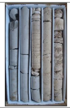
Description: 1200-1204.5 – Grout. 1204.5-1210 – light brown dolomitic Limestone (wackestone). Moderately well indurated, low permeability. Pinpoint and moldic porosity with some calcite infilling.
