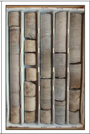
Description: 2320-2330 - Tan-light brown dolomitic limestone (wackestone) 2320-2321.75, 2323-2325, 2328-2328.5, tan-light brown limestone (wackestone) 2321.75-2323, brown crystalline dolostone 2325-2328 and 2328.5-2340. Granular to crystalline texture. Slightly to moderately fractured. Well indurated. Low porosity and permeability. Fracture, intergranular/intercrystalline and some moldic porosity. Some white to opaque gypsum infilling fossil molds and voids.
