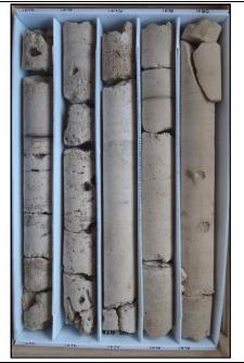
Description: 1270-1280 - Light brown dolomitic limestone (wackestone). Moderately well indurated with moderate horizontal permeability. Moldic and intergranular porosity with solution channels (<1 centimeter) from 1271-1273. Some calcite infilling of solution channels and molds (euhedral crystals).
