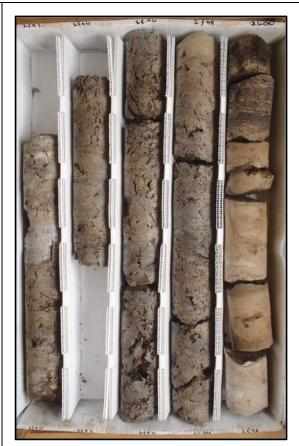
Description: 2590-2600 - 2590-2596.5 Thickly bedded light to dark brown to gray crystalline dolostone, 2596.5-2600 medium bedded light brown limestone (mudstone). Moderately well to well indurated. Moderately fractured. Granular to crystalline texture. Moderate to high porosity and permeability. Fracture, some moldic and intergranular/intercrystalline porosity. Abundant vugs and secondary porosity developed 2590-2596.5.
