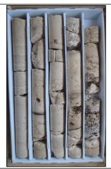
Description: 1220-1228.5 and 1229.25-1230– light brown dolomitic limestone (wackestone). 1228.5-1229.25 – drown dolostone (crystalline), vuggy. Moderately well to well indurated, low to moderate permeability. Moldic and intergranular porosity with some calcite infilling.
