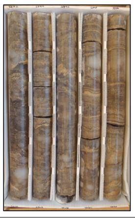
Description: 2840-2850 - Laminated to medium bedded light brown to light to dark gray dolomitic anhydrite and gypsum. Very well indurated. Very low porosity and permeability. Intercrystalline porosity. Fracture surfaces appear fresh and do not appear natural.
