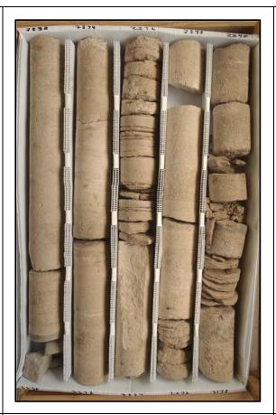
Description: 2230-2240 - Tan to light brown limestone (mudstone-wackestone). Moderately well indurated, granular texture, somewhat friable and poorly indurated 2234.6-2236.3 and 2238-2240. Fracture, intergranular, moldic porosity, moderately low porosity and permeability. White-opaque gypsum infilling some fossil molds 2234-2240.
