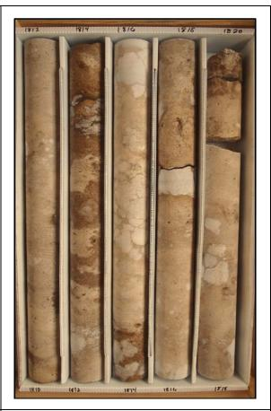
Description: 1810-1820 - Light brown to brown dolostone (wackestone-crystalline with fractured medium bedded white to opaque gypsum and anhydrite 1814.75-1815.3, thinly bedded 1812.15-1812.35, 1813.5-1813.7, 1815.75-1815.85, 1815.95-1816.1, 1817.1-1817.3. Well indurated, low permeability and porosity. Moldic and intercrystalline porosity. Massive. Some shell, bivalves. Voids infilled with gypsum and anhydrite. Some horizontal fracturing (< 2 millimeters) 1819-1820, gypsum and anhydrite infilled.
