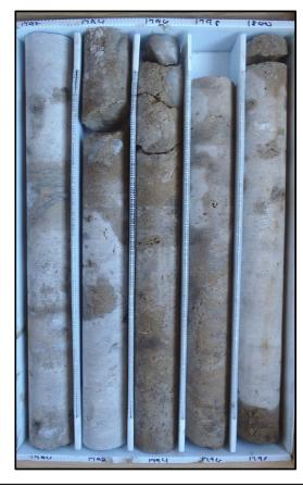
Description: 1790-1800 - Light brown to brown dolostone (wackestone-crystalline). Well indurated, low permeability and porosity. Massive to somewhat sucrosic from 1793.25-1796.4 and 1799.5-1800. Moldic and intercrystalline porosity. Some shell, bivalves. Voids infilled with gypsum and anhydrite. Some laminations at 1791.25. Sandy seams and apparent natural breaks at 1793.5 and 1796.2.
