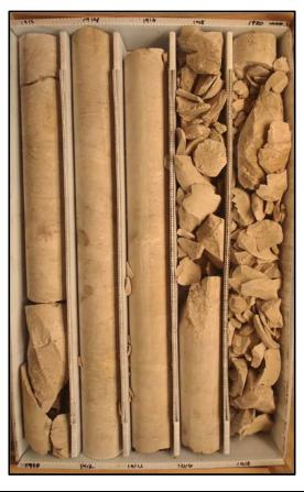
Description: 1910-1920 - Light brown to tan limestone (mudstone-wackestone), granular. Poorly to well indurated, low to moderately low permeability and porosity. Intergranular and fracture porosity. Slightly fractured 1910-1915 and 1919-1920, very intensely fractured 1915-1919. Pseudophragmina and bivalves. Core is very dry.
