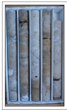
Description: 1770-1780 - Light brown to brown dolostone (wackestone-crystalline) with thinly bedded white to opaque gypsum and anhydrite from 1771.2-1771.4. Well indurated, low permeability. Some moldic and intercrystalline porosity. Sandy seams and apparent natural break at 1773.75. Some shell 1770.5-1774.5 and 1776.5-1778, bivalves. Voids infilled with gypsum and anhydrite.
