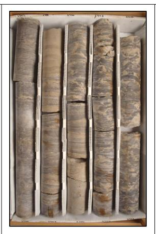
Description: 2740-2750 - Thickly bedded light brown to gray dolomitic finely crystalline anhydrite with some white gypsum laminations throughout. Irregular bedded light brown dolomitic limestone (mudstone) laminations throughout. Well indurated. Granular to massive texture. Slightly to moderately fractured. Very low porosity and permeability. Fracture and intercrystalline porosity.
