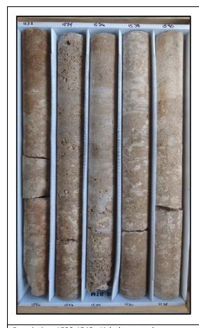
Description: 1530-1540 - Light brown to brown dolomitic limestone (wackestone). Moderately well indurated, low to moderately low permeability. Friable from 1539.75-1540. Moldic and pinpoint porosity with some vugs in more highly dolomitized areas from 1532-1535. Some laminations, shell and bivalves.
