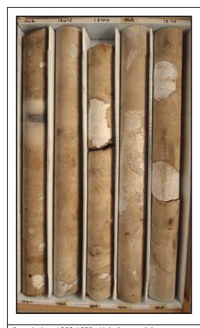
Description: 1860-1870 - Light brown dolostone (crystalline), massive. Some brown chert at 1861.3. Lignite lamination at 1862, sandy seams at 1865.25 and 1866. Well indurated, very low permeability, low porosity. Intercrystalline porosity, little moldic porosity. Voids infilled with gypsum and anhydrite. Some horizontal laminations throughout. Apparent natural breaks at 1862, 1865.25 and 1866.
