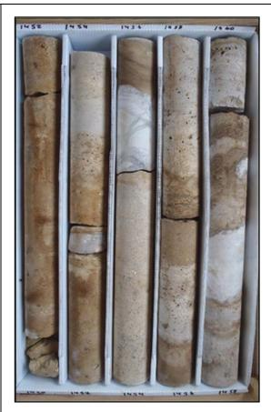
Description: 1450-1453.5- Light brown dolomitic limestone (mudstone to wackestone), 1453.5-1460 light brown to brown dolostone (mudstone to wackestone), thinly bedded white to opaque gypsum and anhydrite 1452.5-1452.6 and med. bedded gypsum and anhydrite 1454.9-1455.5 & 1458.2-1458.6. Mod. to well indurated, low perm. Moldic, vuggy, pinpoint & intergranular porosity, gypsum infill.
