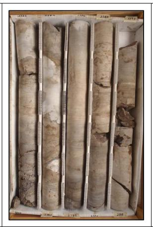
Description: 2380-2390 - Thickly bedded brown to gray crystalline dolostone, medium bedded white to opaque gypsum and anhydrite 2381-2382 and 2383-2384, nodule at 2382.5. Very well indurated. Massive texture. Slightly to moderately fractured, fracture zones 2380-2381 and 2389-2389.3, some fracturing at oblique angles to drill string. Some white to opaque gypsum infilling oblique fractures. Low porosity and moderately low permeability. Fracture, moldic and intercrystalline porosity.
