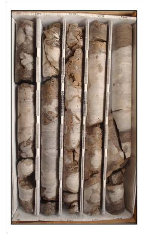
Description: 2400-2410 - Thickly bedded brown to gray crystalline dolostone. Very well indurated. Massive texture. Slightly to moderately fractured, fracture zone 2400-2401, some fracturing at oblique angles to drill string. Some white to opaque gypsum infilling fractures. Lignite laminations 2400-2402. Moderate porosity and permeability. Fracture, moldic and intercrystalline porosity. Some iron staining along fractures throughout.
