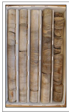
Description: 2820-2830 - Laminated-medium bedded light brown to light to dark gray dolomitic anhydrite. Slightly fractured, intensely fractured 2829-2830. Irregular bedded light brown dolomitic limestone throughout. Granular to massive texture. Well indurated. Slightly to intensely fractured. Very low porosity and permeability. Intergranular and intercrystalline porosity. Very little secondary porosity appears to be developed between 2828-2828.5.
