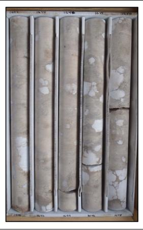
Description: 1640-1650 - Light brown to brown dolostone (crystalline) with thinly bedded white to opaque gypsum and anhydrite from 1648.1-1648.3. Well indurated, low permeability. Intercrystalline porosity. Horizontal and vertical fracturing and voids completely infilled with gypsum and anhydrite.
