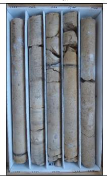
Description: 1390-1400 - Light brown dolomitic limestone (wackestone). Moderately well indurated, low permeability. Moldic, pinpoint and intergranular porosity, gypsum infilling. Horizontal and vertical fracturing with gypsum infilling at 1381.5 and 1391.7. Medium bedded white to opaque gypsum at 1399. Lignite laminations at 1390.2, 1395 and 1397.
