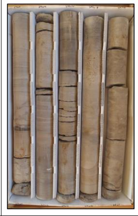
Description: 2940-2950 -Thickly bedded light gray to gray to yellow-brown limestone (mudstone-wackestone), med. bedded w/ some organics 2946.25. Some dark somewhat irregular laminations with some organics throughout. Slightly fractured to v. intensely fractured, fracture zones 2944.5-2945.25 and 2947.5-2950. Fracture surfaces appear fresh. Mod. well indurated. Low to mod. poros. and perm. Intergranular, fracture and some moldic poros.
