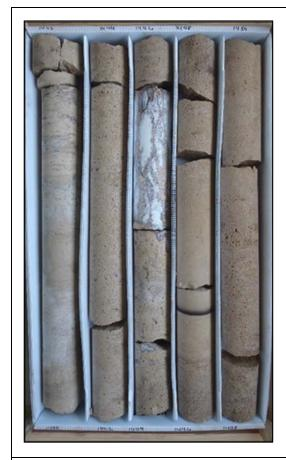
Description: 1440-1450 - Light brown dolomitic limestone (mudstone to wackestone) with medium bedded white to opaque gypsum and anhydrite (0.8' bed) at 1445 (fractured with micritic infilling). Moderately well indurated, low permeability. Moldic, pinpoint and intergranular porosity, gypsum infilling. Lignite laminations at 1446.5. Bivalve molds.
