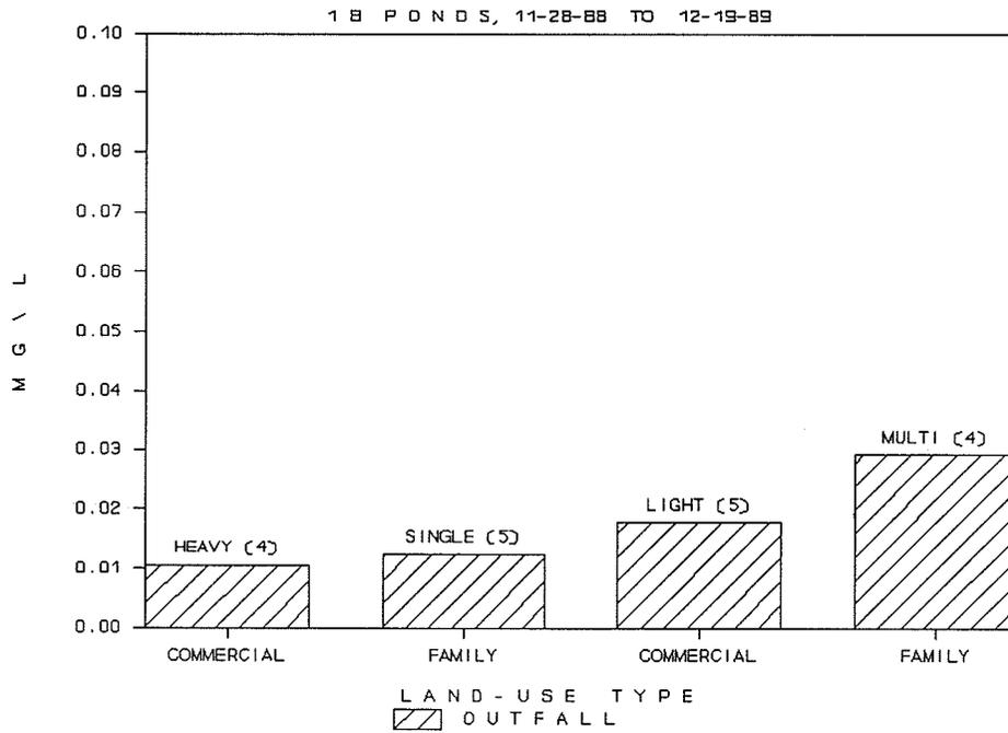
**Figure 37. Mean Outfall Copper by Four Land-Use Types. Number of ponds in parenthesis.**
