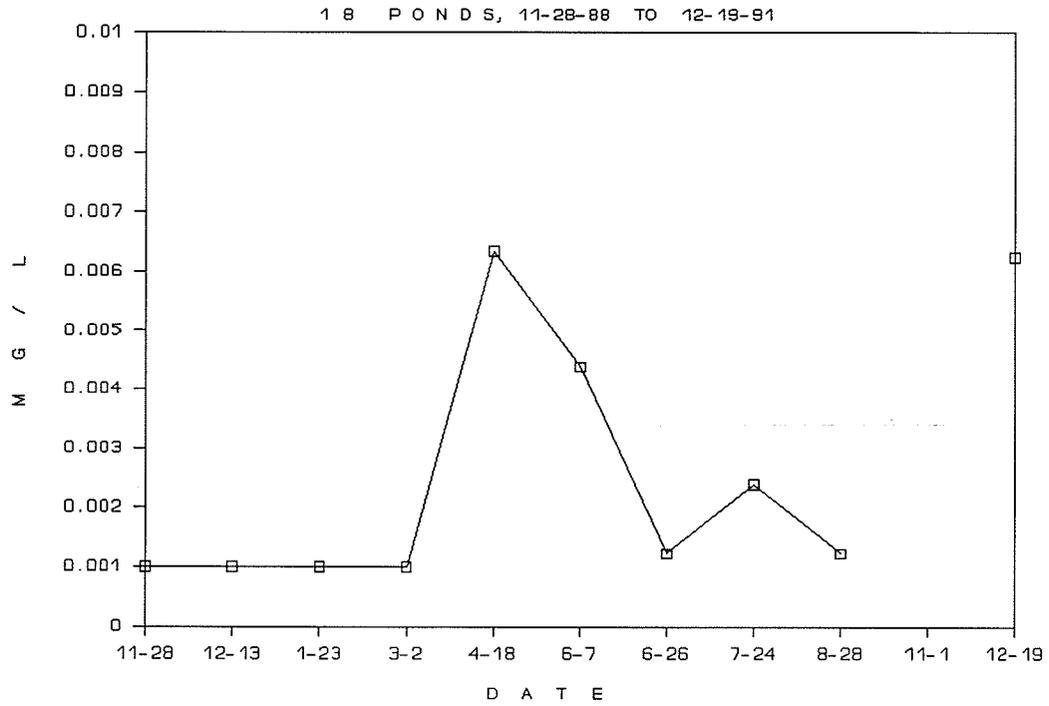
**Figure 30. Mean Cadmium Versus Date for 18 Ponds [Class III = 0.0012 mg/L].**
