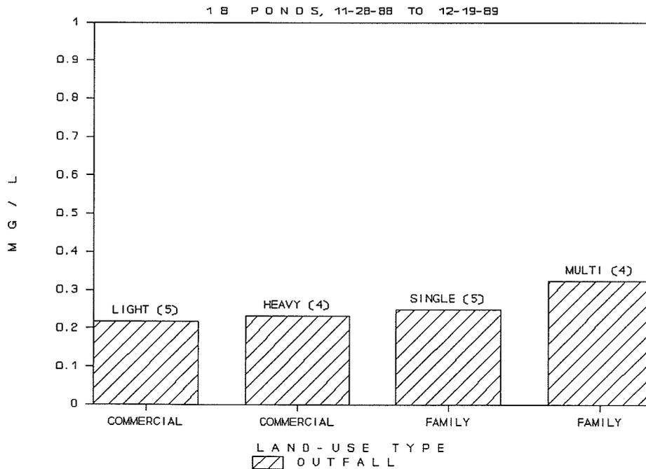
**Figure 36. Mean Outfall Iron by Four Land-Use Types. Number of ponds in parenthesis.**
