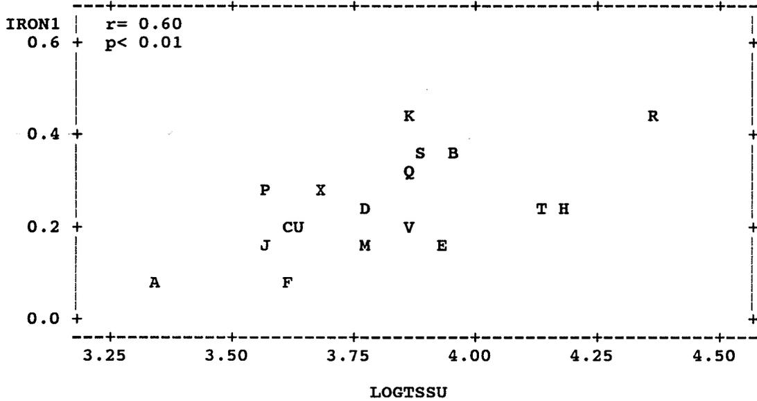
MEAN TOTAL IRON (MG/L) VS. LOG MEAN TURBIDITY (N.T.U.)
