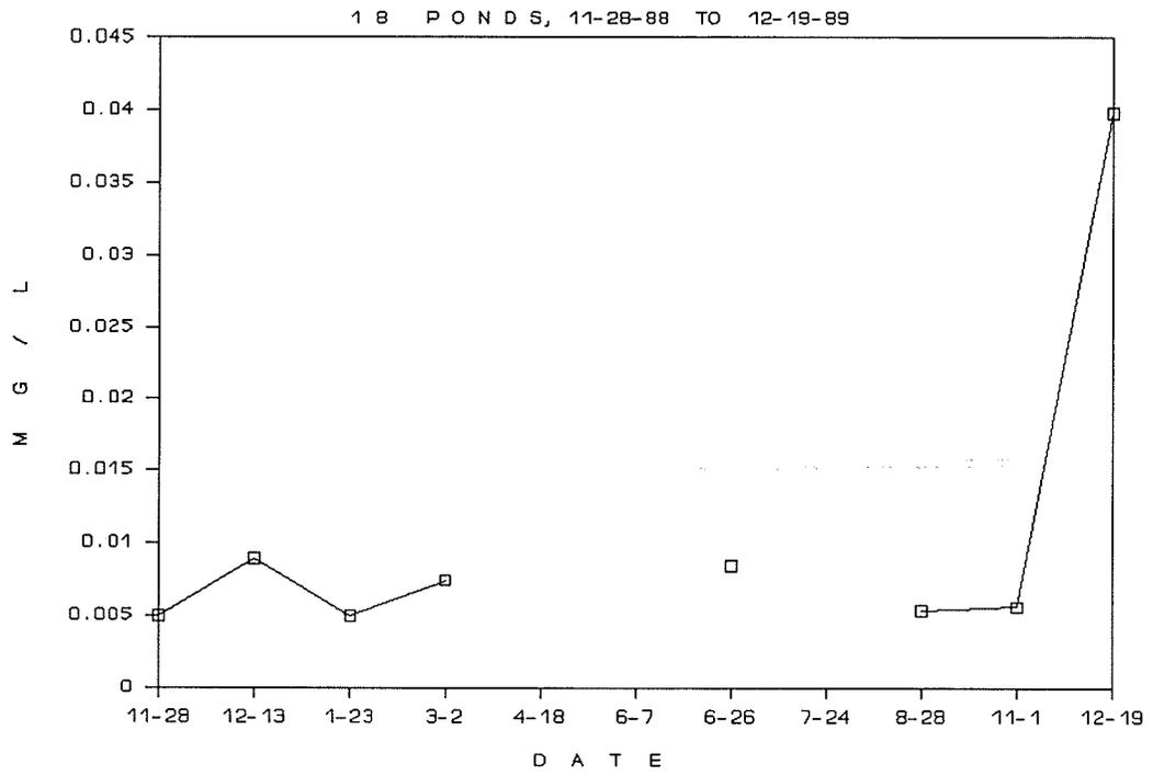
**Figure 32. Mean Nickel Versus Date for 18 Ponds [Class III = 0.10 mg/L].**
