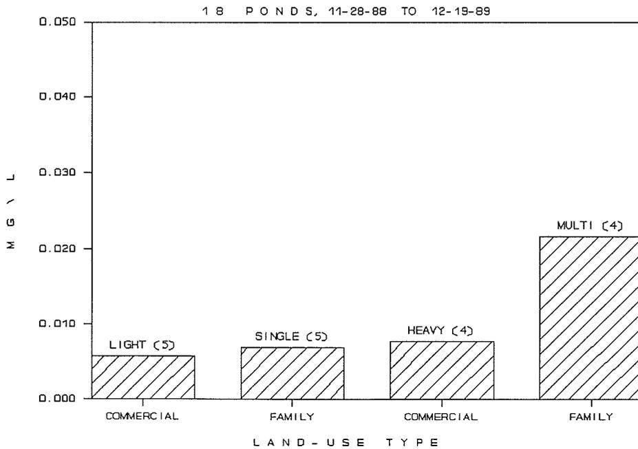
**Figure 42. Mean Nickel by Four Land-Use Types. Number of ponds in parenthesis.**
