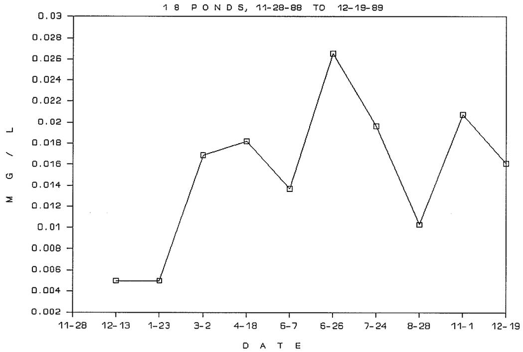
**Figure 28. Mean Manganese Versus Date for 18 Ponds [Class II = 0.10 mg/L – No Class III Standard].**
