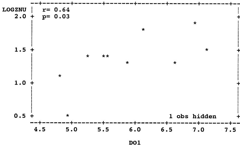
LOG MEAN TOTAL COPPER (UG/L) VS. MEAN PH
