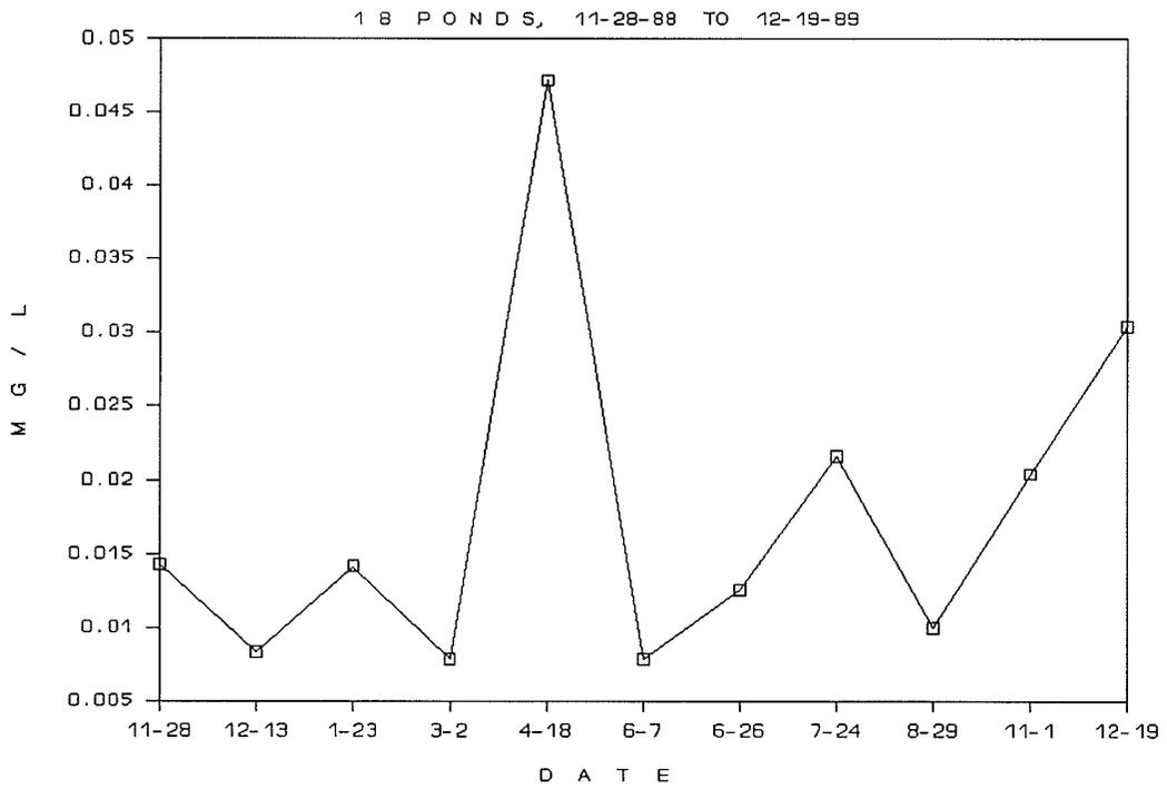
**Figure 27. Mean Copper Versus Date for 18 Ponds [Class III = 0.03 mg/L].**
