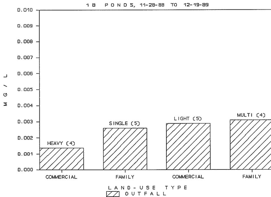
**Figure 40. Mean Outfall Cadmium by Four Land-Uses. Number of ponds in parenthesis.**
