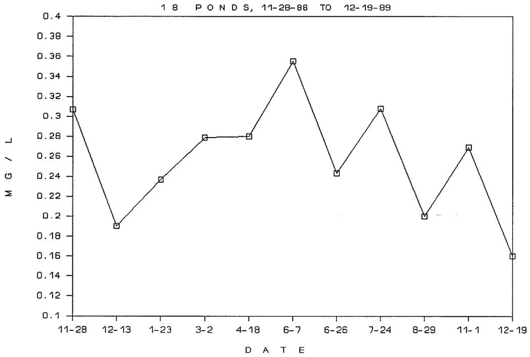
**Figure 26. Mean Iron Versus Date for 18 Ponds [Class III = 1.0 mg/L].**
