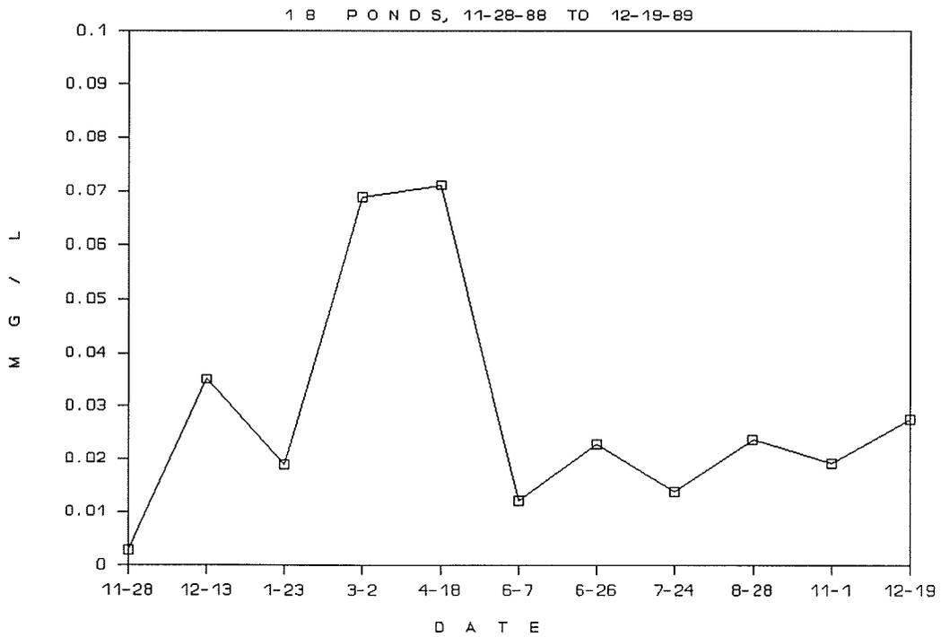
**Figure 25. Mean Zinc Versus Date for 18 Ponds [Class III = 0.03 mg/L].**
