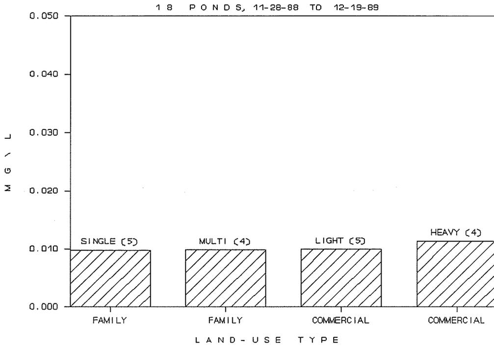
**Figure 41. Mean Outfall Chromium by Four Land-Uses. Number of ponds in parenthesis.**
