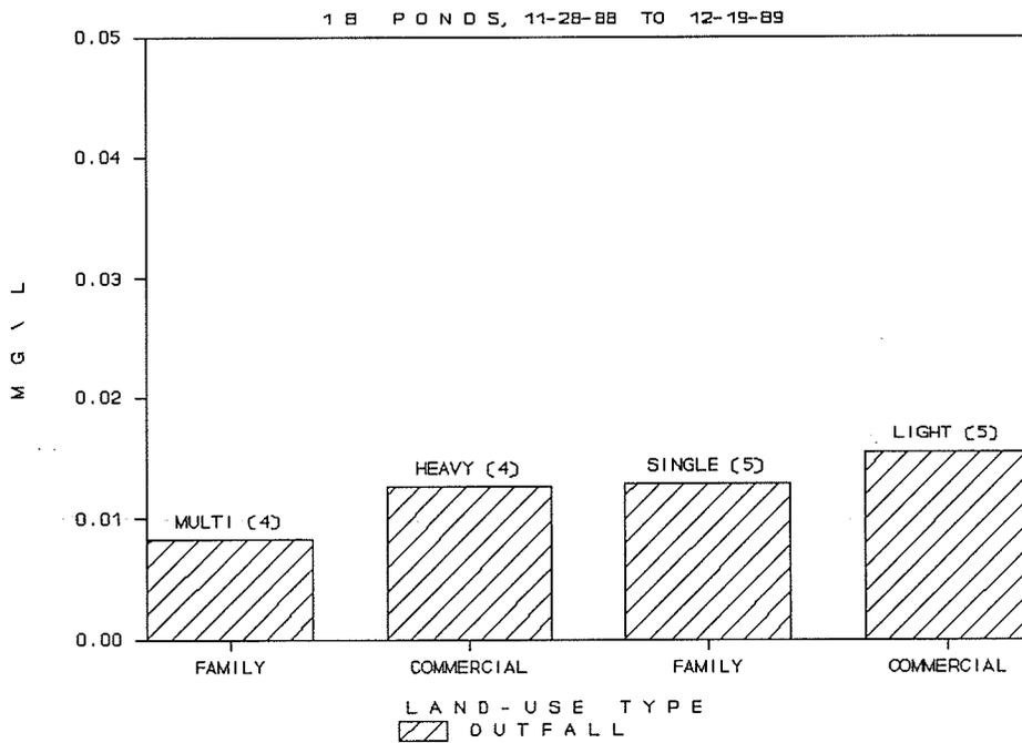
**Figure 39. Mean Outfall Lead by Four Land-Use Types. Number of ponds in parenthesis.**
