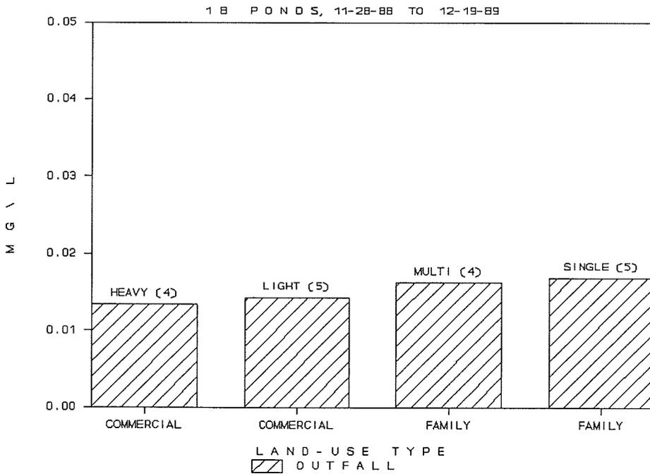
**Figure 38. Mean Outfall Manganese by Four Land-Use Types. Number of ponds in parenthesis.**
