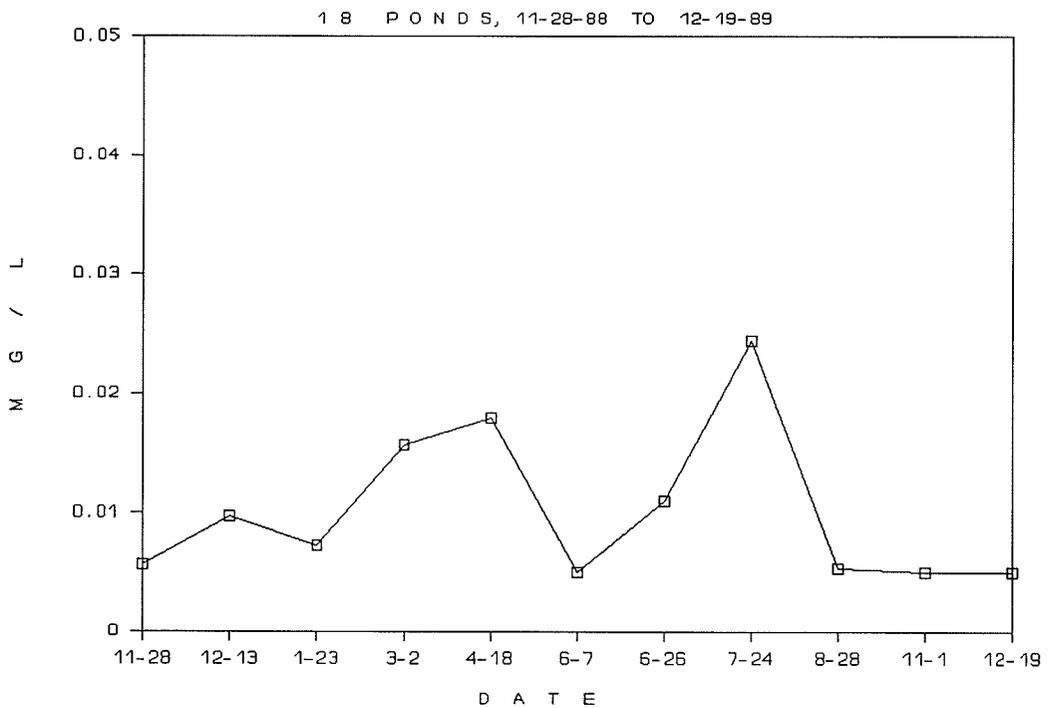
**Figure 31. Mean Chromium Versus Date for 18 Ponds [Class III = 0.05 mg/L].**
