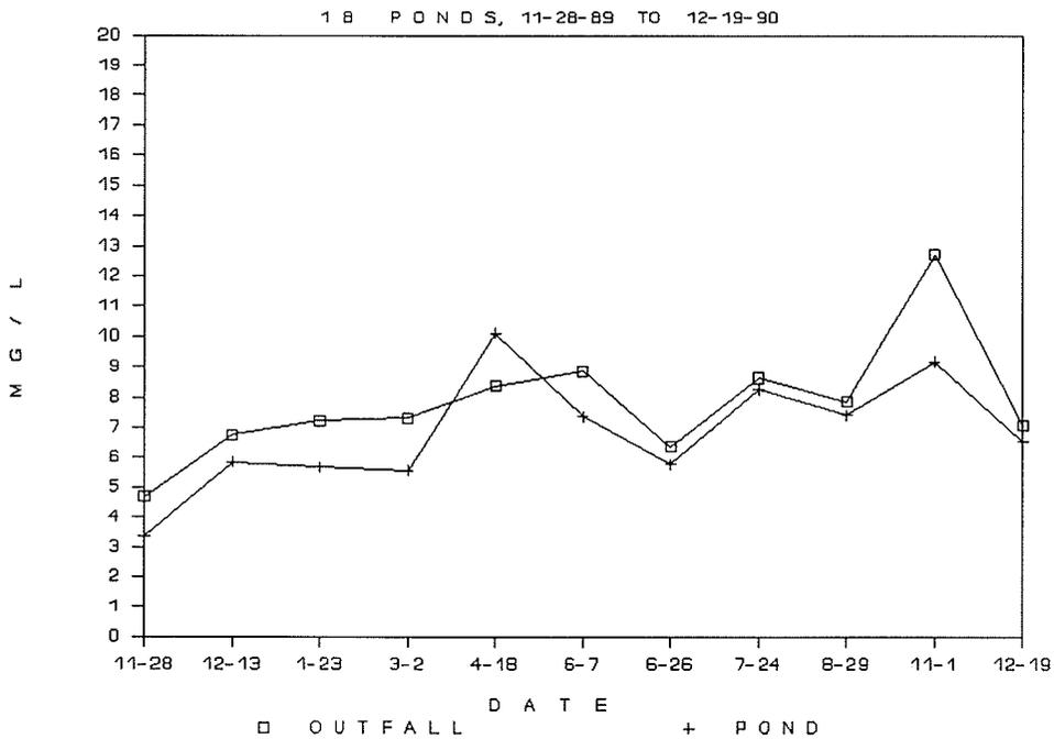
**Figure 23. Mean Total Suspended Solids Versus Date for 18 Ponds (2 Stations) [Secondary STP Effluent = 20.0 mg/L].**
