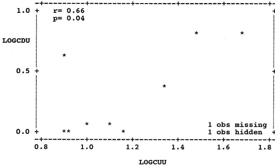
LOG MEAN TOTAL CADMIUM (UG/L) VS. LOG MEAN CONDUCTIVITY (UMHOS/CM)
