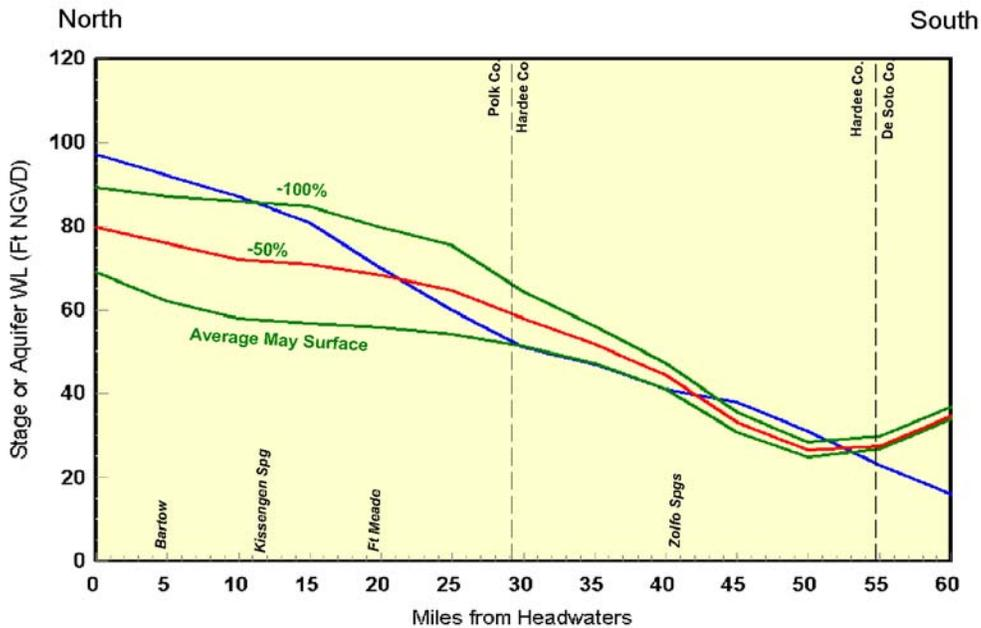
**Figure 57.** Predicted increase in the elevation of the Upper Floridan aquifer potentiometric surface during May due to reduction in pumpage of 50 and 100 percent in a 676 square-mile area.
