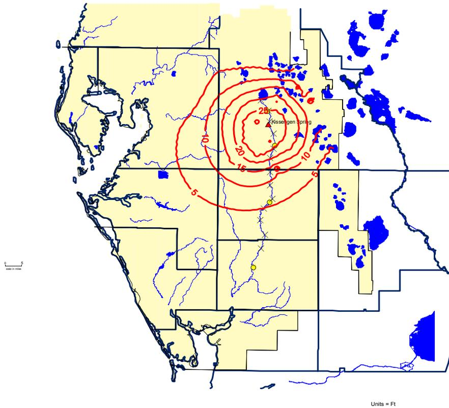
**Figure 56.** Simulated increase in Upper Floridan aquifer potentiometric surface when April-May ground-water withdrawals are reduced 100 percent within the 676 square-mile area.
