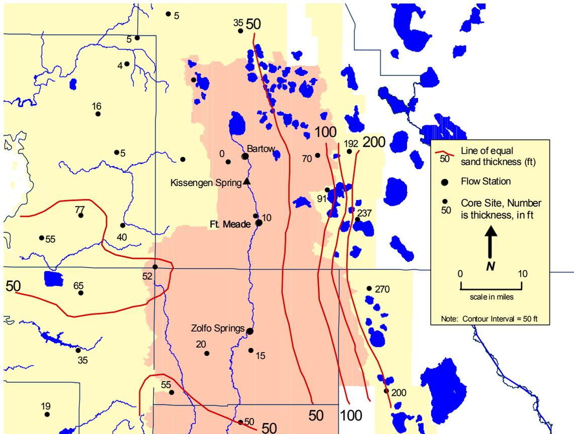
**Figure 9.** Sand thickness of the surficial aquifer.
