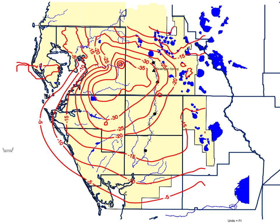
**Figure 52.** Simulated increase in Upper Floridan aquifer potentiometric surface when April-May ground-water withdrawals are reduced 80 percent across SWCFGWB.
