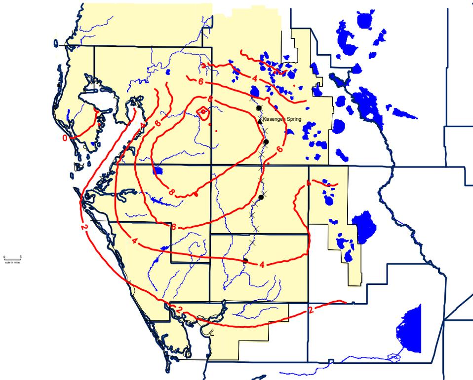
**Figure 50.** Simulated increase in Upper Floridan aquifer potentiometric surface when April-May ground-water withdrawals are reduced 20 percent across SWCFGWB.
