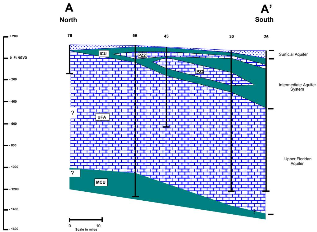
Figure 7. Hydrogeologic cross-section A-A'.
