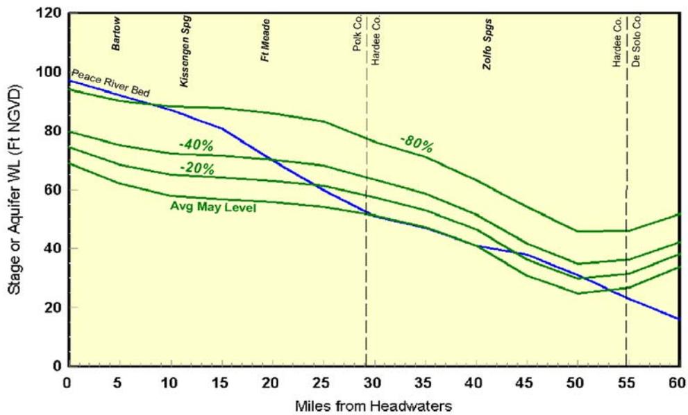
**Figure 54.** Predicted increase in the elevation of the Upper Floridan aquifer potentiometric surface during May due to reductions in pumpage of 20, 40, and 80 percent.
