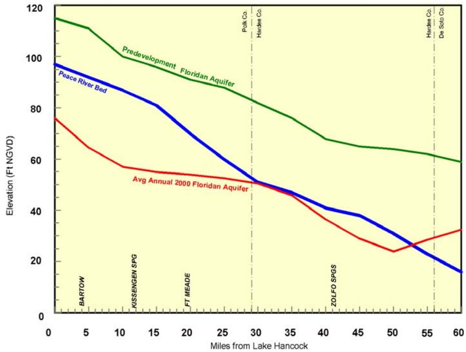
**Figure 28.** Hydrologic cross-section showing the relation between Peace River bed and the 2000 average annual potentiometric surface of the Upper Florida aquifer (modified from Lewelling and others, 1998).
