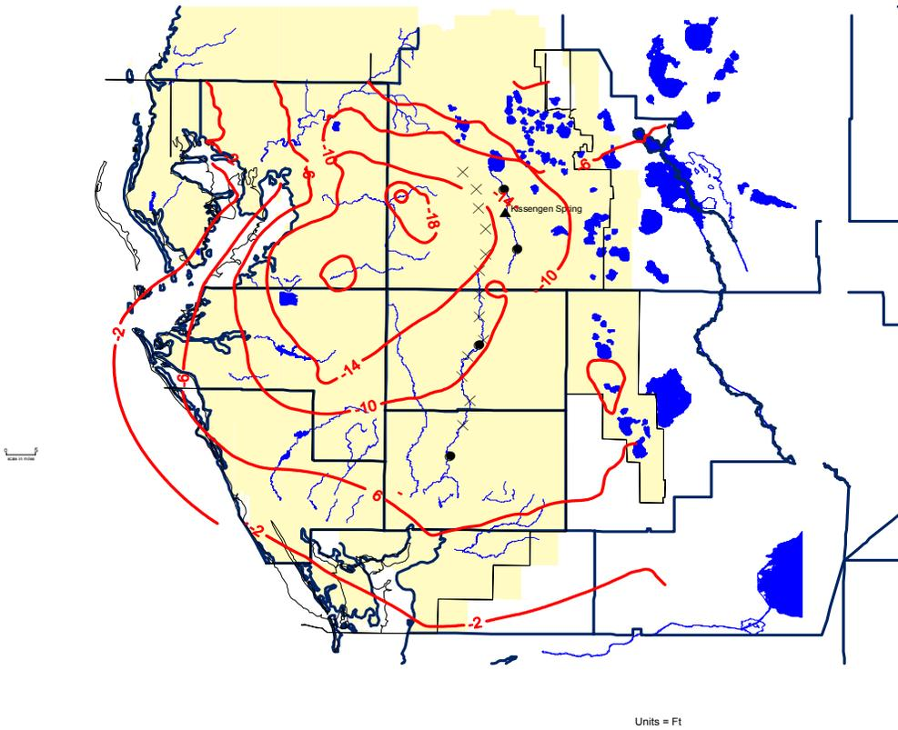
**Figure 51.** Simulated increase in Upper Floridan aquifer potentiometric surface when April-May ground-water withdrawals are reduced 40 percent across SWCFGWB.
