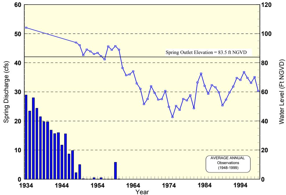
**Figure 41.** Comparison of Kissengen Spring discharge and Upper Floridan aquifer water levels (1934-1999).
