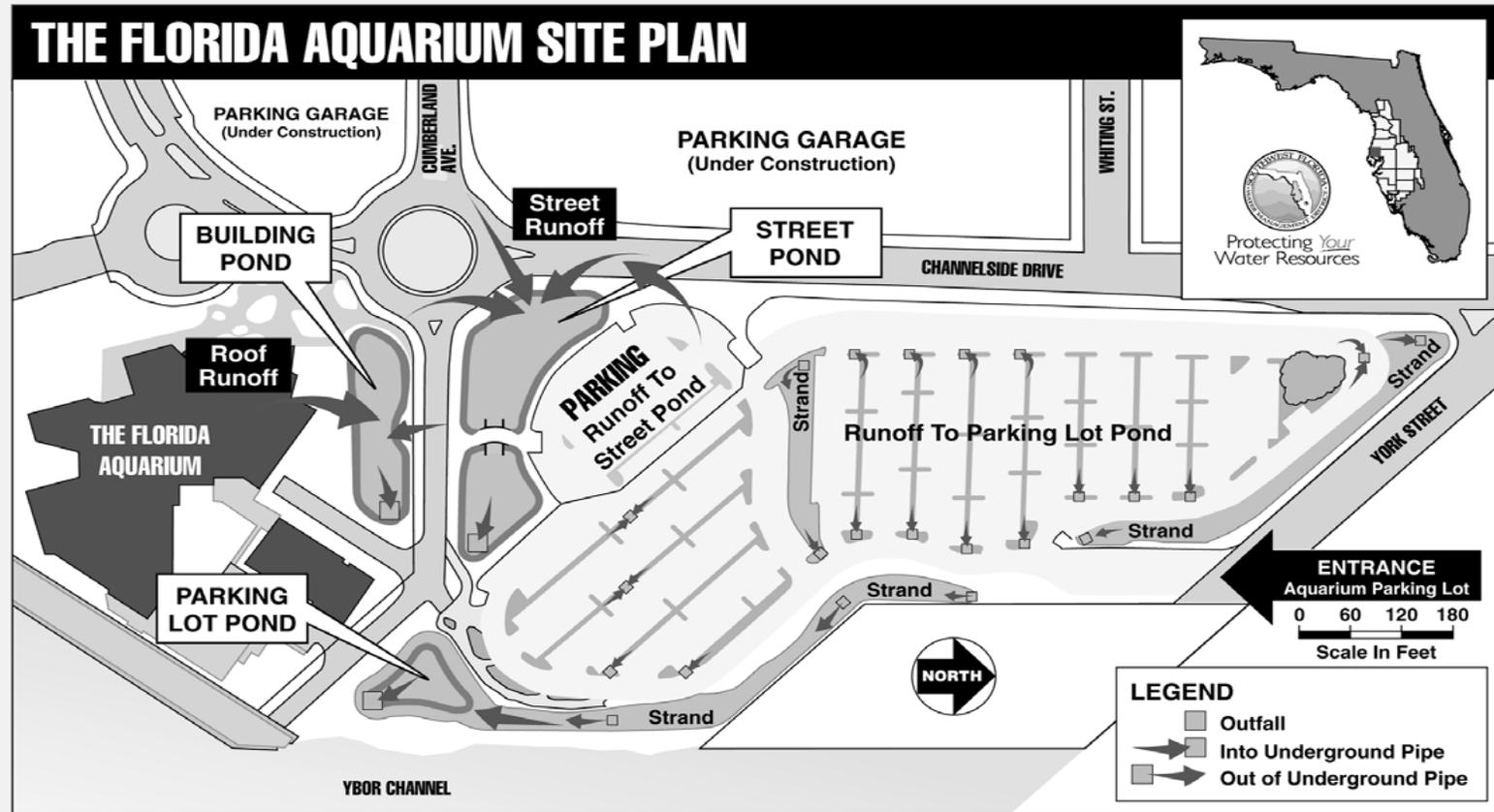
Figure 1a. Site plan showing the three stormwater ponds and the layout of the whole basin stormwater system used for the Parking Lot Pond.
