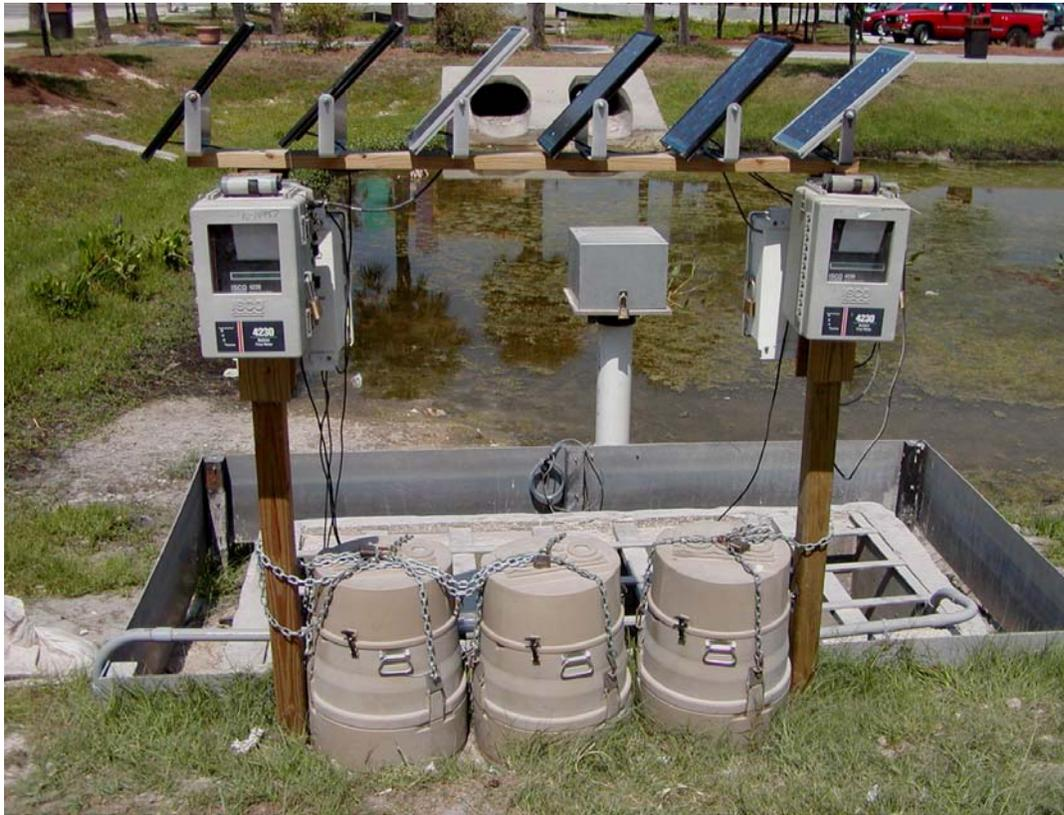
SAMPLING EQUIPMENT FOR DETAILED STUDY SHOWING FLOW METERS AND SAMPLERS AT OUTFLOW
