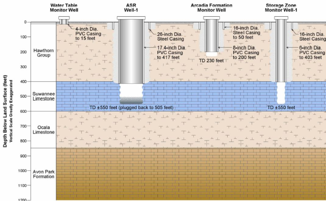
**Figure 5 Bradenton ASR Well Profile and Hydrogeologic Cross-Section**
