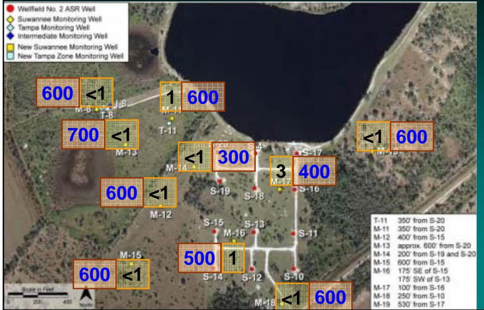
**Approximate Suwannee Limestone As ( $\mu\text{g/L}$ ) and TDS (mg/L) concentrations after Cycle 5 Recovery (July 2006)**
