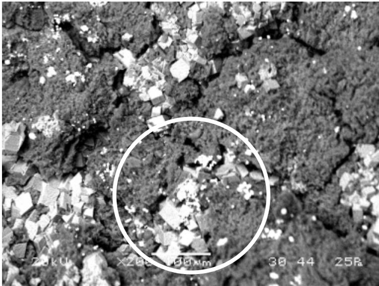
**Figure B4.** SEM image of sample from boring SZMW-7, Suwannee Limestone, 320-330 ft bls (approximately 321 ft bls). Image is 200X. White crystals are euhedral pyrite embedded in limestone matrix. Area in circle is shown in Figure B5.
