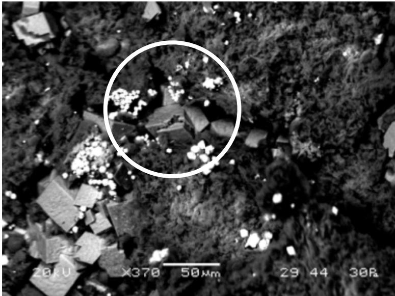
**Figure B5.** SEM image of sample from boring SZMW-7, Suwannee Limestone, 320-330 ft bls (approximately 321 ft bls). Image is 370X, a detail from Figure B4. Large euhedral cubic pyrite crystals occur with framboidal pyrite. Framboidal pyrite appears as white spots. Area in circle is shown in Figure B6.
