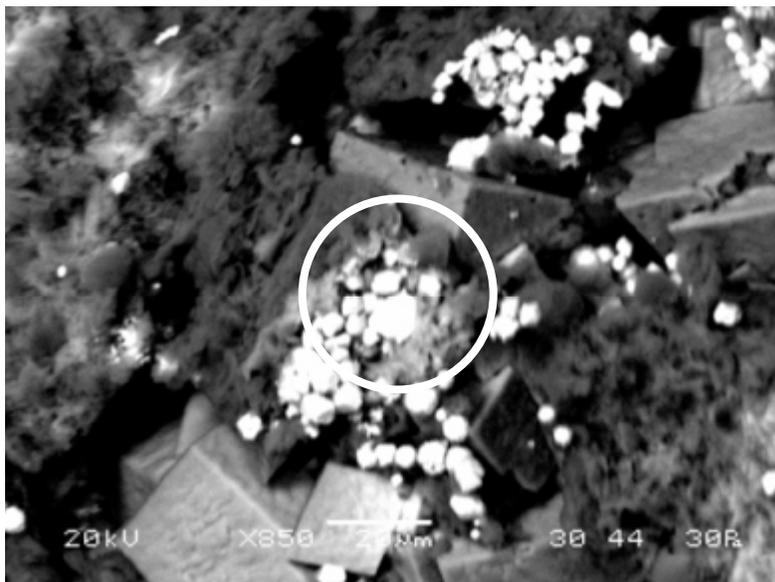
**Figure B6.** SEM image of sample from boring SZMW-7, Suwannee Limestone, 320-330 ft bls (approximately 321 ft bls). Image is 850X, a detail from Figure B5. Large euhedral cubic pyrite crystals occur with framboidal pyrite. Framboidal pyrite appears as white spots. Area in circle is shown in Figure B7.
