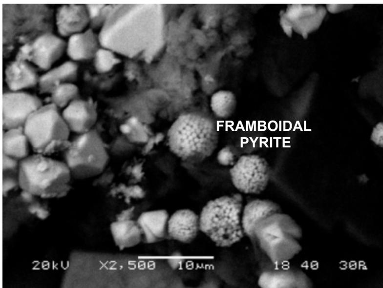
**Figure B8.** SEM image of sample from boring SZMW-7, Suwannee Limestone, 320-330 ft bls (approximately 321 ft bls). Image is 2,500X, and shows detail of euhedral and framboidal pyrite, similar to Figure B7.
