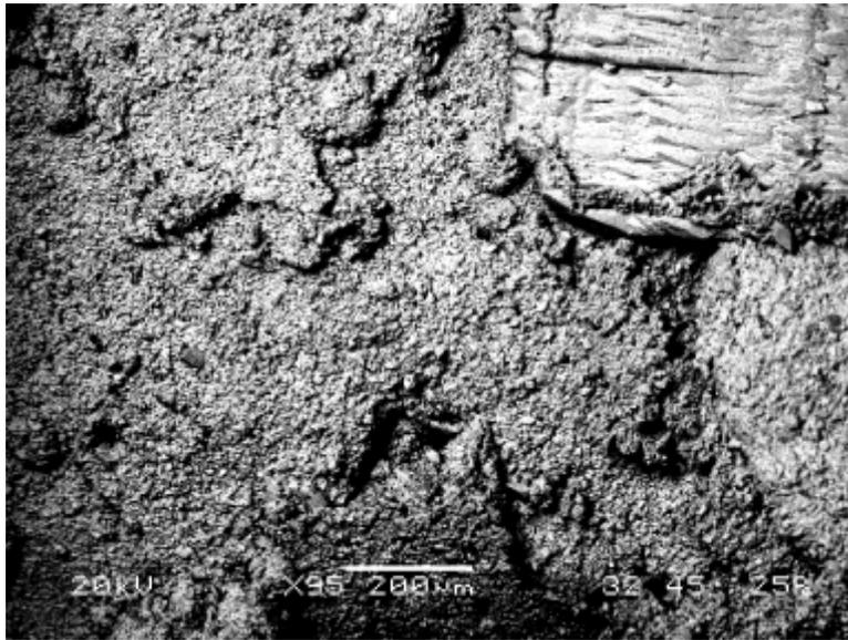
**Figure B1.** Scanning Electron Micrograph (SEM) image of sample from boring SZMW-9, Suwannee Limestone, 301-303 ft below land surface (bls). Boring obtained at the Tampa-Rome Avenue Park ASR system. Image is 95X. Image shows texture of bulk limestone.
