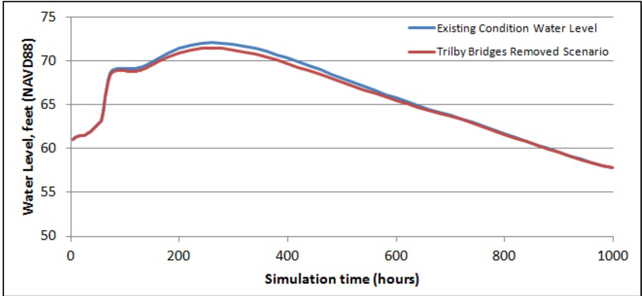
**Figure 5-7 Upstream Side of SR 575 during the 100-year Design Storm**
