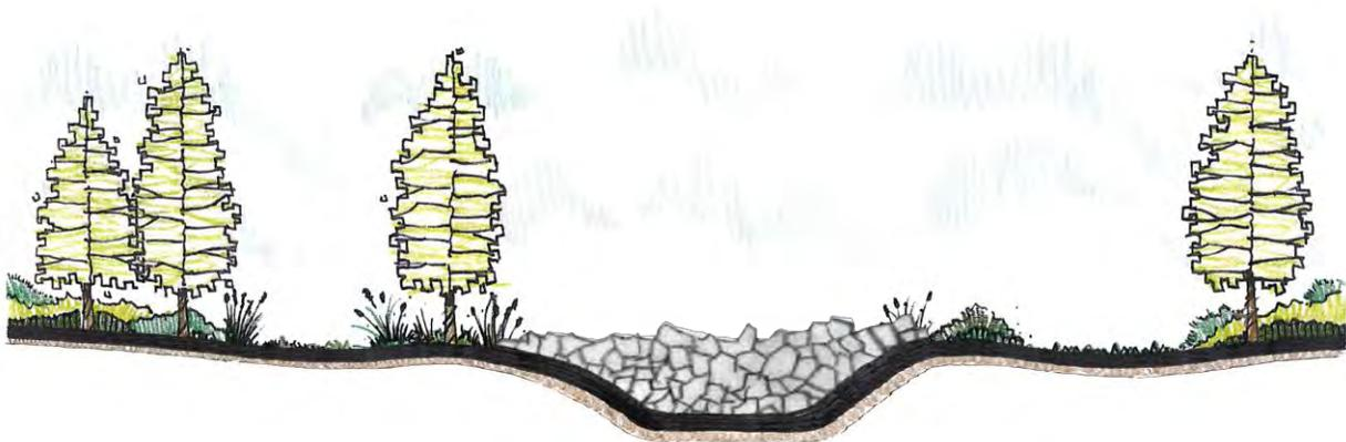
**Figure 17-3 River Channel with the Addition of Rocks**
