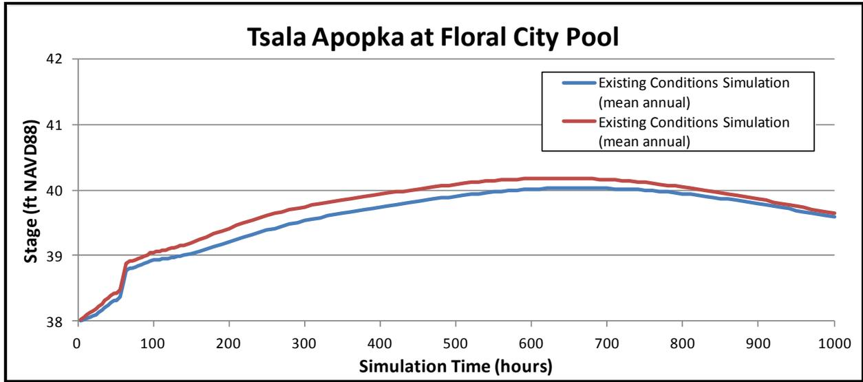
**Figure 12-6 Comparison of Water Levels in the Floral City Pool for the Mean Design Storm Event**
