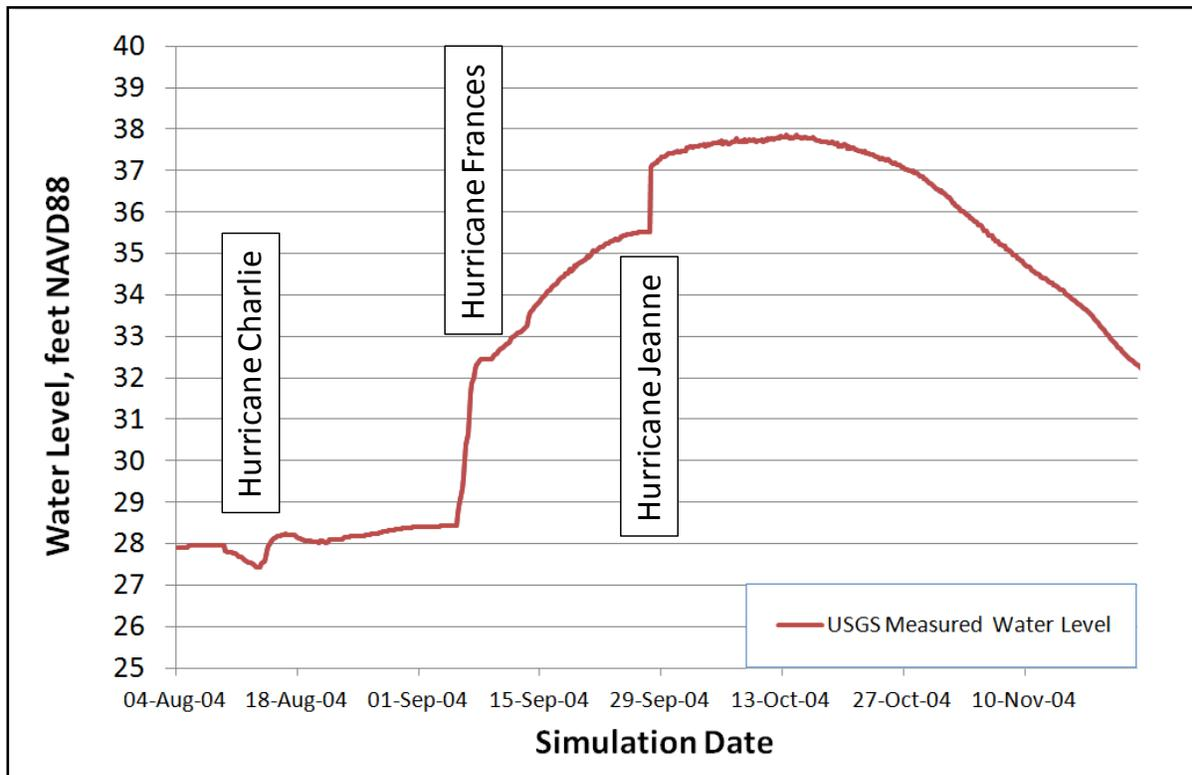
**Figure 9-1 Water Levels on the Withlacoochee River at SR 200 during the 2004 Hurricanes**
