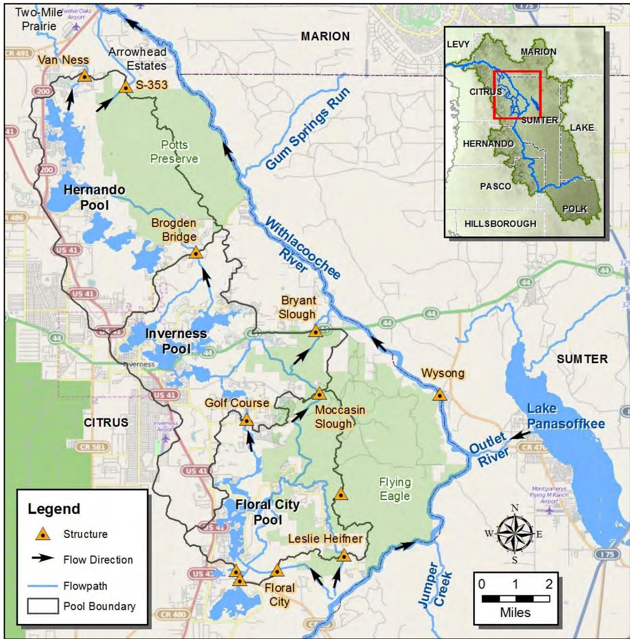
Figure 13-1 Flowpaths, Structures and Pools within the Tsala Apopka Chain-of-lakes
