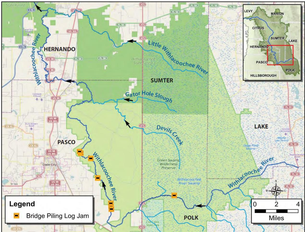
**Figure 2-2 Bridge Piling Log Jams along the Withlacoochee River in the Green Swamp**
