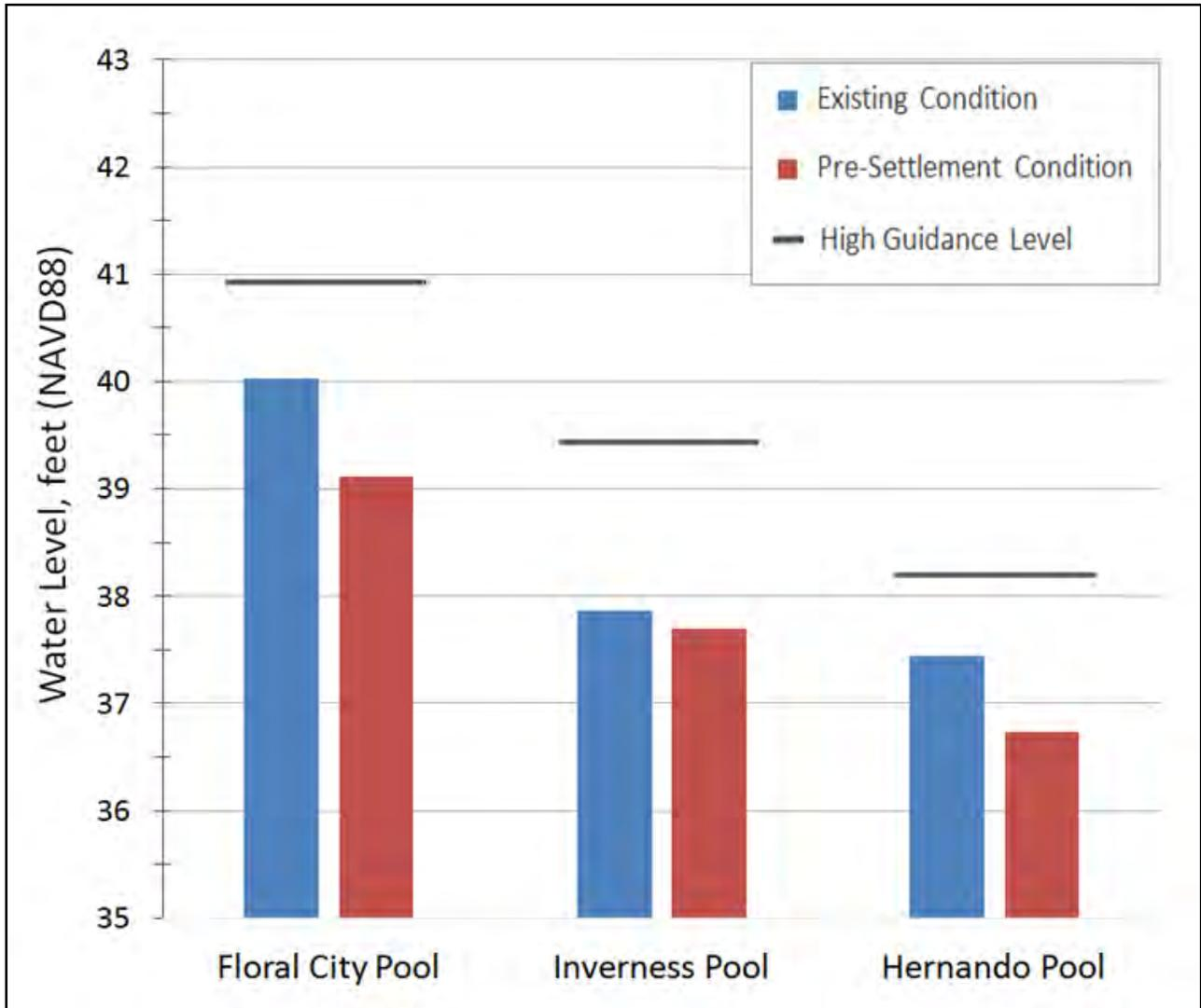
**Figure 11-8 Comparison of Peak Water Levels during the Mean Annual Storm Event**
