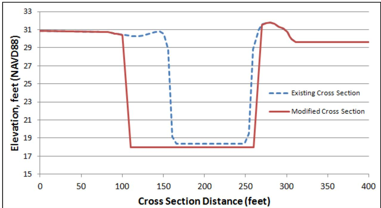
**Figure 18-4 Comparison of Existing and Modified Bypass Channel Cross Section**
