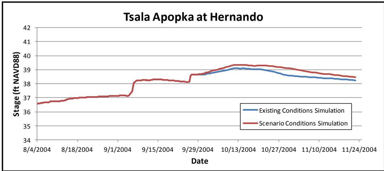
**Figure 15-3 Comparison of Water Levels in the Hernando Pool during the 2004 Hurricanes**
