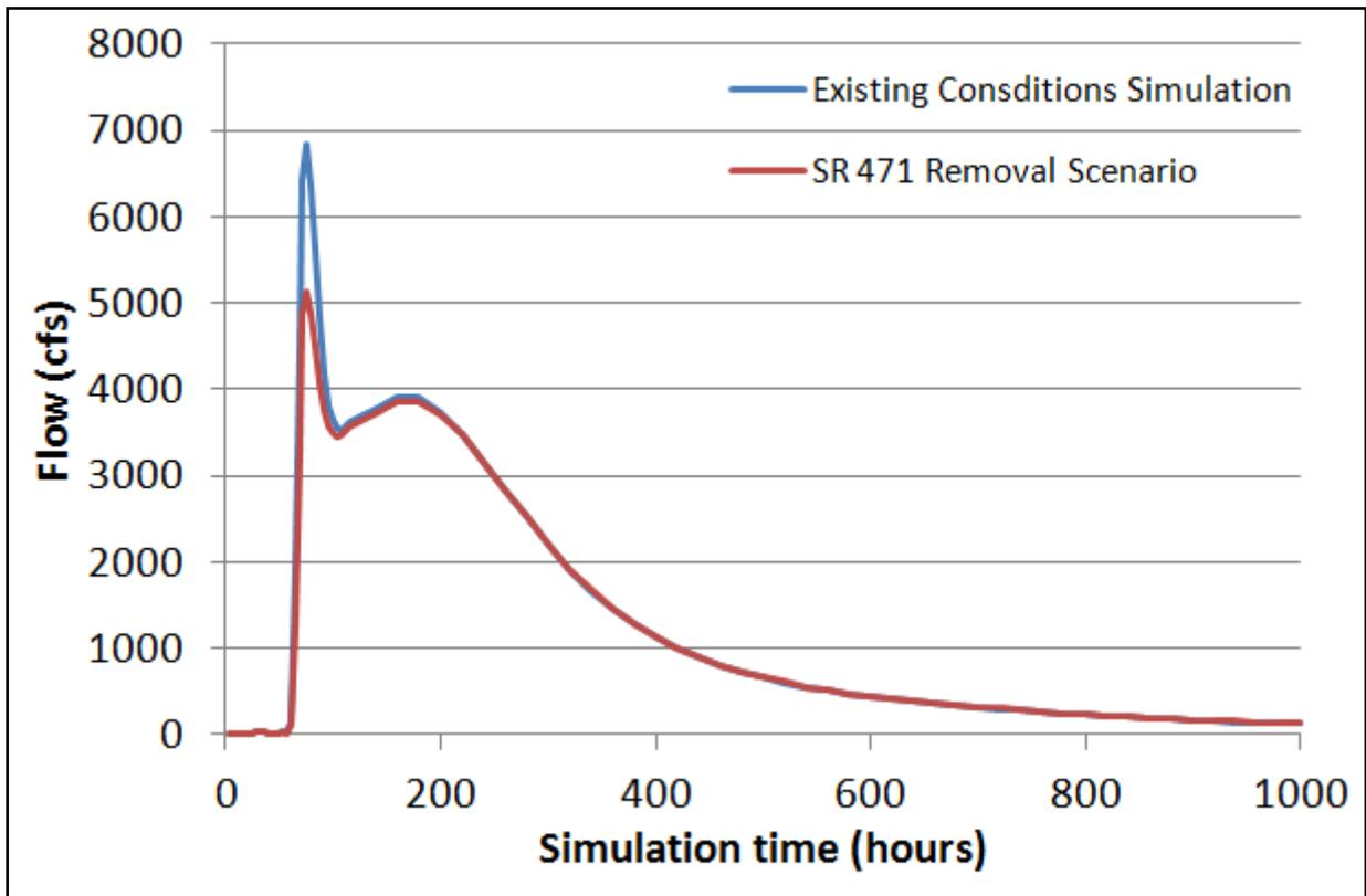
**Figure 3-4 Comparison of Flows on the Withlacoochee River at SR 471 for the 100-year Storm Event**
