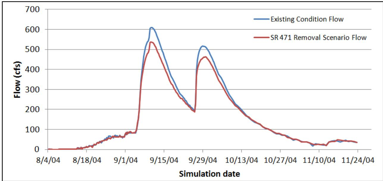
**Figure 3-5 Comparison of Flows for the Little Withlacoochee River at SR 471**
