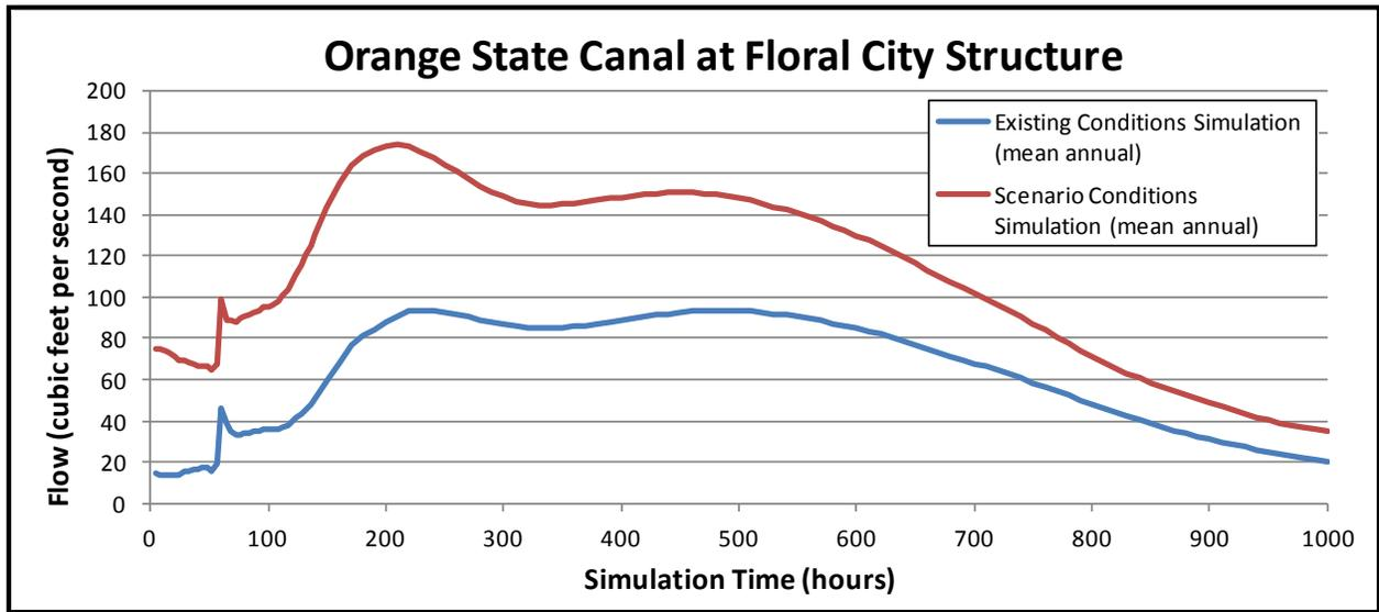
**Figure 12-4 Orange State Canal Flow Comparison – Mean Annual Storm Event**
