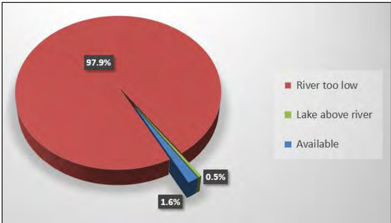
**Figure 6-4 Availability of River Water to enter Lake Oriole under Natural Conditions**
