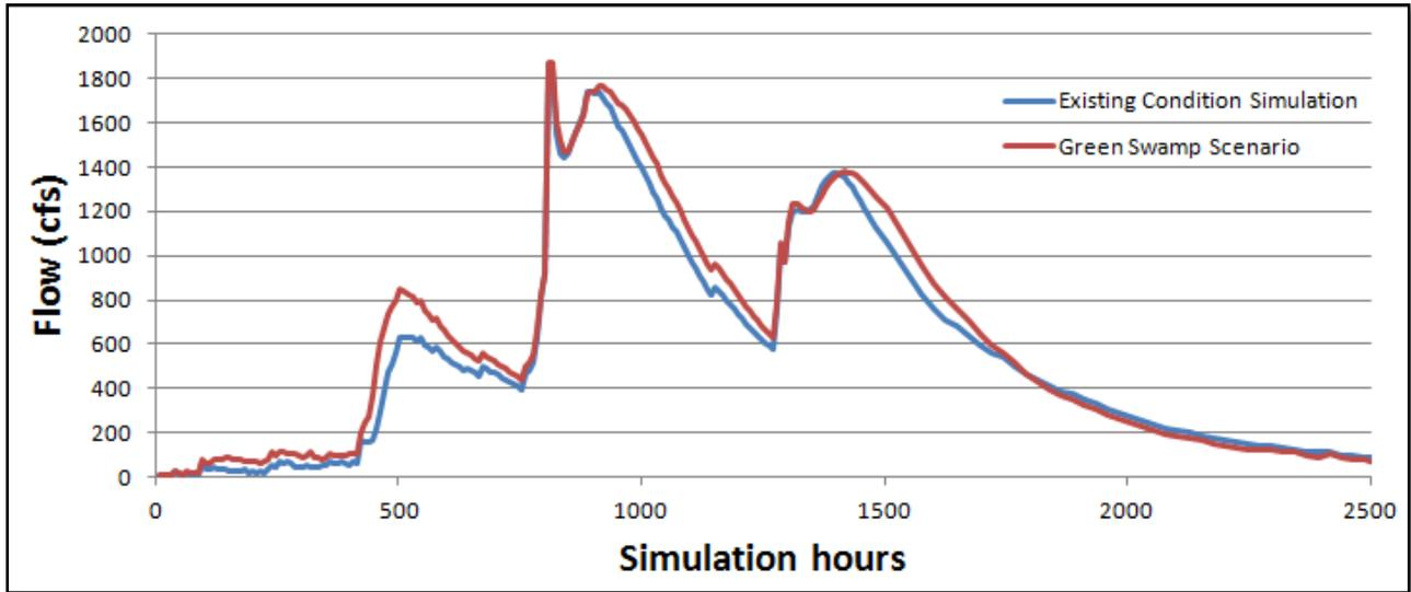
**Figure 1-7 Comparison of Flows for the Withlacoochee River at SR 471 for the 2004 Hurricanes**
