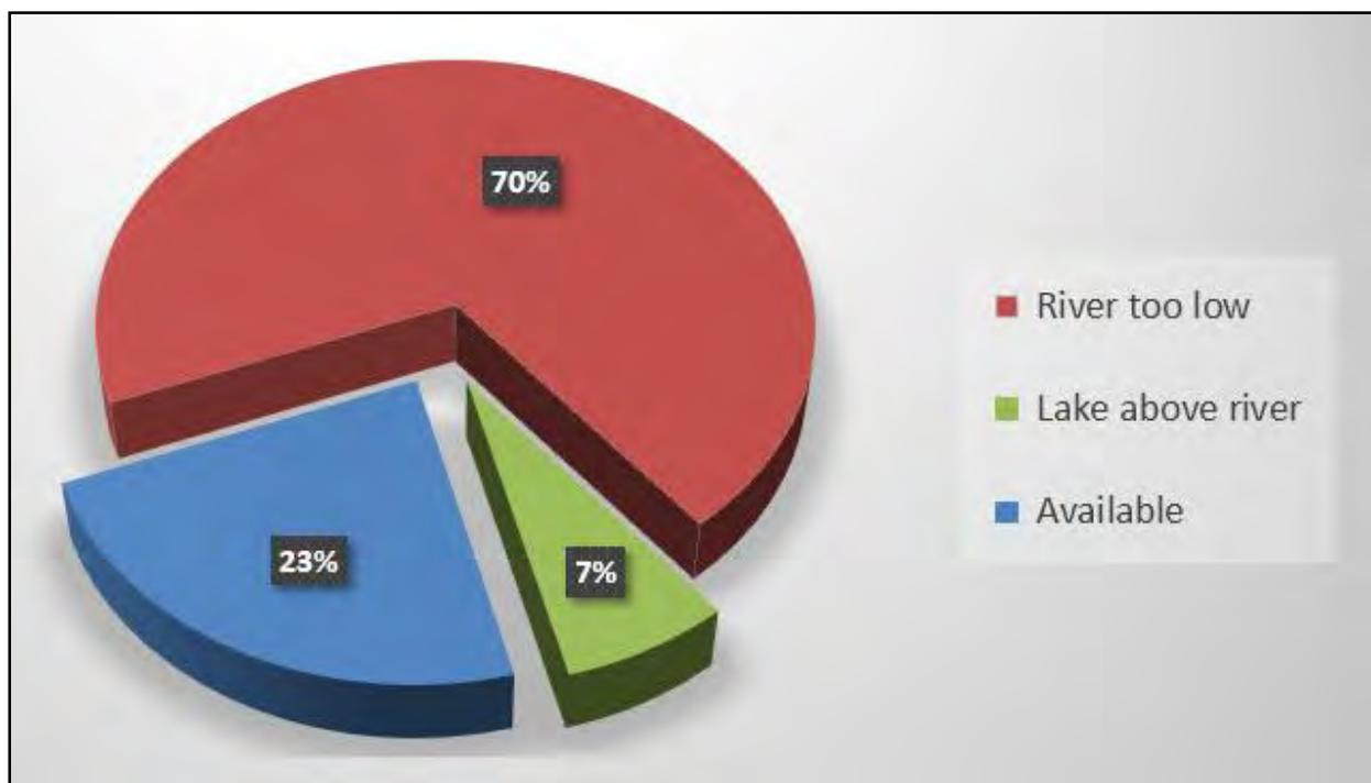
**Figure 6-7 Availability of River Water to enter Lake Oriole under Simulated Conditions**
