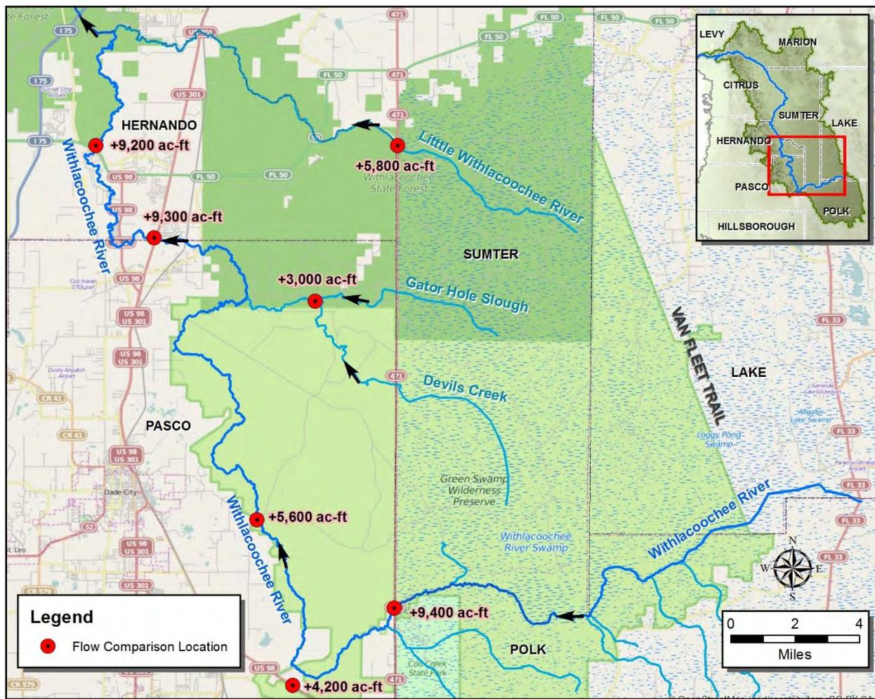
Figure 1-9 Flow Volume Increases (acre-feet) with Historical Railroad Berms Removed
