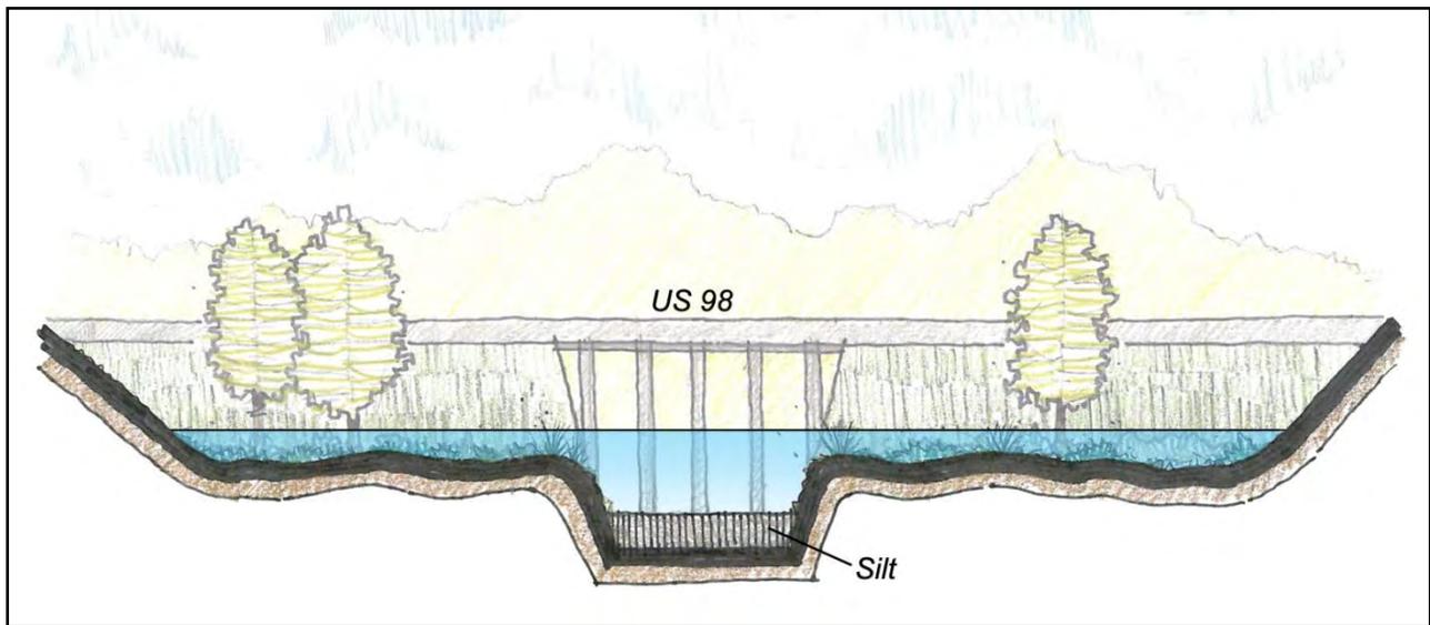
**Figure 4-4 Comparison of the Current US 98 Bridge Opening to the Natural Flow Path (black line)**
