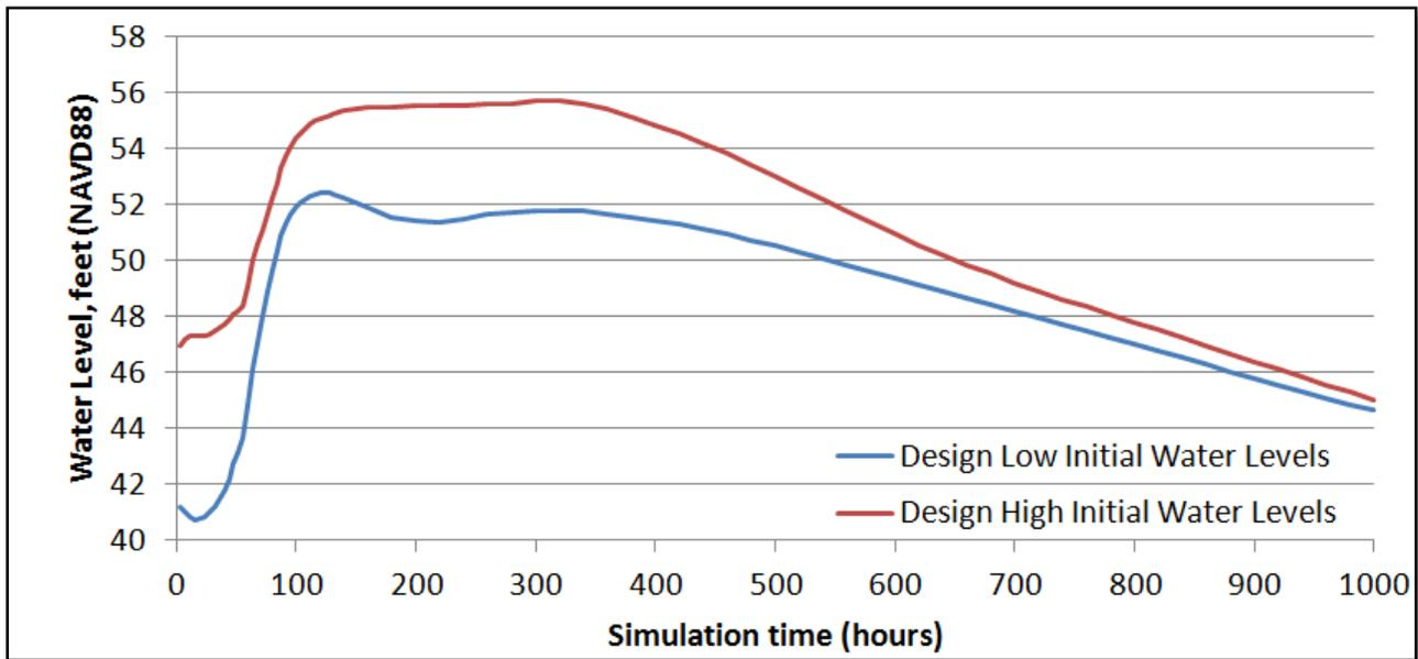
**Figure 9-6 Comparison of Water Levels on the Withlacoochee River at Croom for the 100-Year Storm Event**
