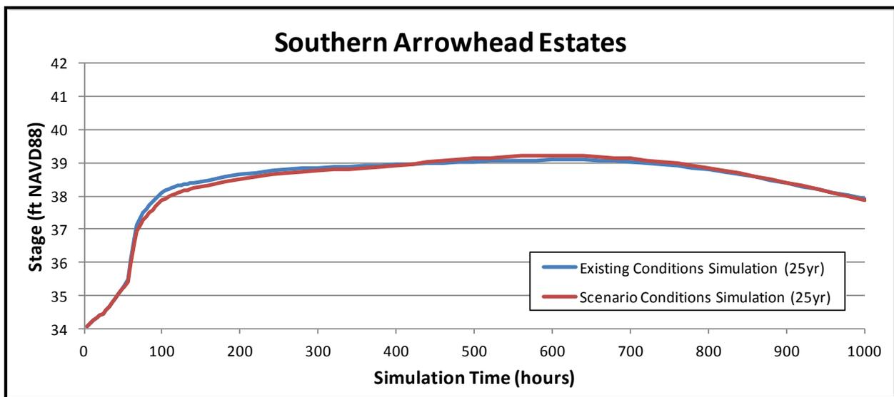
**Figure 15-4 Comparison of Water Levels at Arrowhead Estates during the 25-Year Design Storm Event**
