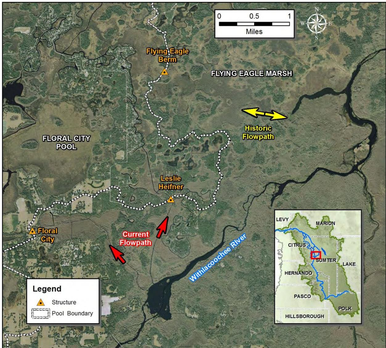
**Figure 10-2 Comparison of Current and Historical Flowpaths between the Withlacoochee River and the Tsala Apopka Chain-of-lakes**
