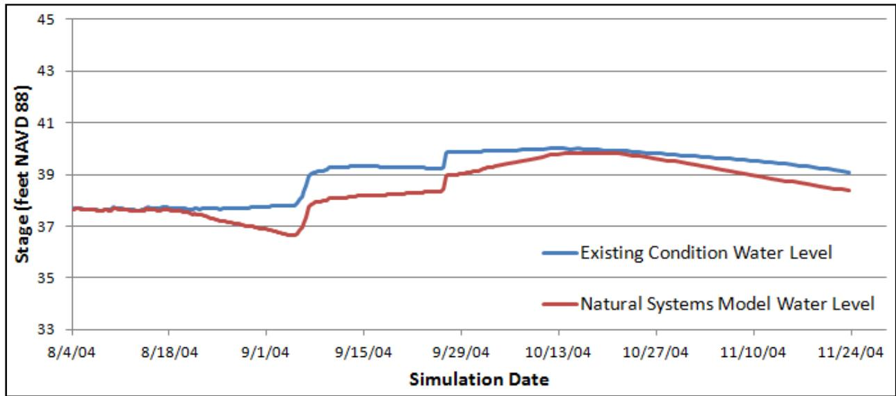
**Figure 11-5 Comparison of Water Levels in the Inverness Pool during the 2004 Hurricanes**
