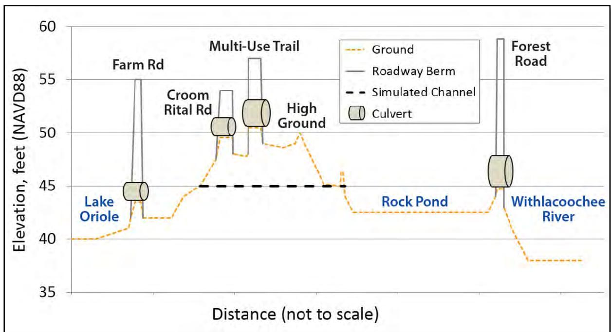
**Figure 6-3 Profile of Ground and Culvert Elevations between Lake Oriole and the Withlacoochee River**
