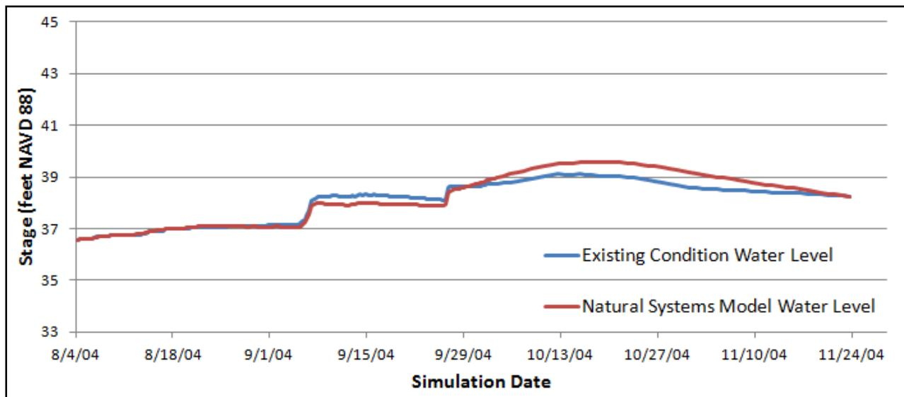
**Figure 11-6 Comparison of Water Levels in the Hernando Pool during the 2004 Hurricanes**
