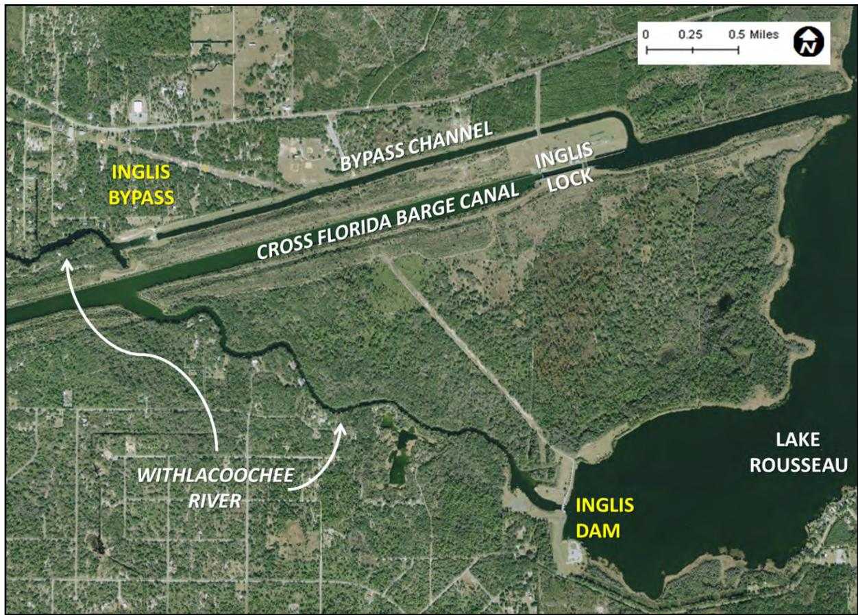
**Figure 18-2 Outflow Channels and Structures at Lake Rousseau**
