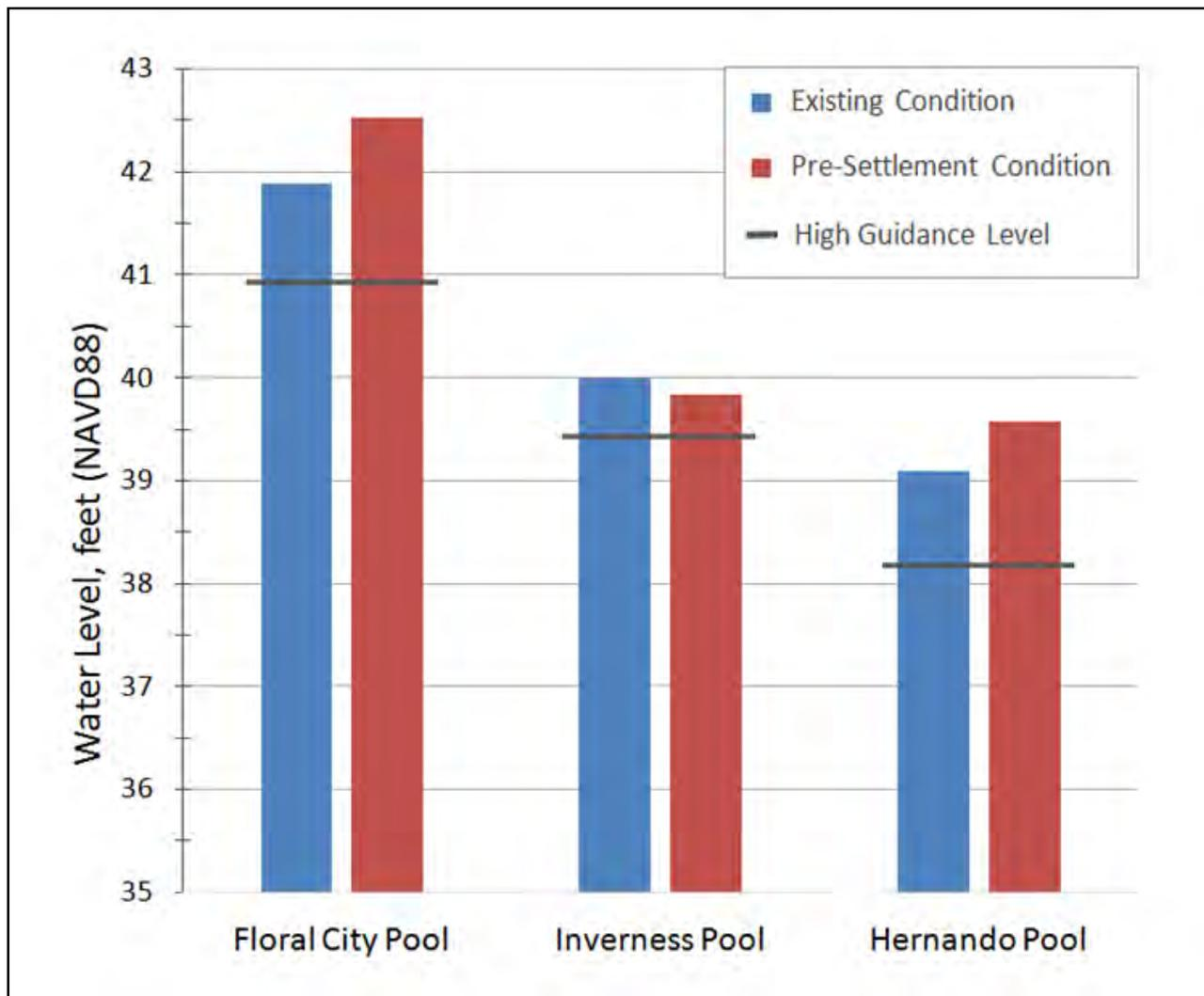
**Figure 11-7 Comparison of Peak Water Levels during the 2004 Hurricanes**
