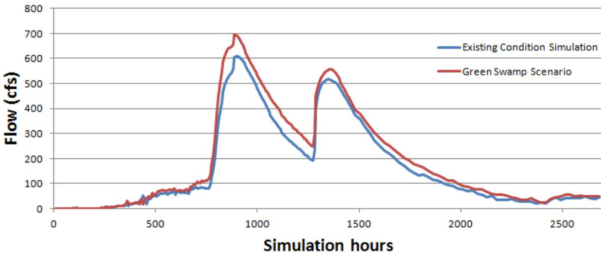
**Figure 1-6 Comparison of Flows for the Little Withlacoochee River at SR 471 for the 2004 Hurricanes**
