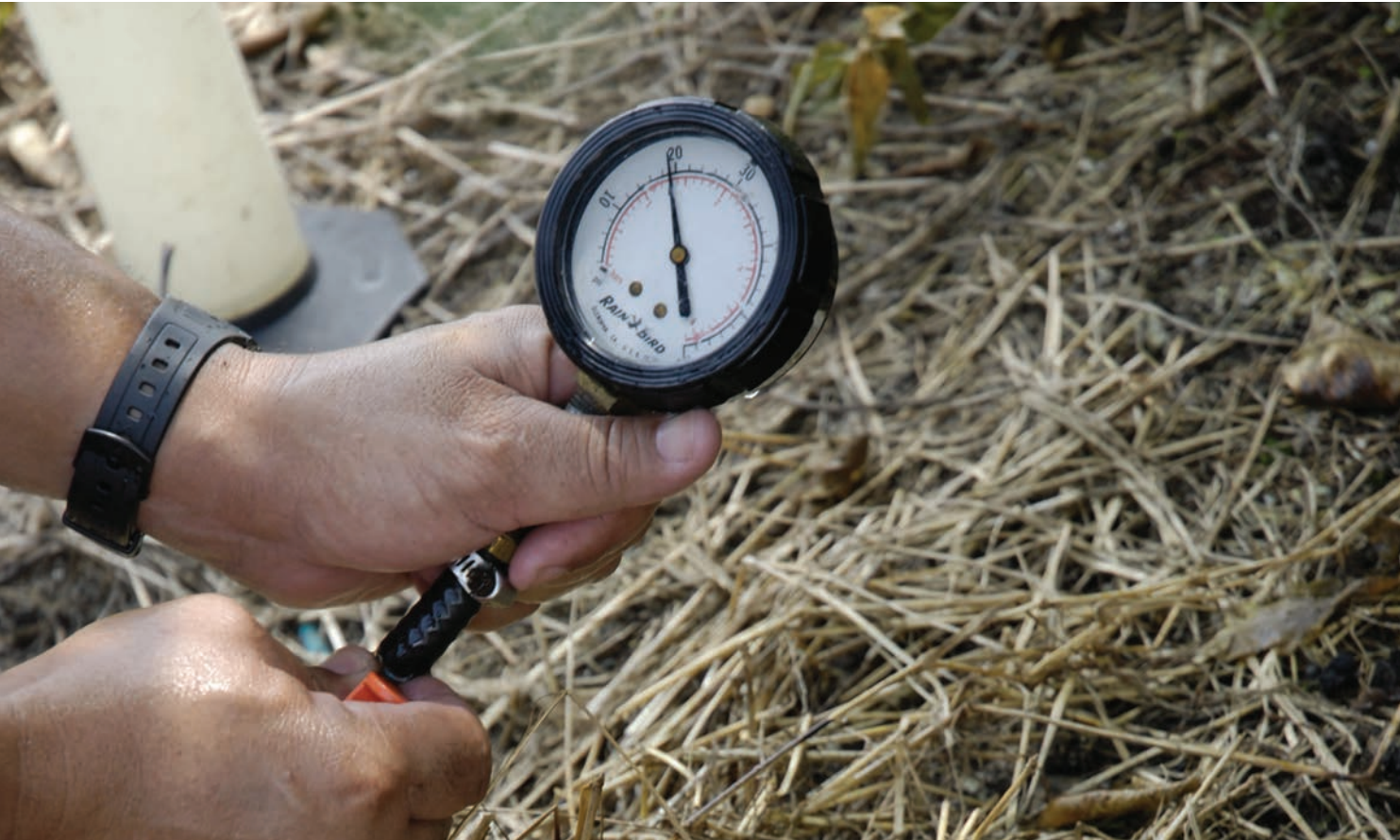
An irrigation test performed through the MIL to check the uniformity of water delivery and identify irrigation system deficiencies.
