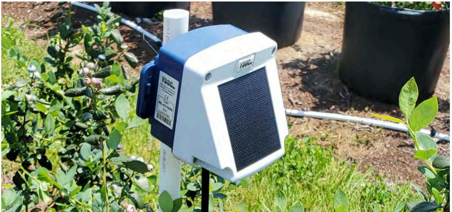
A solar powered soil moisture probe installed at Thayer Berry Hill in Polk County through the Mini-FARMS program. The probe provides real-time data on water and nutrient levels to allow the grower to efficiently manage their irrigation and nutrient scheduling.
