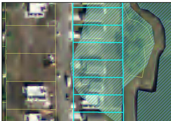
Figure 2. Example of inconsistencies between wetland delineation and residential parcels (outlined here in light blue)
