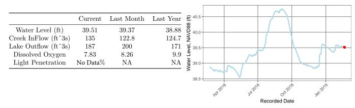
Dissolved Oxygen (DO), and Light Penetration are recorded at Lake Panasoffkee. These parameters are taken from the North and South side of the lake, the middle of the lake, and the outlet canal of the lake. DO indicates the amount of oxygen present in the water. This affects the lakes ability to support life. Light Penetration indicates the available sunlight reaching the lake bottom as a percentage.
