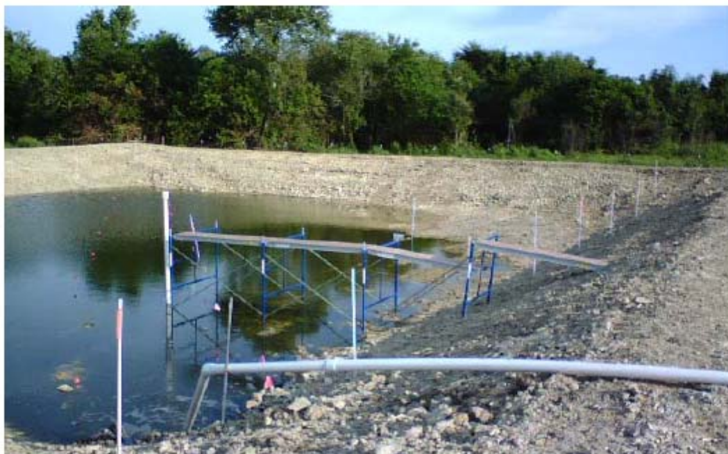
EXHIBIT 2-7 Water Level Recorder, Staff Gauge, Water Distribution Pipe, and Sampling Boardwalk at the Lake Hancock Plant Establishment Study Cells
