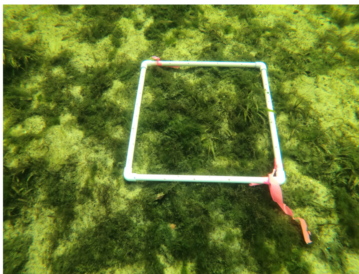
Figure 8: A quadrat is used to measure percent coverage of SAV species in the Homosassa River.
