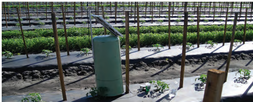
A soil moisture sensor that relays readings back to a central control unit to indicate irrigation needs to the grower.
