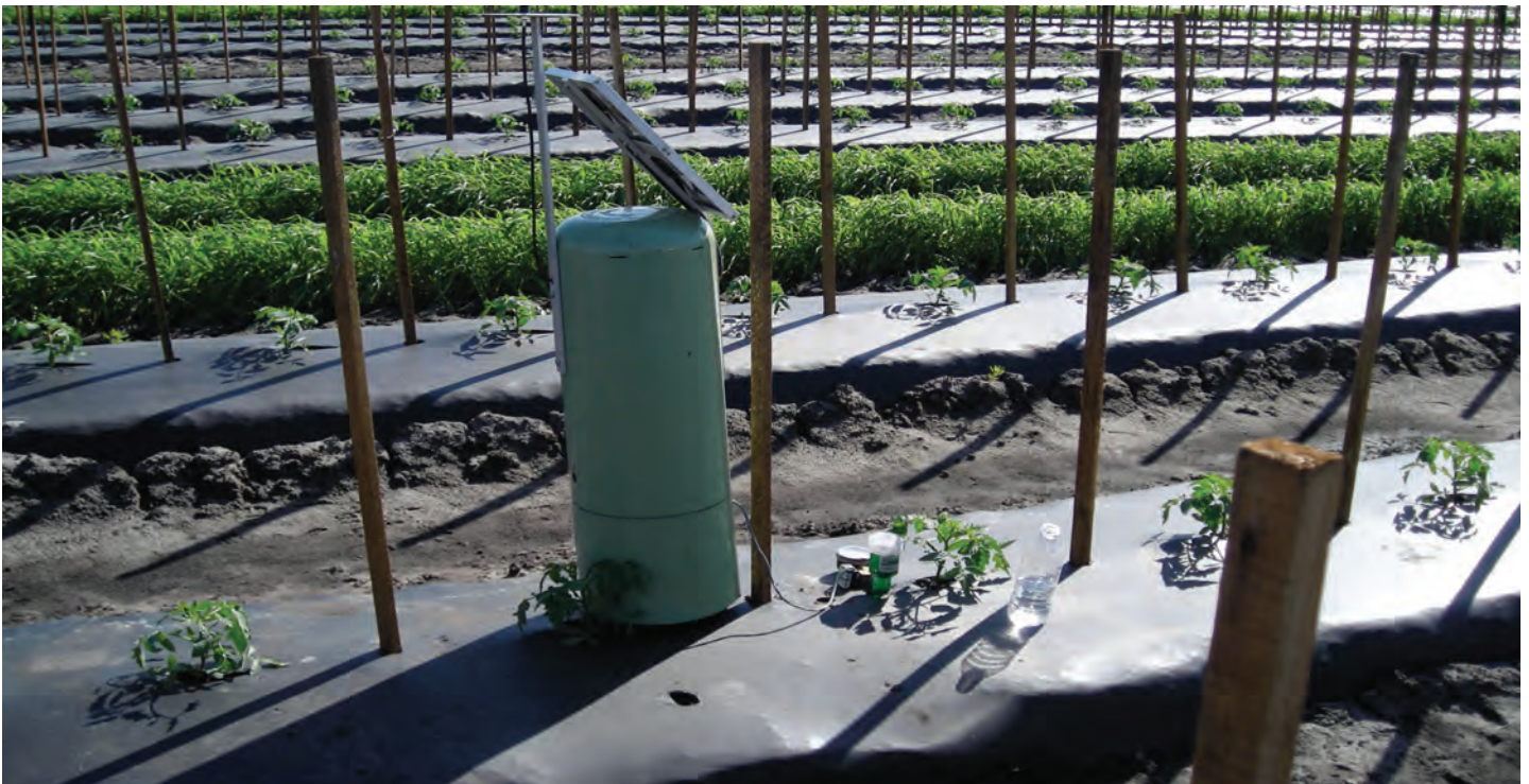
A soil moisture sensor that relays readings back to a central control unit to indicate irrigation needs to the grower.
