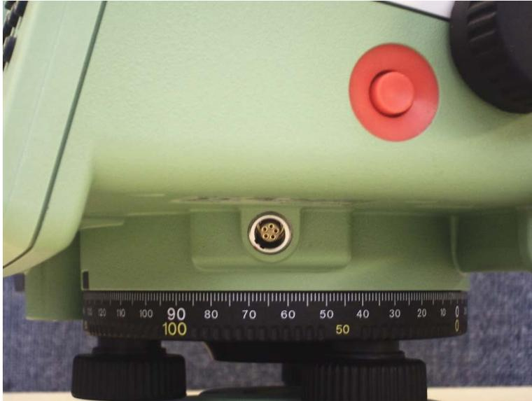
**\*NOTE\***-Also shown in this picture is the RS-232 port for connecting a data collector if necessary.
