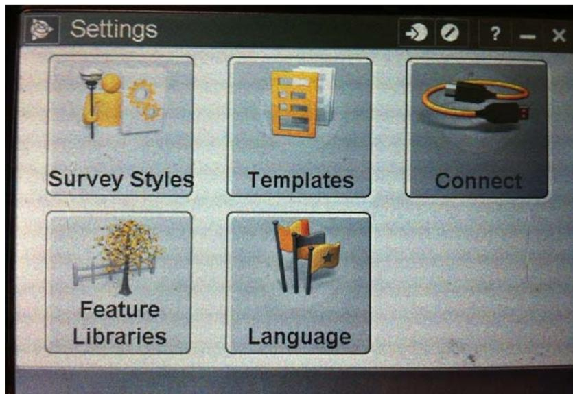
Select the **Connect** icon to go to the **Connections** screen then select **GNSS contacts**.
