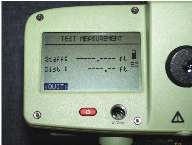
When you finish using the TEST MEASUREMENT screen you will need to highlight the <QUIT> tab as shown above to exit the TEST MEASUREMENT screen and return to your level screen. After shooting the back sight shot the Foresight screen will appear like below.
