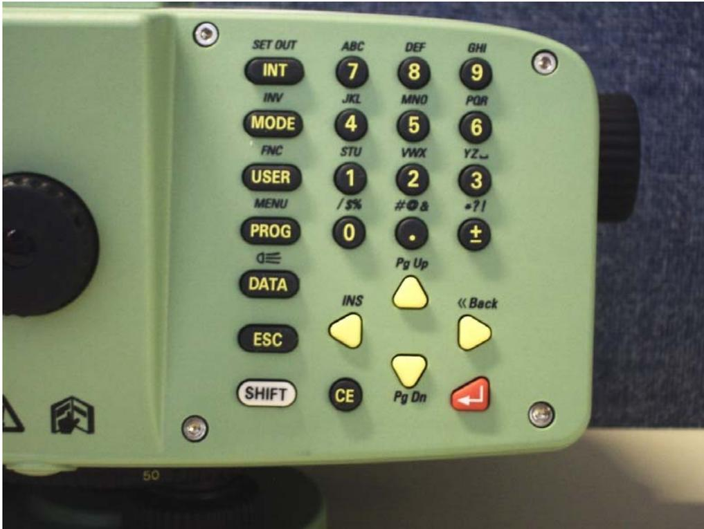
This keyboard uses the Tap method of entry, (like a cell phone), with the shift key allowing you to switch between the Alphabetic and Numeric forms of entry. You will note that there will be a symbol at the bottom of the screen for both modes and that they are different depending on what screen you are in.
