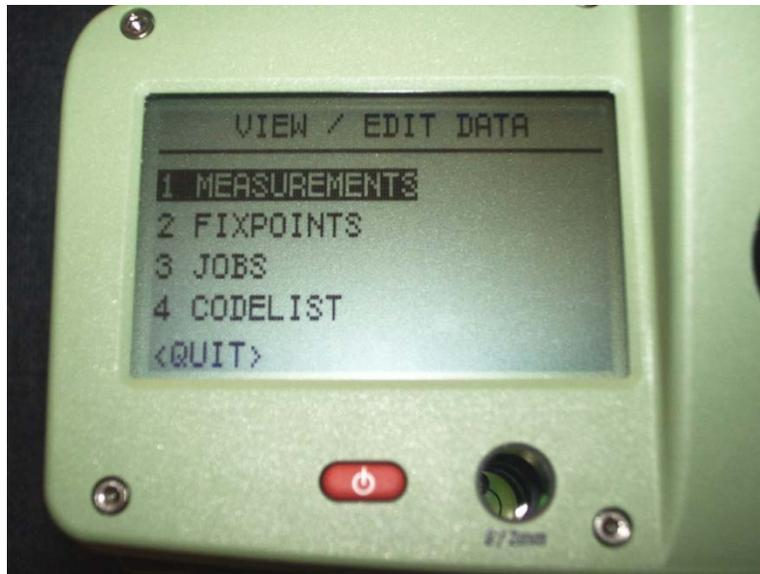
Choose the highlighted “1 MEASUREMENTS” tab to get to the “VIEW MEASUREMENT” screen shown below.
