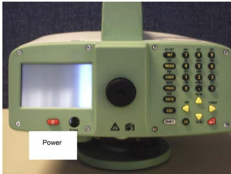
When turning the level on for the first time it will be in Measure and Record Mode. This is **NOT** the mode you will be using to do your task.
