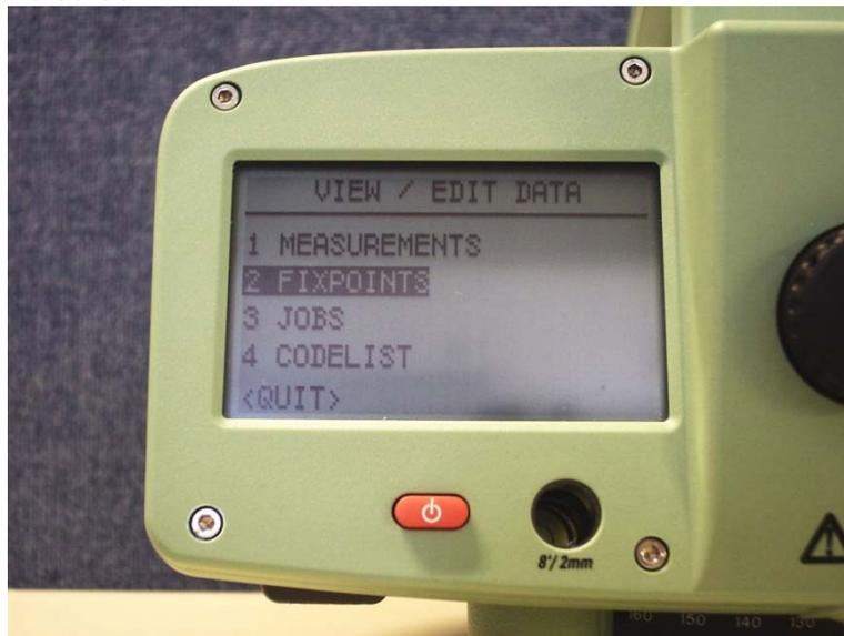
Push either the "2" or use the YELLOW arrows to navigate to the 2 FIXPOINTS line. You will now see the screen below. Use the YELLOW arrows to navigate to the <NEW/EDIT> tab at the bottom right of the screen and push the RED enter key.
