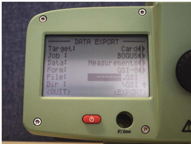
You need to navigate to the “FILE:” line as shown above and enter the work order number with NO dashes. If you enter dashes it will not accept the name and you will have to escape out to the beginning and start over with the export process. Press the RED enter key a second time and the <EXPORT> tab will be highlighted. Press the RED enter key.
