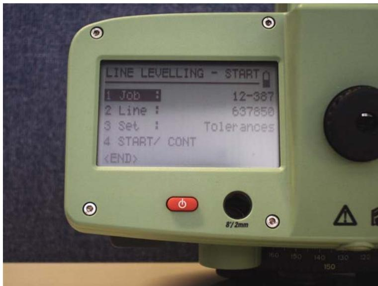
The "1 Job :" line will be highlighted. This is where you will enter the work order number of the job you are working on using the alphanumeric keyboard seen below.
