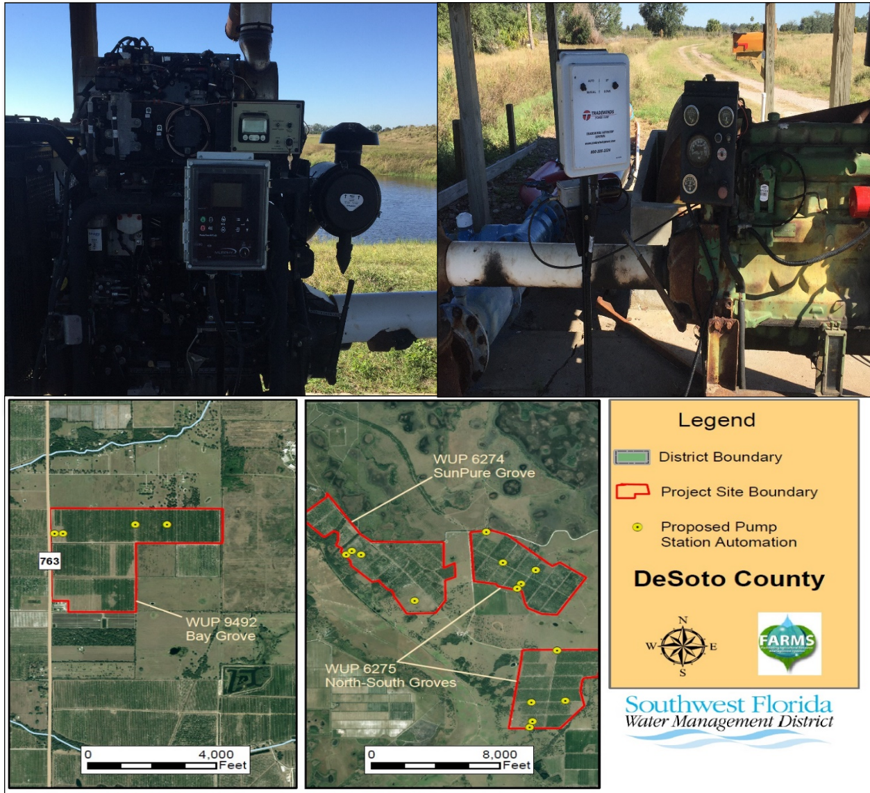
Figure 9. Left side shows auto-stop engine controls and the right side shows citrus groves pumping stations locations.
