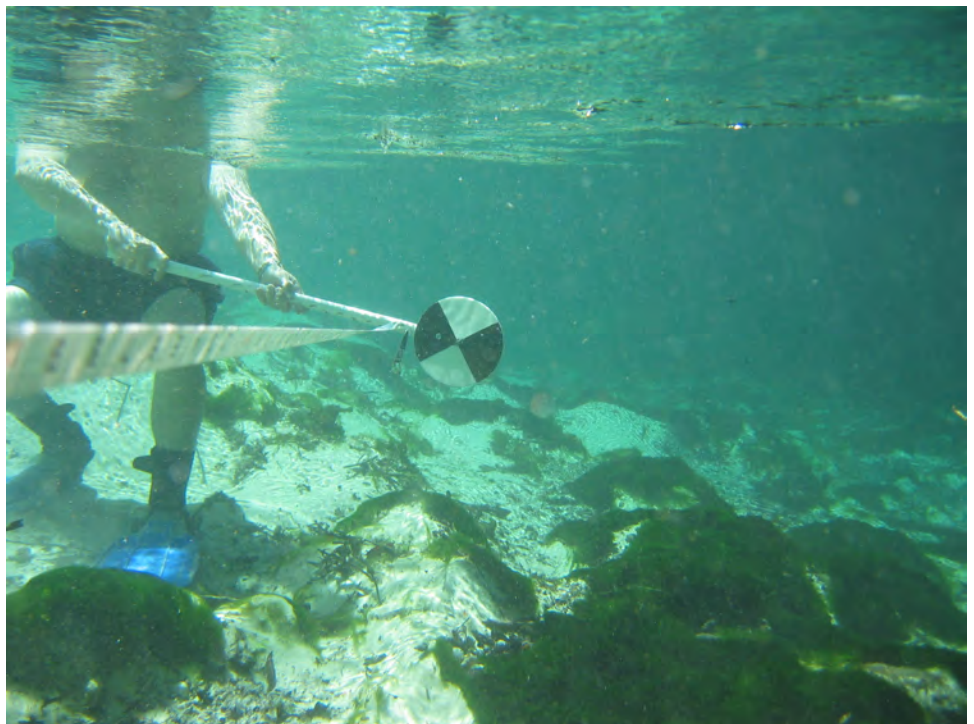
Figure 7: A secchi disk is used to measure water clarity.
