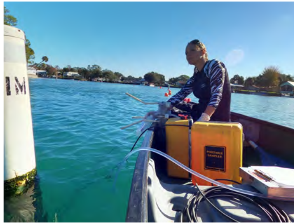
Figure 3: Water quality data collection at one of the sampling stations in Kings Bay.
