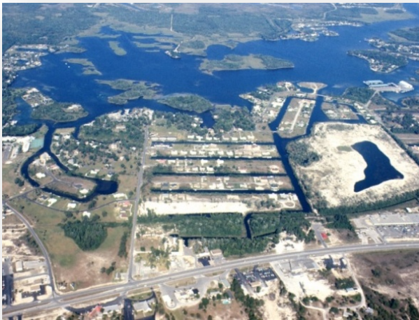
Aerial of Crystal River in 1977 showing the intense dredge and fill operations that destroyed many of the beneficial wetlands along the banks of Kings Bay.
