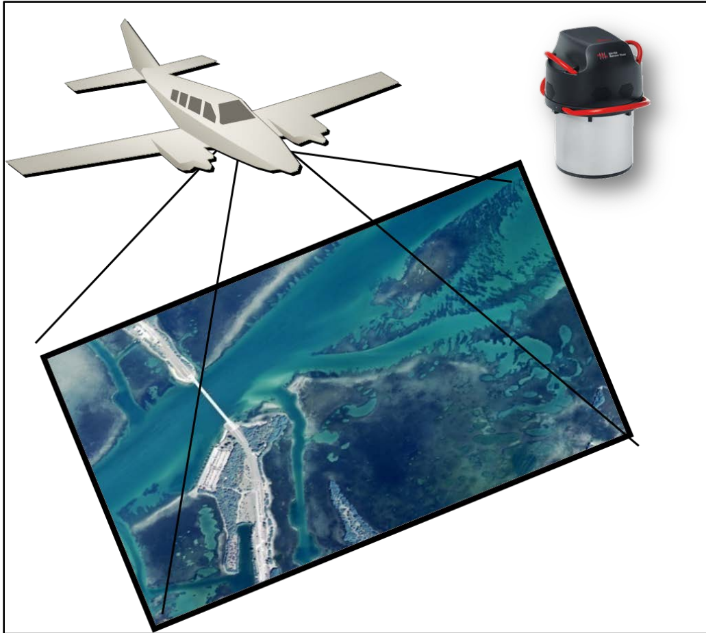
Figure 29 – SWFWMD seagrass mapping based on photointerpretation of aerial imagery. An aircraft is flown at an altitude of 8000-10000 feet. Imagery is collected using a digital camera mounted on the aircraft. Photo-interpreters then draw polygons on the imagery delineating areas of seagrass using a modified Florida Land Use Cover Classification Scheme (FLUCCS).
