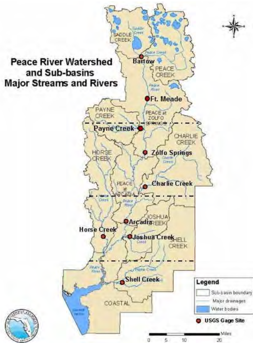
Figure 1. Map of Peace River watershed showing the main stem of river, major tributaries, and the locations of long-term USGS streamflow gages. Adapted from SWFWMD (2002).
