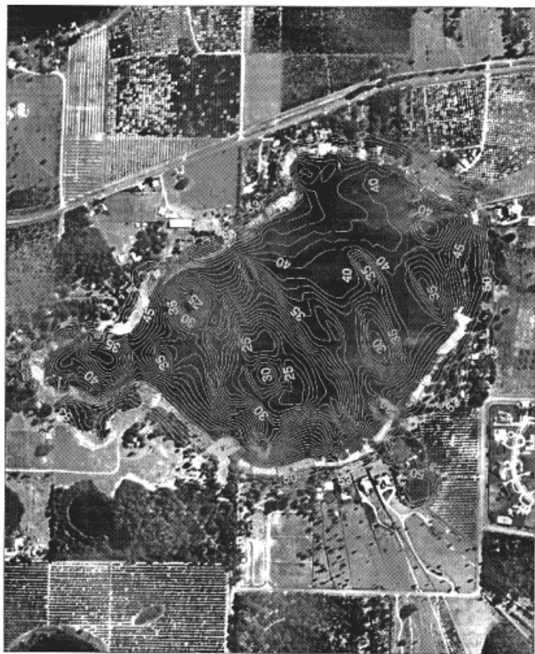
Figure 6-9. One-foot contour map of the Lake Calm basin, Hillsborough County, Florida. Values shown are elevations, in feet, above the National Geodetic Vertical Datum.
