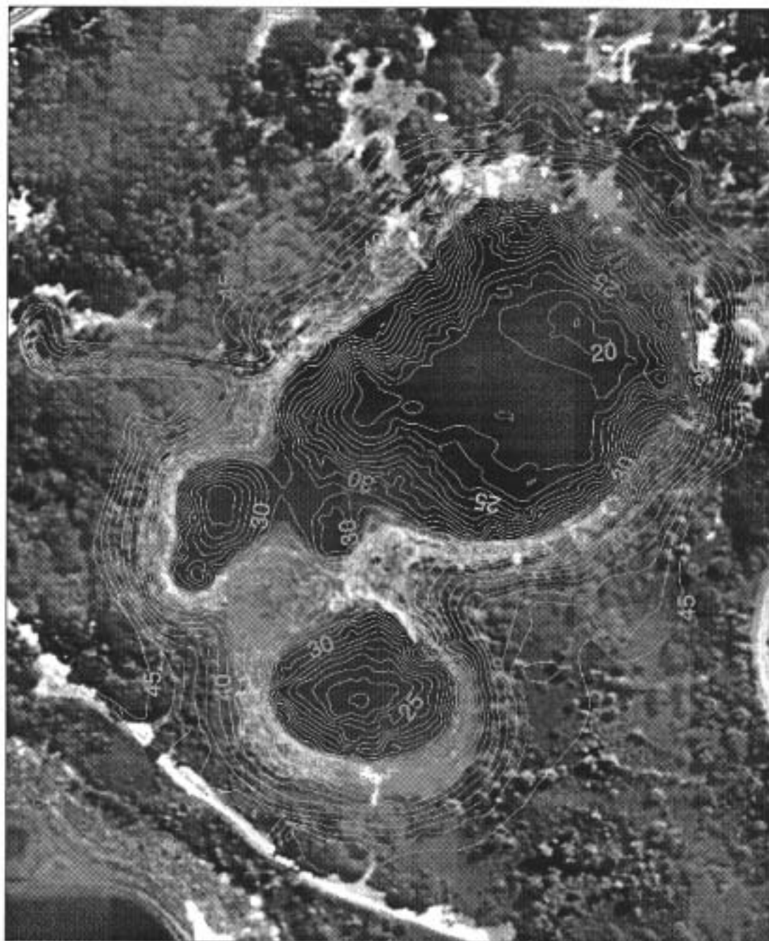
Figure 6-47. One-foot contour map of the Lake Raleigh basin, Hillsborough County, Florida. Values shown are elevations, in feet, above the National Geodetic Vertical Datum.
