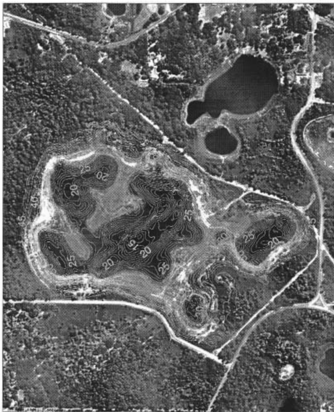
Figure 6-52. One-foot contour map of the Lake Rogers basin, Hillsborough County, Florida. Values shown are elevations, in feet, above the National Geodetic Vertical Datum.
