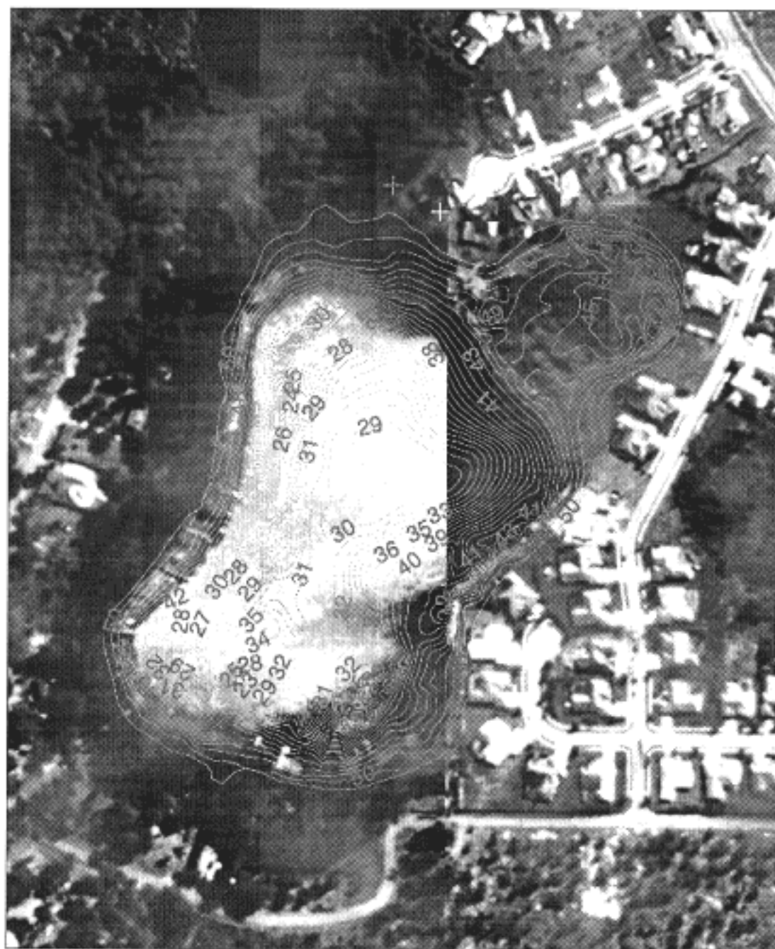
Figure 6-24. One-foot contour map of the Cypress Lake basin, Hillsborough County, Florida. Values shown are elevations, in feet, above the National Geodetic Vertical Datum.
