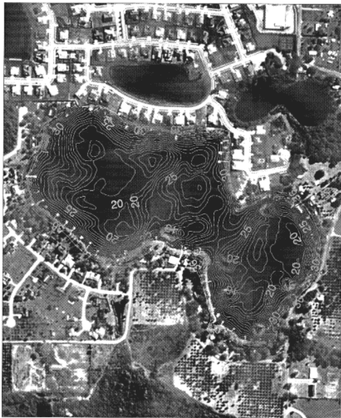
Figure 6-29. One-foot contour map of the Fairy Lake basin, Hillsborough County, Florida. Values shown are elevations, in feet, above the National Geodetic Vertical Datum.
