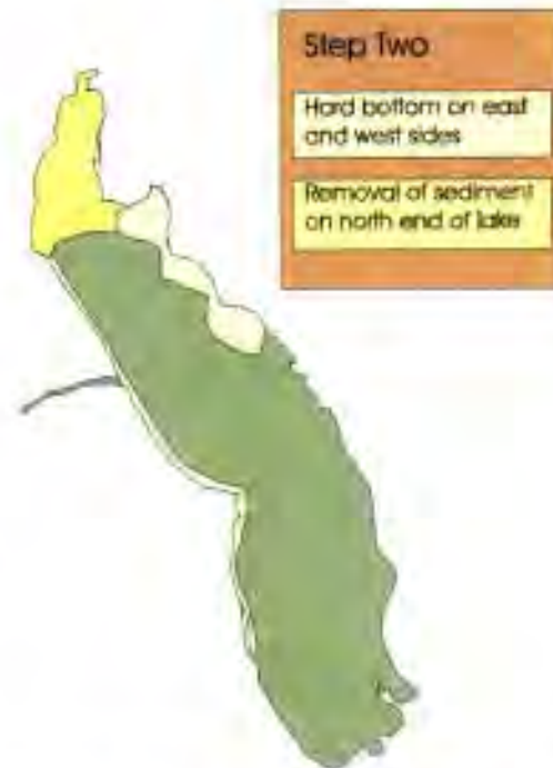
Figure 1. Step Two - Dredge to Hard Bottom from 35' Contour - entails dredging on east side of lake in vicinity of Shell and Geasey Points, along most of western shoreline. Although sediment deposits are deep, the north end is dredged to prevent material from this area being transported into hard bottom areas.
