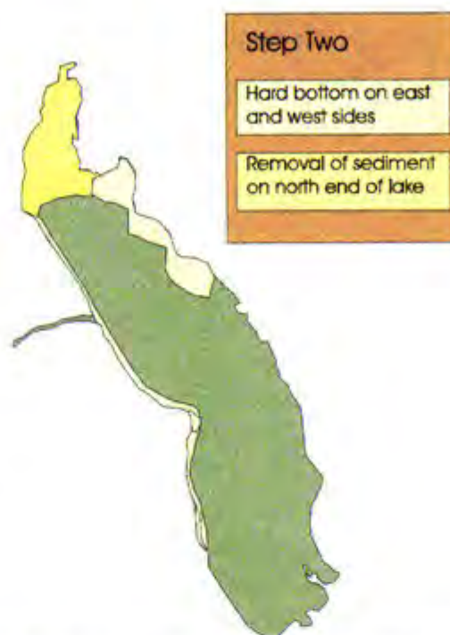
Figure 1. Step Two - Dredge to Hard Bottom from 35' Contour - entails dredging on east side of lake in vicinity of Shell and Grassy Points, along most of western shoreline. Although sediment deposits are deep, the north end is dredged to prevent material from this area being transported into hard bottom areas.
