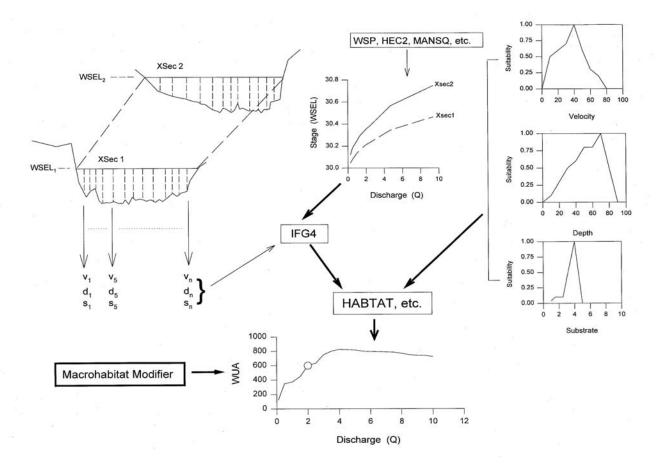
[Schematic of the PHABSIM model. The circle on the WUA/Discharge plot (above) represents the discharge at which 15% of habitat is lost]
