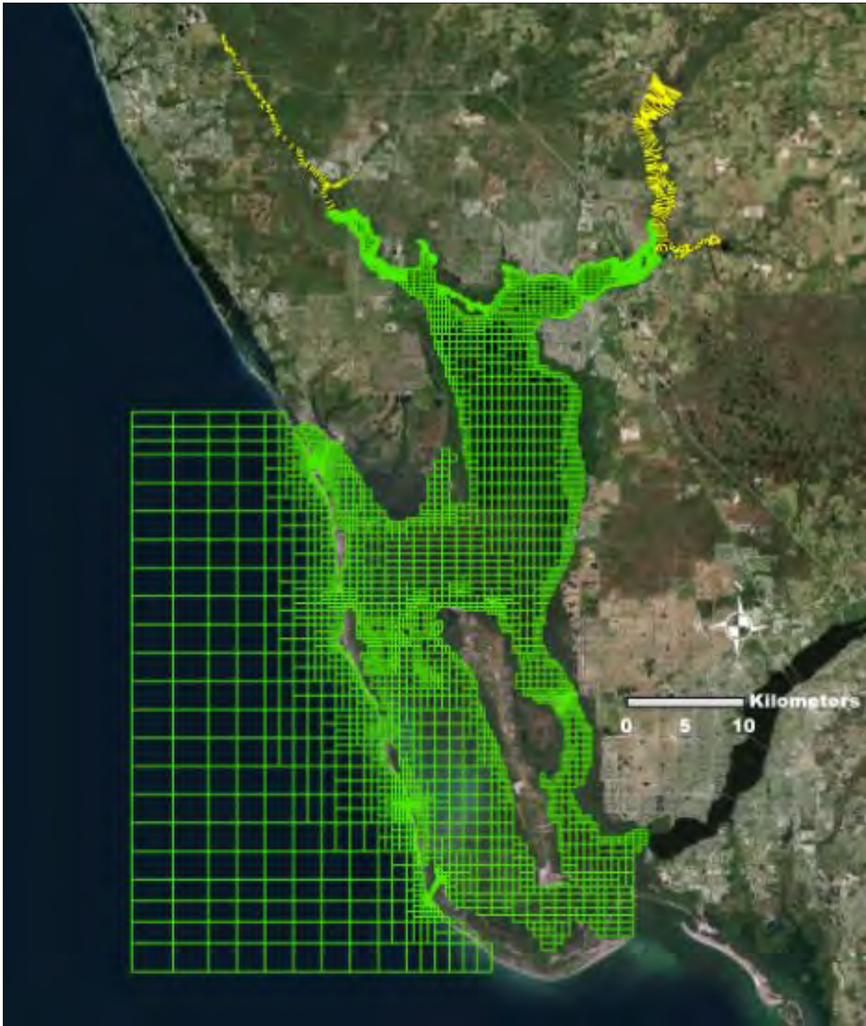
FIGURE 3. UnLESS model mesh used for greater Charlotte Harbor hydrodynamic modeling. Green rectangular tiles are model grids for the 3D simulation domain, while 2DV grids are bounded by cross sections drawn with yellow lines.
