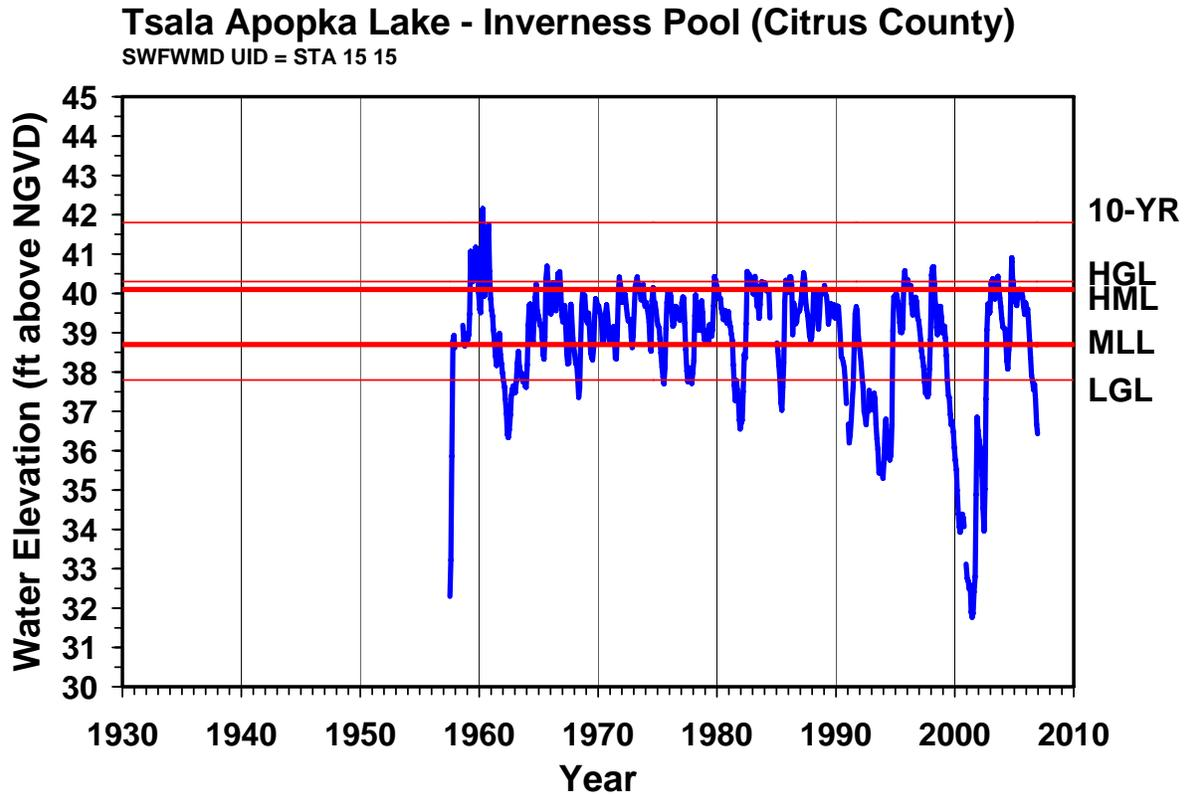
Figure 32. Mean monthly surface water elevation of the Hernando Pool of Tsala Apopka Lake through December 2006, and adopted Guidance and Minimum Levels. Levels include the Ten Year Flood Guidance Level (10-YR), High Guidance Level (HGL), High Minimum Lake Level (HMLL), and Minimum Lake Level (MLL).
