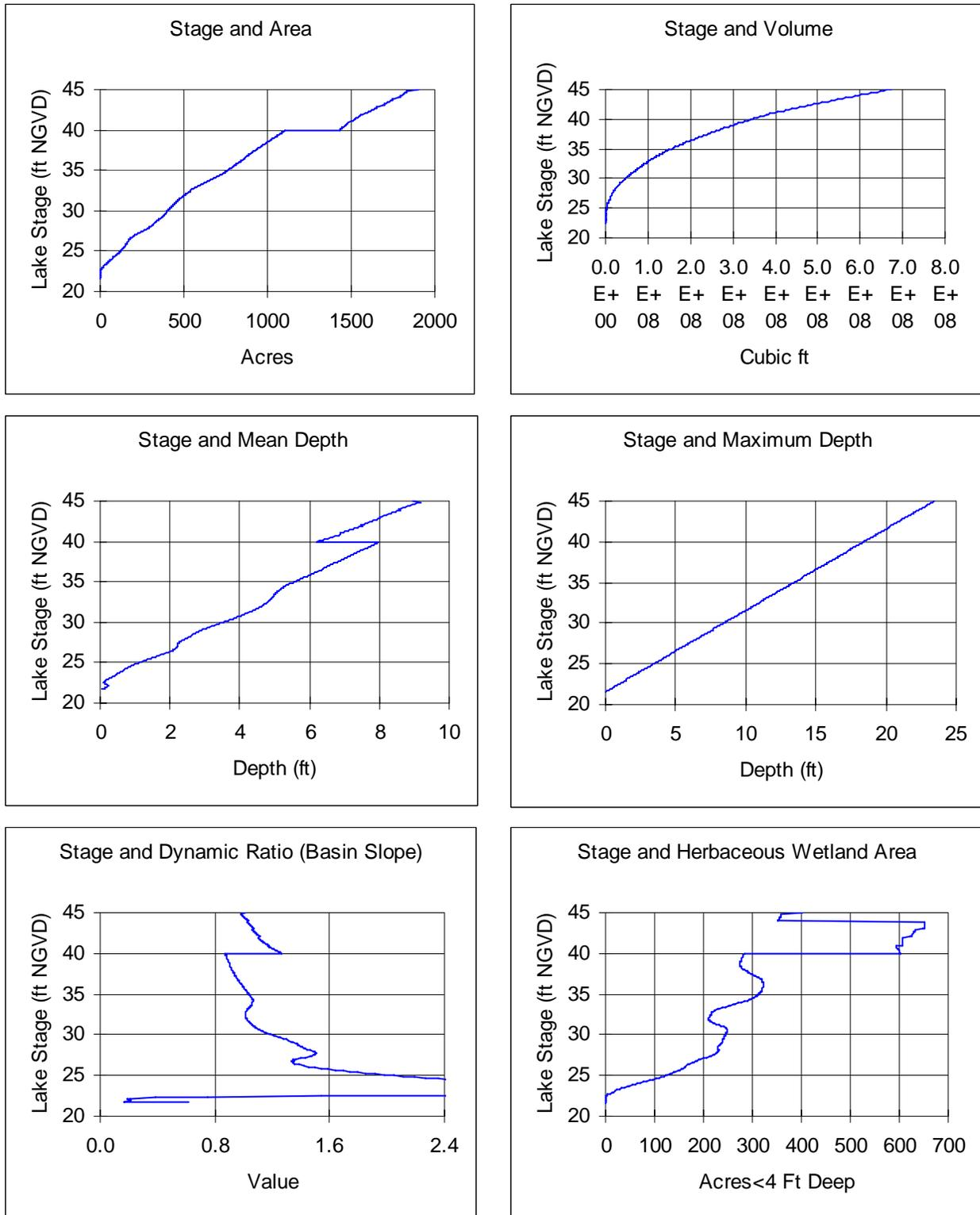
**Figure 26. Little Henderson Lake surface area, volume, mean depth, maximum depth, dynamic ratio (basin slope) and potential herbaceous wetland area versus lake stage.**
