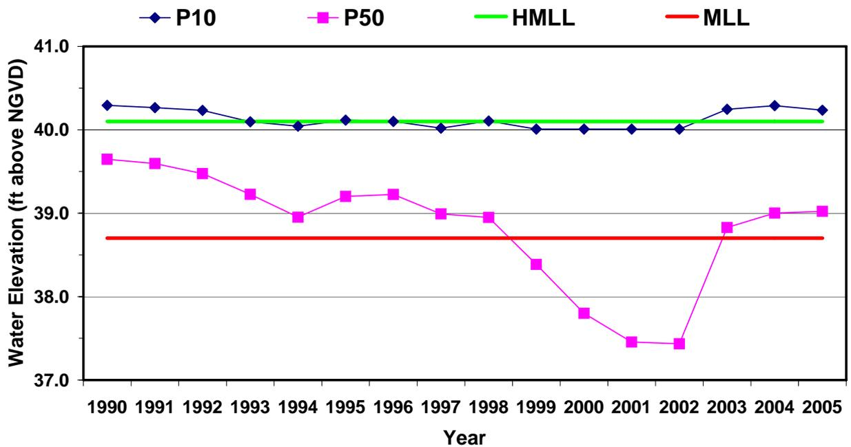
Figure 35. P10 and P50 values for the past sixteen ten-year periods in relation to the High Minimum Lake Level (HMLL) and Minimum Lake Level (MLL) for the Hernando Pool.
