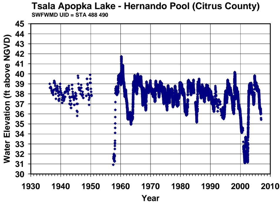
Figure 19. Monthly mean surface water elevations for the Hernando Pool of Tsala Apopka Lake for the Historic period from January 1946 through December 2005.
