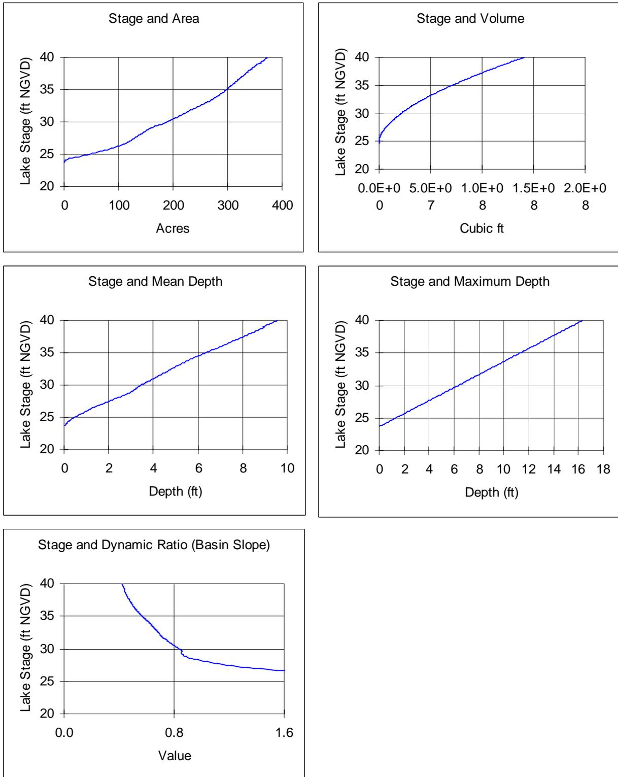
**Figure 28. Hernando Lake surface area, volume, mean depth, maximum depth, and dynamic ratio (basin slope) versus lake stage.**
