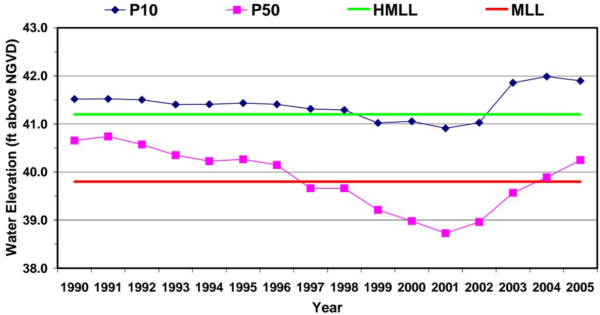
Figure 34. P10 and P50 values for the past sixteen ten-year periods in relation to the High Minimum Lake Level (HMLL) and Minimum Lake Level (MLL) for the Inverness Pool.
