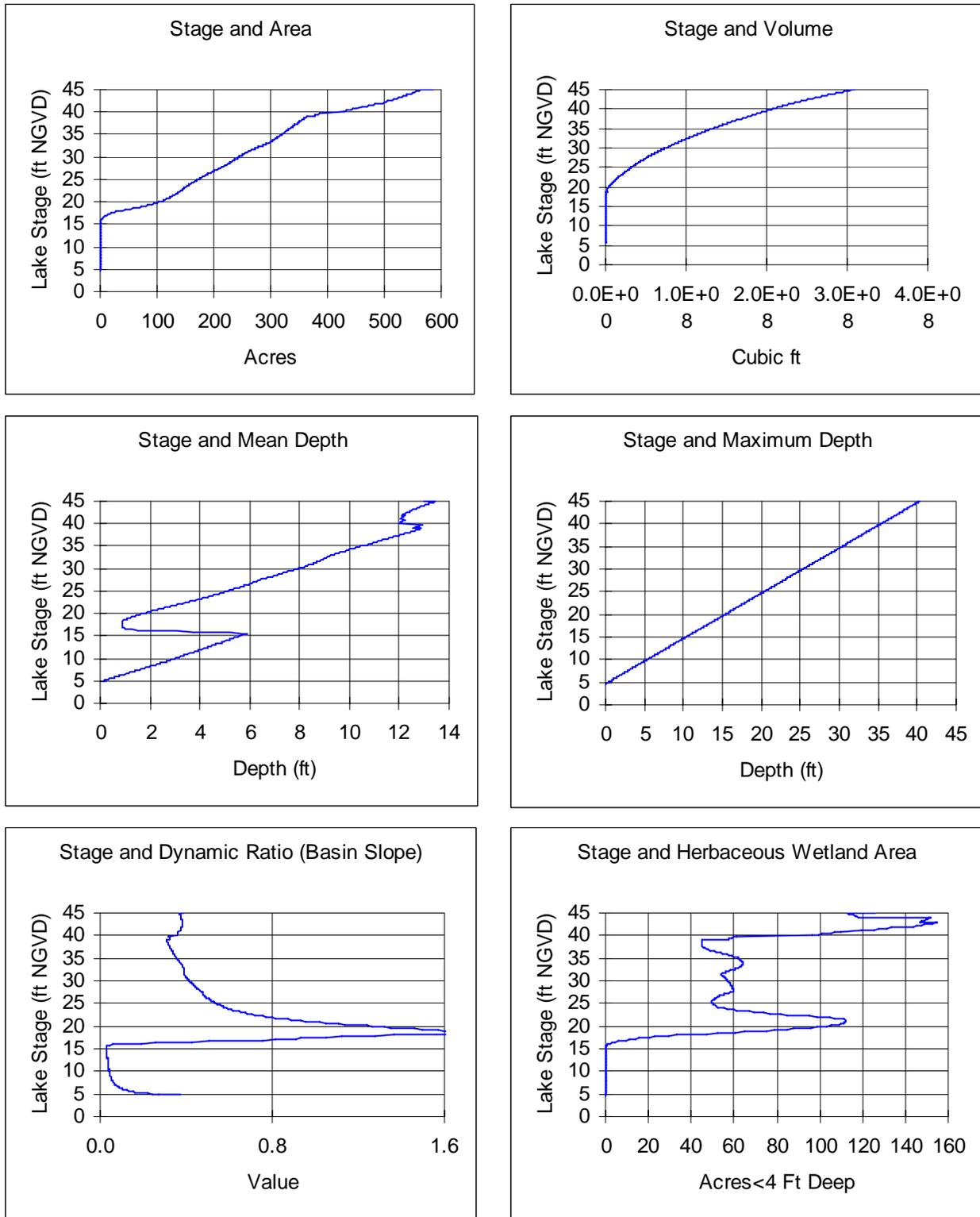
**Figure 27. Croft Lake surface area, volume, mean depth, maximum depth, and dynamic ratio (basin slope) versus lake stage.**
