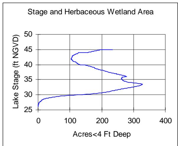
**Figure 23. Hampton Lake surface area, volume, mean depth, maximum depth, dynamic ratio (basin slope) and potential herbaceous wetland area versus lake stage.**
