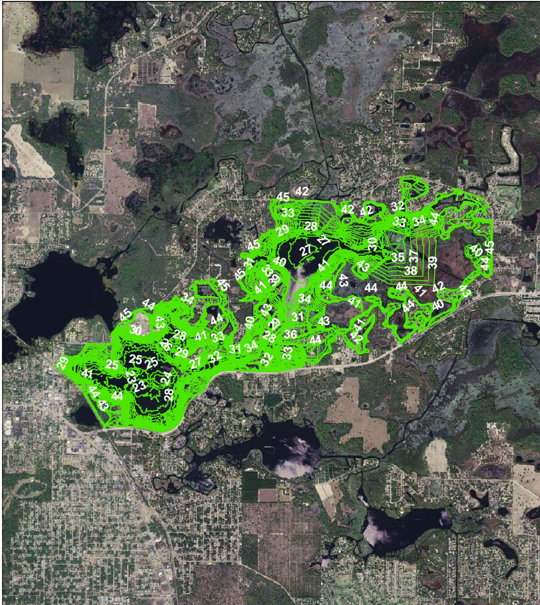
Map prepared using 2004 USGS true color digital orthophotography, elevation data from 1976 SWFWMD aerial photography with contours maps (Secs. 2, 3, 8 - 11, 15 - 17, Twp. 19 S, Rge. 20 E), and elevation data in 2004 collected by D.C. Johnson and Associates, Inc.
