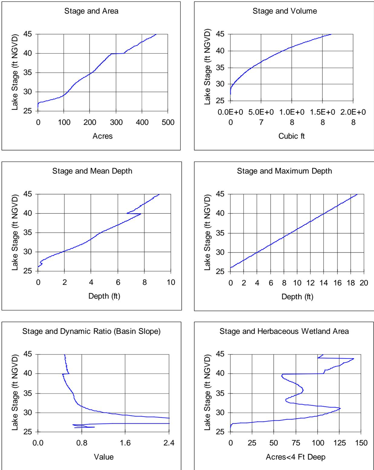
**Figure 25. Henderson Lake surface area, volume, mean depth, maximum depth, dynamic ratio (basin slope) and potential herbaceous wetland area versus lake stage.**
