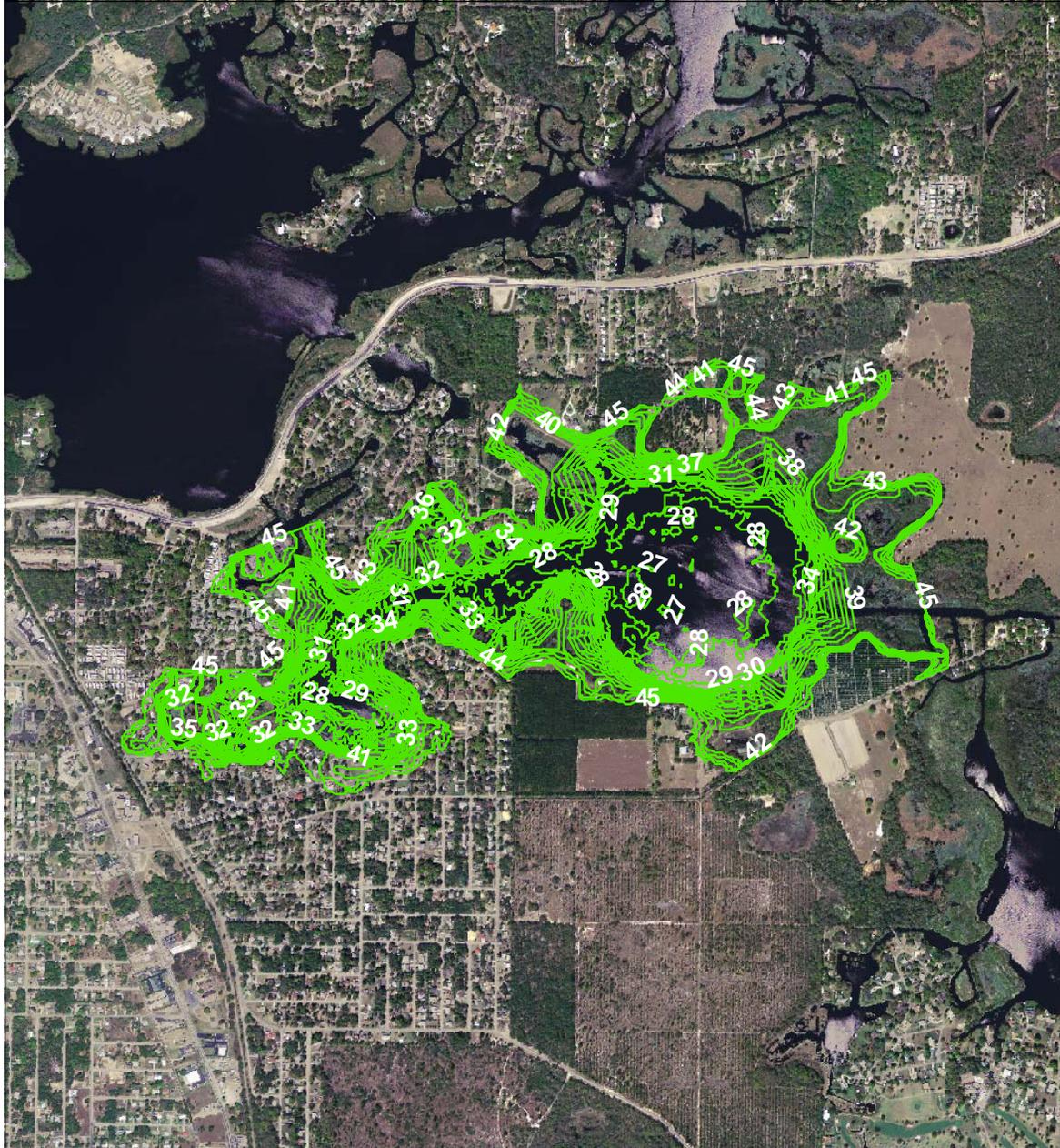
Map prepared using 2004 USGS true color digital orthophotography, elevation data from 1976 SWFWMD aerial photography with contours maps (Secs. 15, 16, 21, 22, Twp. 19 S, Rge. 20 E), and elevation data collected 2004 by D.C. Johnson and Associates, Inc.
