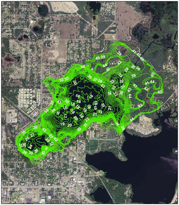
Map prepared using 2004 USGS true color digital orthophotography, elevation data from 1973 and 1976 SWFWMD aerial photography with contours maps (Secs. 7 - 9, 17, and 18, Twp. 19 S, Rge. 20 E), and elevation data collected in 2004 by D.C. Johnson and Associates, Inc.
