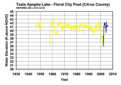
Figure 21. Composite monthly mean surface water elevations for the Inverness Pool of Tsala Apopka Lake for the Historic period from January 1946 through December 2005. Composite data include values based on measured water surface elevations (blue) and modeled values (yellow).
