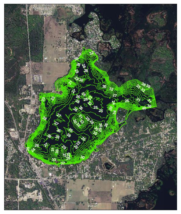
Map prepared using 2004 USGS true color digital orthophotography, elevation data from 1973 SWFWMD aerial photography with contours maps (Secs. 13, 23 - 26, Twp. 18 S, Rge. 19 E), and elevation data collected in 2004 by D.C. Johnson and Associates, Inc.
