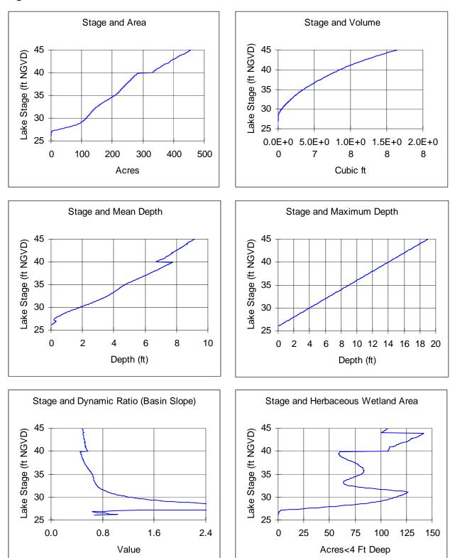
Figure 24. Spivey Lake surface area, volume, mean depth, maximum depth, dynamic ratio (basin slope) and potential herbaceous wetland area versus lake stage.
