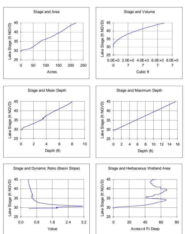
Figure 23. Hampton Lake surface area, volume, mean depth, maximum depth, dynamic ratio (basin slope) and potential herbaceous wetland area versus lake stage.
