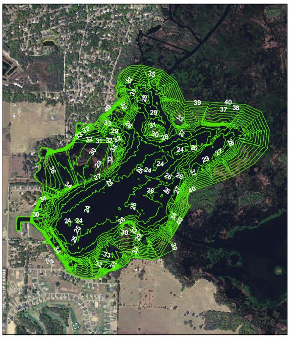
Map prepared using 2004 USGS true color digital orthophotography, elevation data from 1973 SWFWMD aerial photography with contours maps (Secs. 25, and 36, Twp. 18 S, Rge. 19 E, and Sec. 30, Twp. 18 S, Rge 20 E), and elevation data collected in 2004 by D.C. Johnson and Associates, Inc.
