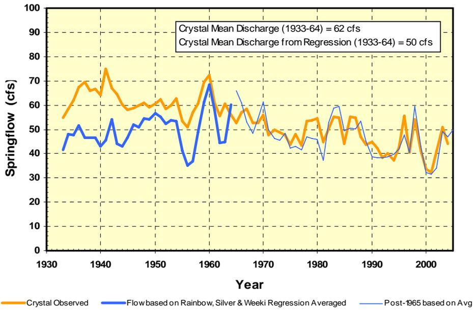
Figure 2. Synthetic Crystal Springs discharge prior to 1965 using the average of three regressions with Weeki Wachee, Rainbow, and Silver Springs from 1965 through 2004.
