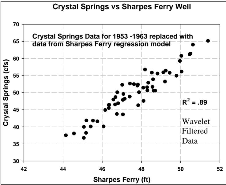
Figure 2-57. Crystal Springs data for 1953 to 1963 adjusted with data from Sharpes Ferry regression model.
