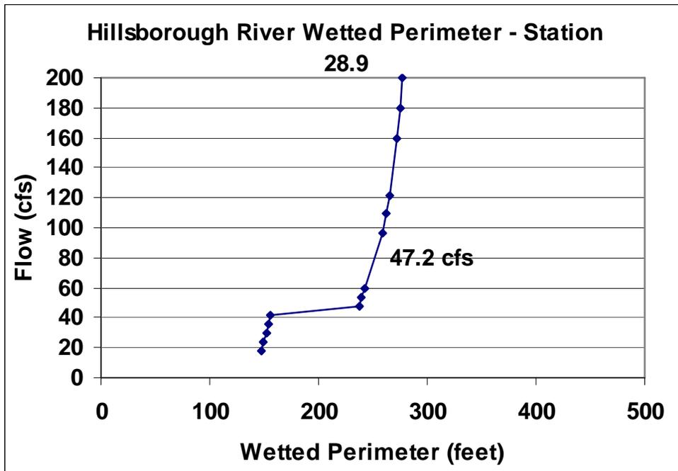
Figure 4-7. Wetted perimeter versus discharge at HEC-RAS transect number 28.9 in the Hillsborough River corridor. Wetted perimeter values for modeled flows up to 200 cfs are shown and the Lowest Wetted Perimeter Inflection Point (LWPIP) is identified.
