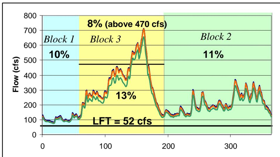
Figure 5-13. Median daily flow plotted for each day of the southern river pattern water year with short-term compliance standards for Blocks 1, 2, and 3. The blue line is the calculated natural flow corrected for withdrawals. The green line represents the natural flow reduced by the maximum allowable. The orange line is the current median calculated from the period of record at the Morris Bridge gage site.
