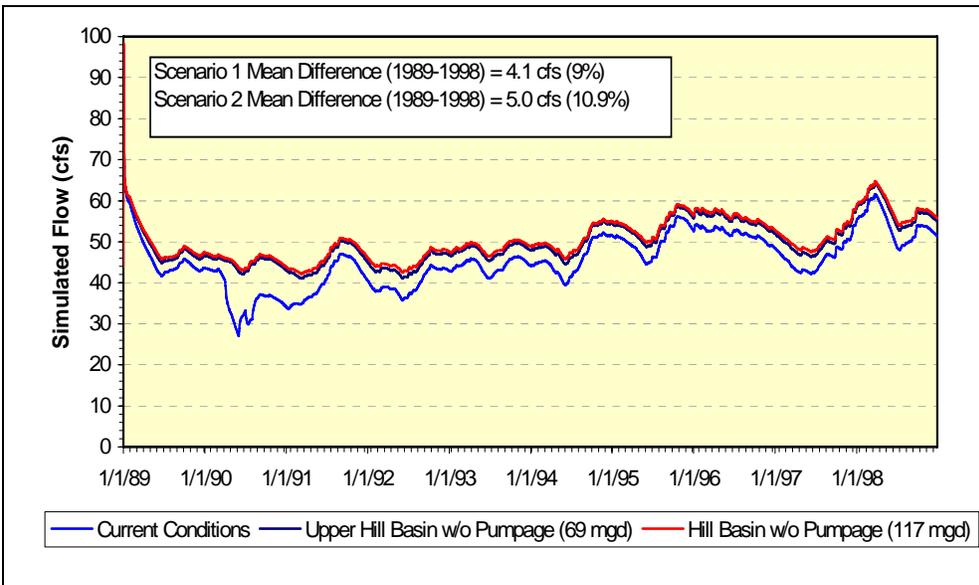
**Figure 2-66. Impacts to Crystal Springs due to 69 mgd and 117 mgd of groundwater withdrawals within the Hillsborough River watershed.**
