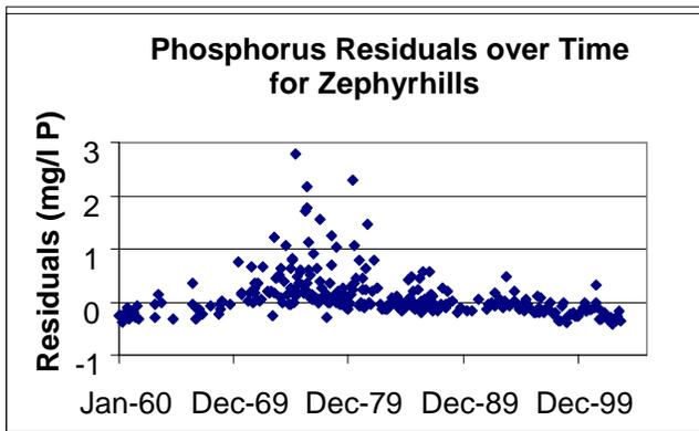
Figure 2-71. Phosphorus concentrations in water samples collected by the USGS at the Hillsborough River near Zephyrhills gage. Upper plot is time series plot; middle plot is concentration versus flow; and the bottom plot is time series plot of residuals of phosphorus concentration regressed against flow.
