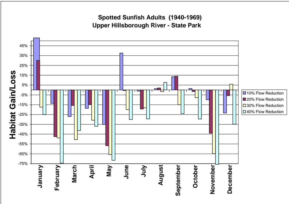
Figure 4-4. Example plot of habitat gain/loss relative to flow reductions of 10, 20, 30, and 40 %. Habitat loss is shown for spotted sunfish adults in the Hillsborough River State Park based on historic flow records from 1940 to 1969.
