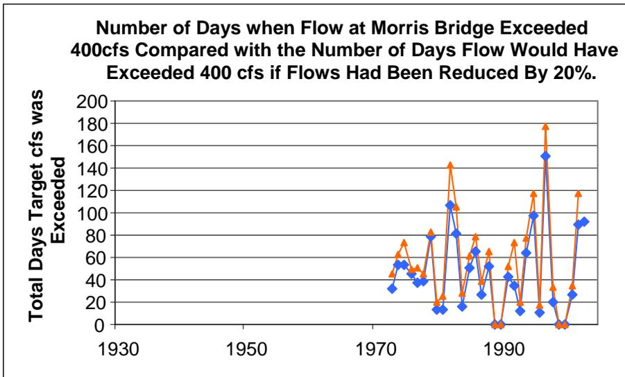
Figure 4-6. RALPH plot of the number of days during the southern river pattern water year that 400 cfs is exceeded at the USGS Hillsborough River near Morris Bridge gage site (orange line) compared with the number of days that inundation would have occurred if there had been a 20% reduction in river flows (blue line).
