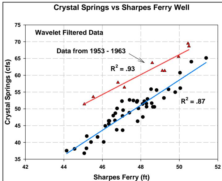
Figure 2-53. Crystal Springs Flow versus Groundwater Elevation
