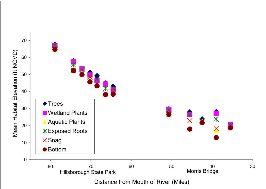
**Figure 5-12. Mean instream habitat elevations at twelve cross-section sites on the Upper Hillsborough River. Instream modeling through HEC-RAS, however, was confined to 9 transects (between Transects 3 and 13 only).**
