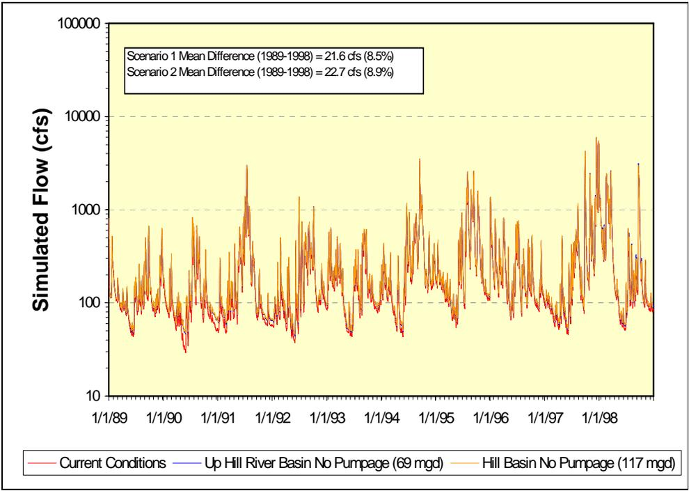
**Figure 2-67. Impacts to Hillsborough River stream flow at the Zephyrhills station due to 69 mgd and 117 mgd of groundwater withdrawals within the Hillsborough River watershed.**
