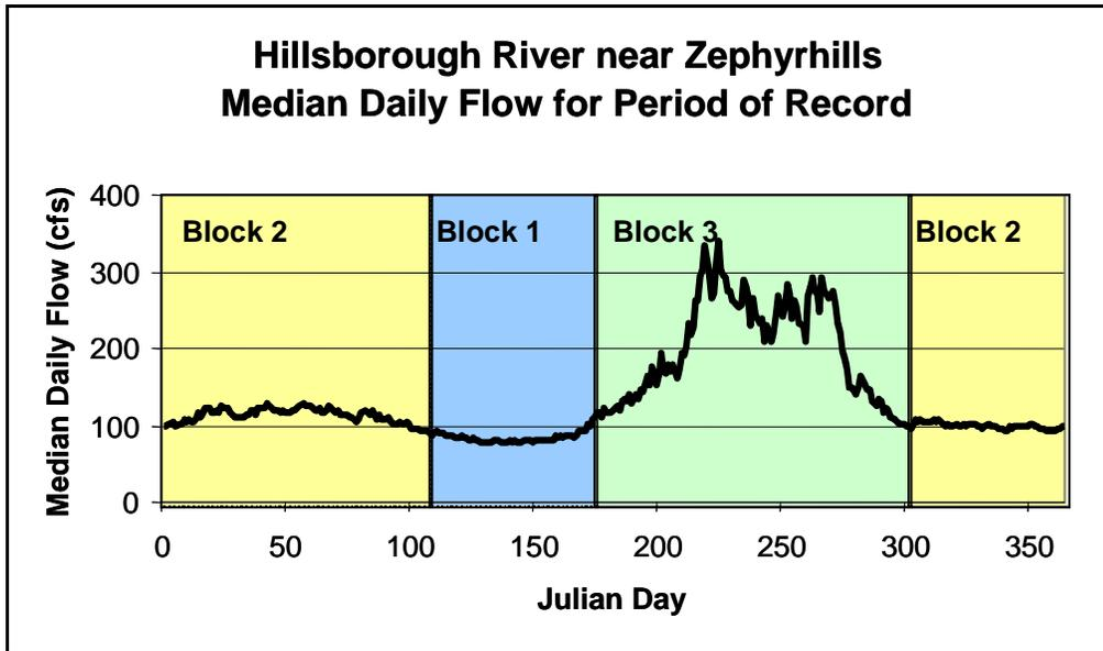
Figure 1-1. Median daily flows for the USGS Hillsborough River near Zephyrhills, FL gage site and seasonal flow blocks (Blocks 1, 2 and 3) for the upper Hillsborough River.
