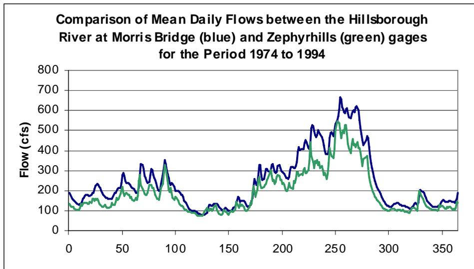
Figure 2-20. Comparison of Mean Daily Flows between the Hillsborough River at Morris Bridge gage with the Zephyrhills gage for the period 1974 to 1994.
