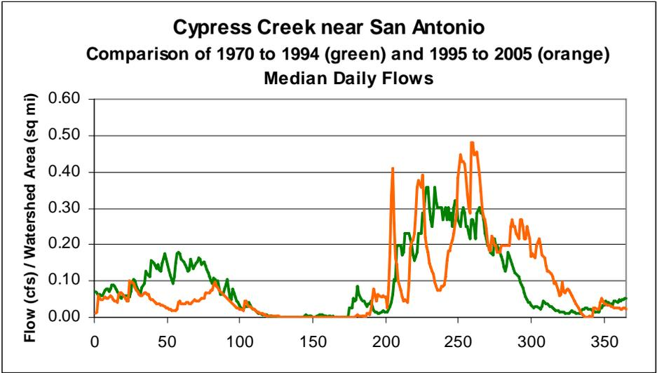
**Figure 2-27. Comparison of mean and median daily flows for two time periods – 1970 to 1994 (green) and 1995 to 2005 (orange) for the Cypress Creek near San Antonio gage site.**
