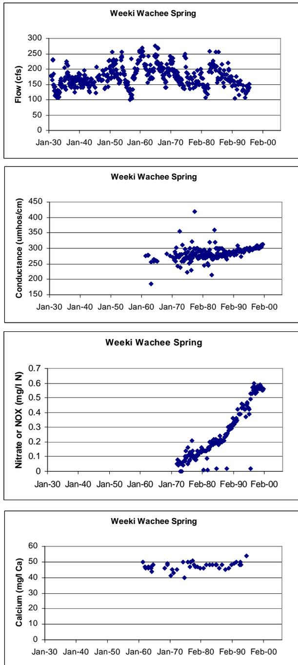
Figure 2-86. Time series plots of flow and selected water quality parameters at Weeki Wachee Springs.
