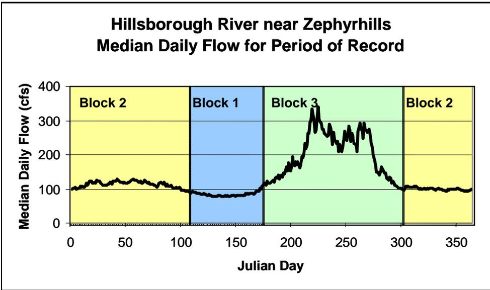
Figure 2-31. Median daily flows for 1937 through 2003 at the USGS Hillsborough River near Zephyrhills, FL Gage site and seasonal flow blocks (Blocks 1, 2 and 3) for the upper Hillsborough River.
