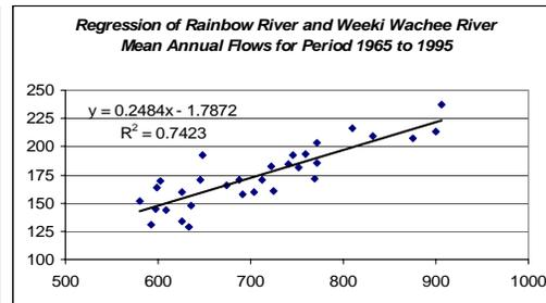
**Figure 2-39. Simple regression analysis of mean annual flow for period 1965 to 1995 between various spring systems: Crystal Springs, Silver River, Rainbow River and Weeki Wachee River.**
