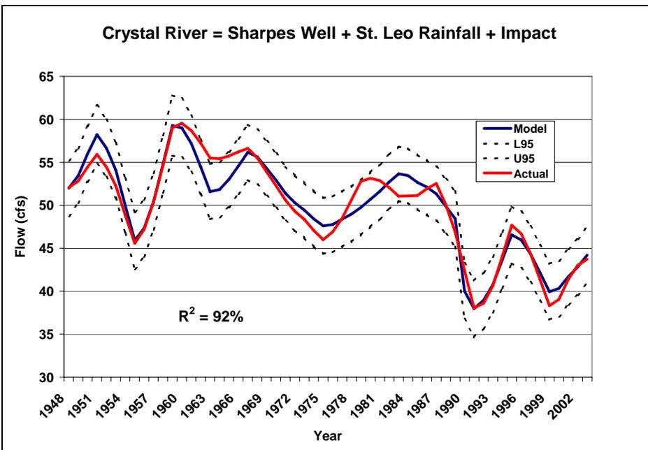
Figure 2-60. Multiple regression model for Crystal Springs Flow using wavelet filtered data.
