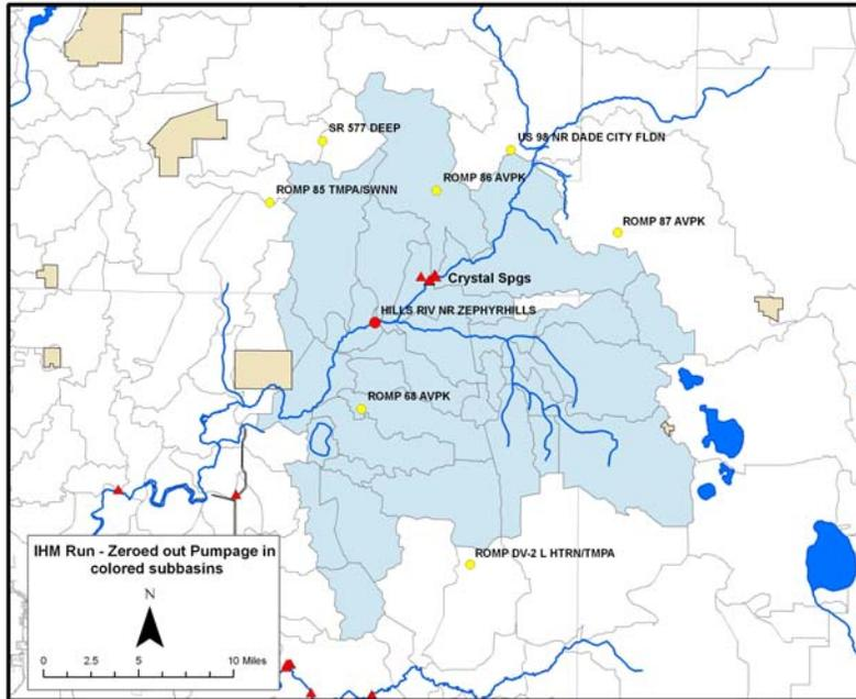
**Figure 2-64. INTBM scenario 1 where impacts to the hydrologic system were simulated due to groundwater withdrawals of 69 mgd (1989-1998 average) in the shaded area.**
