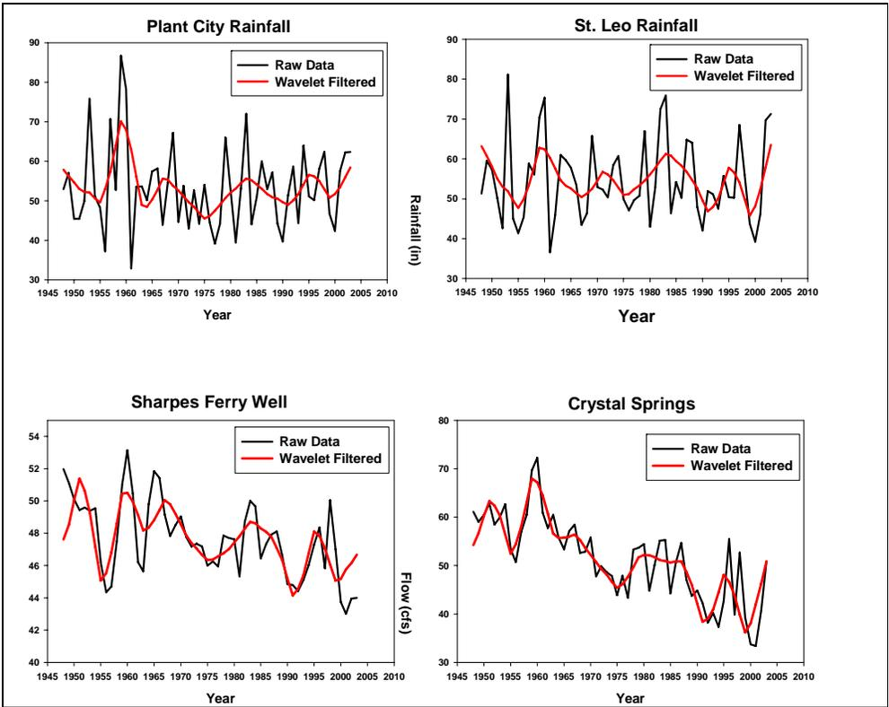
**Figure 2-51. Filtered Wavelet Data, where the noise from crystals d1 and d2 have been removed, versus Original Raw Data.**
