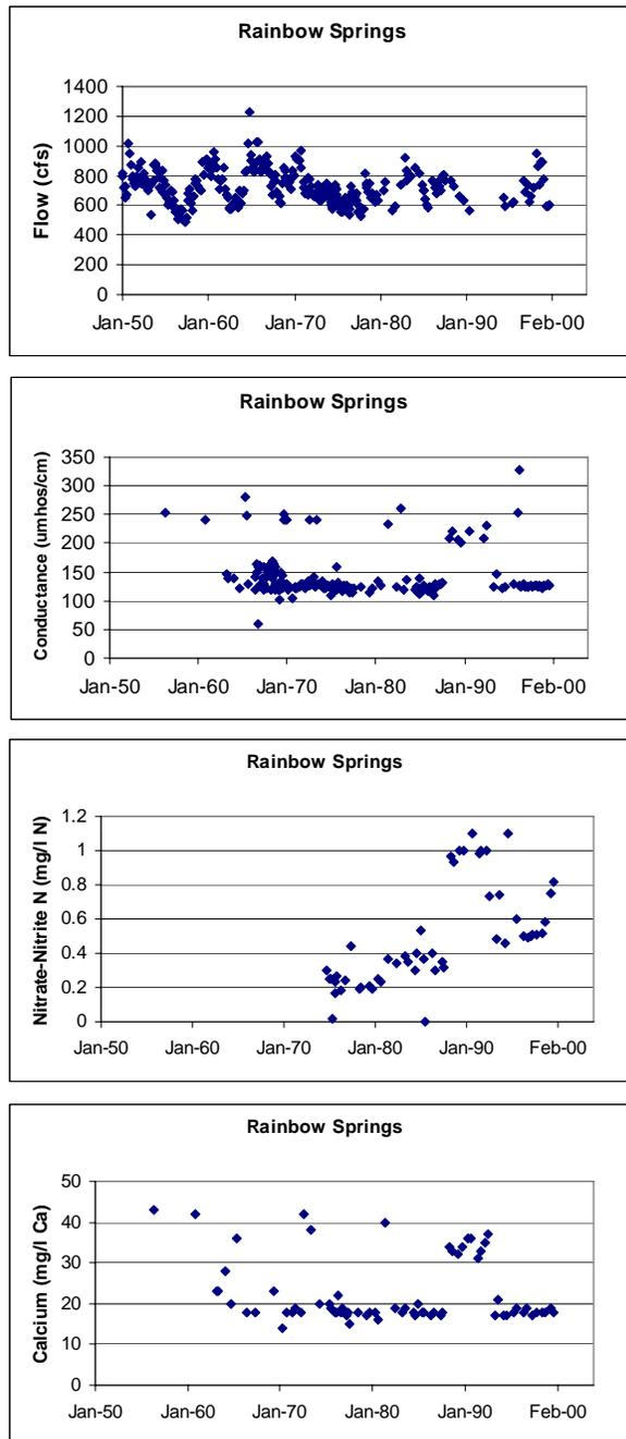
Figure 2-83. Time series plot ss of flow and selected water quality parameters at Rainbow Spring.
