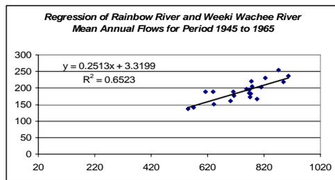
Figure 2-37. Simple regression analysis of mean annual flow for period 1945 to 1965 between various spring systems: Crystal Springs, Silver River, Rainbow River and Weeki Wachee River.
