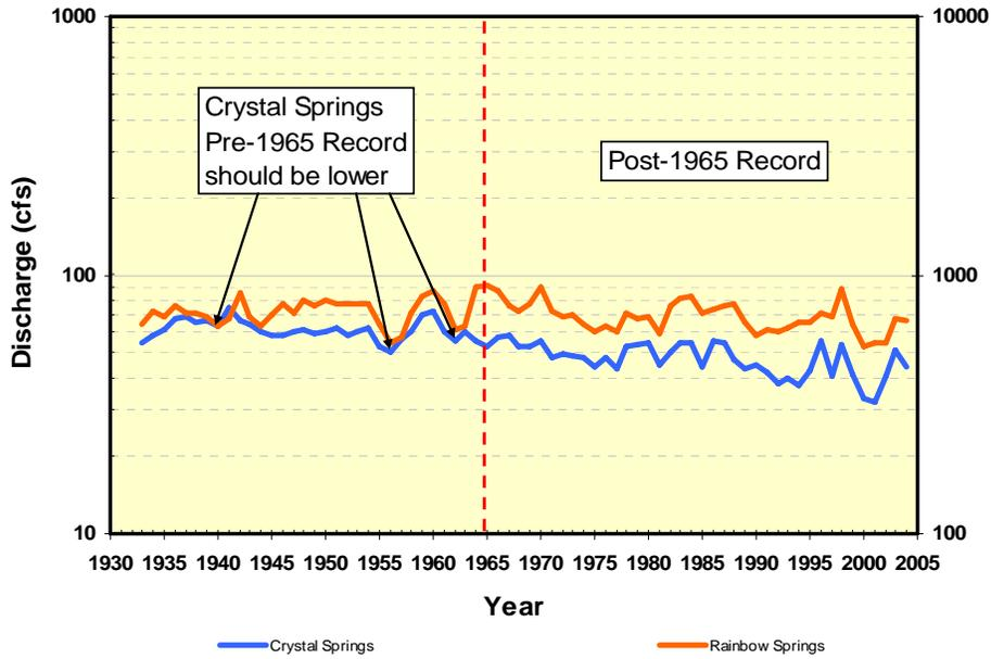
Figure 1. Mean annual discharge of Crystal Springs and Rainbow Springs (1933-2004).
