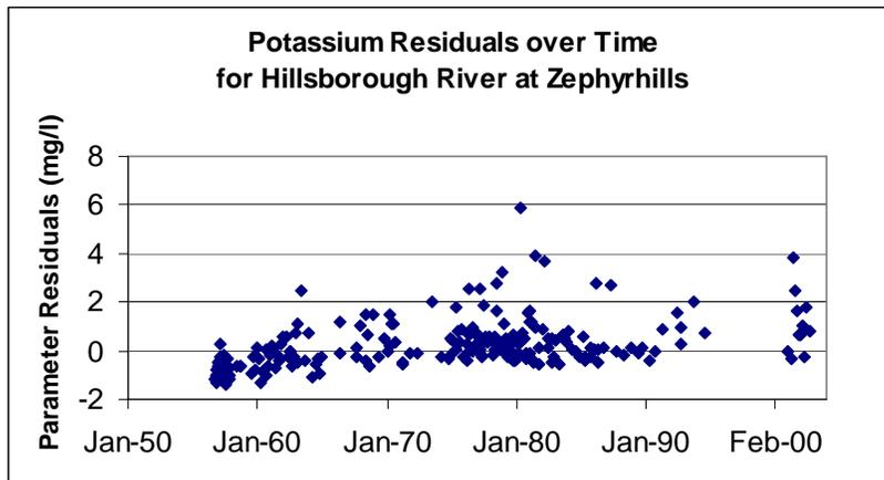
Figure 2-74. Potassium concentrations in water samples collected by the USGS at the Hillsborough River near Zephyrhills gage. Upper plot is time series plot; middle plot is concentration versus flow; and the bottom plot is time series plot of residuals of potassium concentration regressed against flow.
