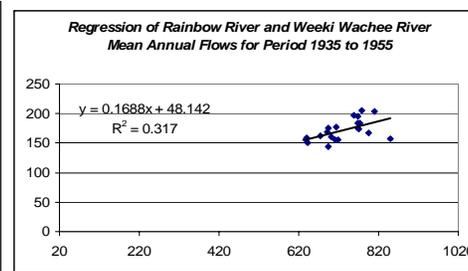
**Figure 2-36. Simple regression analysis of mean annual flow for period 1935 to 1955 between various spring systems: Crystal Springs, Silver River, Rainbow River and Weeki Wachee River.**
