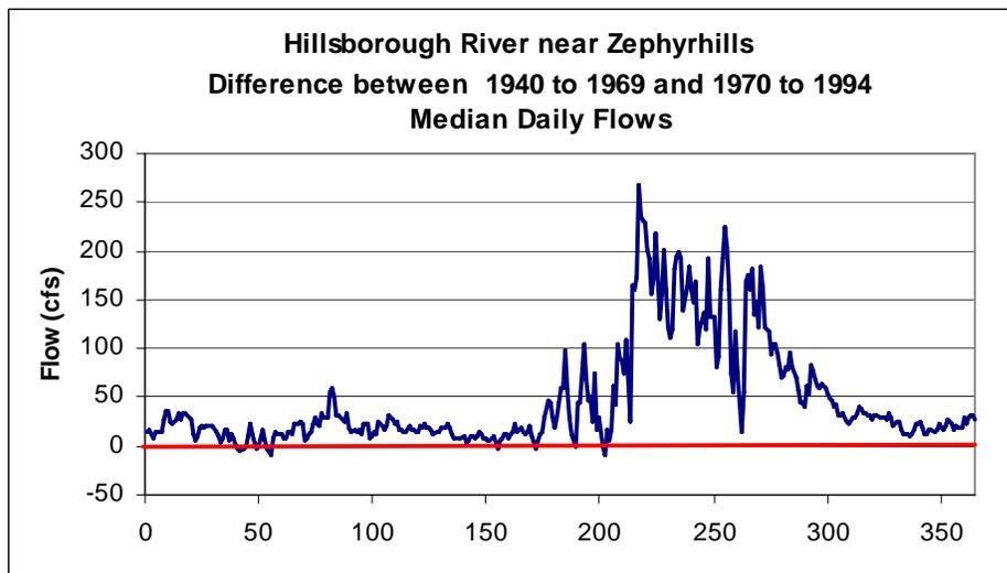
Figure 2-24. Comparison of median daily flows for the Hillsborough River near Zephyrhills for two time periods (1940 to 1969 and 1970 to 1994).
