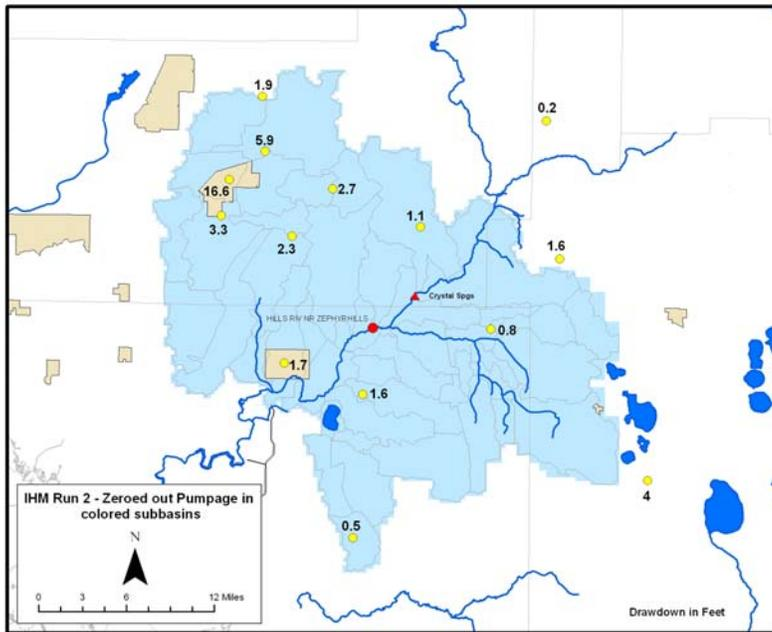
Figure 2-68. Predicted decline in the Upper Floridan aquifer at selected locations due to 117 mgd of groundwater withdrawals within the Hillsborough River watershed.
