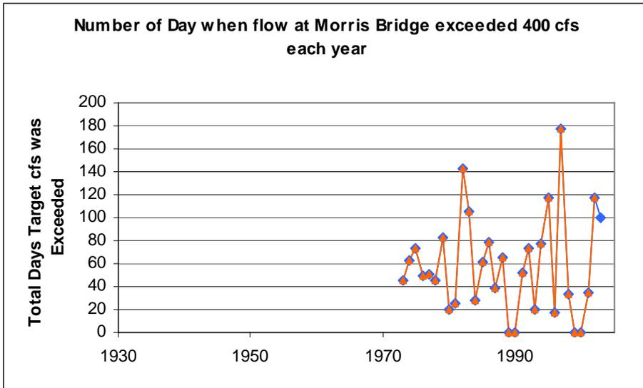
Figure 4-5. RALPH plot of the number of days during the southern river pattern (SRP) water year that 400 cfs is exceeded at the USGS Hillsborough River near Morris Bridge gage site.
