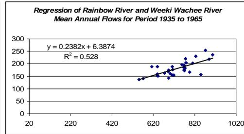
Figure 2-38. Simple regression analysis of mean annual flow for period 1935 to 1965 between various spring systems: Crystal Springs, Silver River, Rainbow River and Weeki Wachee River.
