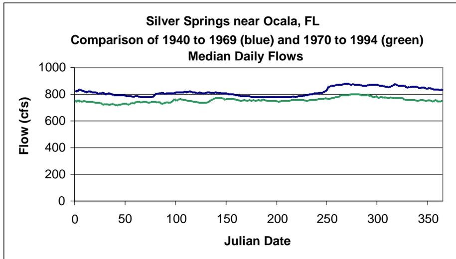
Figure 2-70. Plot comparing median daily flows for two AMO periods; the average difference in mean and median daily flows between the two periods amounted to 8.7 and 7.6%, respectively.
