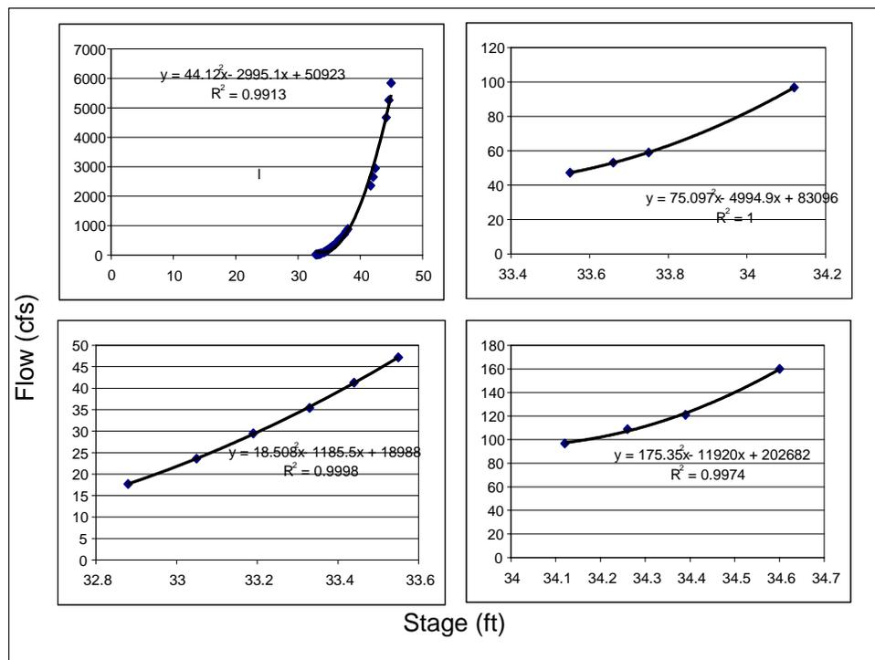
**Figure 4-8. Stage flow relationships between HEC-RAS cross-section 40.4 and flow at the USGS Morris Bridge gage derived from the HEC-RAS model of the Hillsborough River. The upper-left plot shows the relationship derived for the entire range of flows evaluated. The other three show relationships used to develop regression equations for selected portions of the flow range.**
