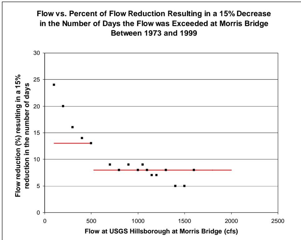
Figure 5-8. Percent-of-flow reductions that result in a 15% reduction in the number of days flows at the USGS Upper Hillsborough River near the Morris Bridge gage are achieved, based on flow records from 1973 through 1999.
