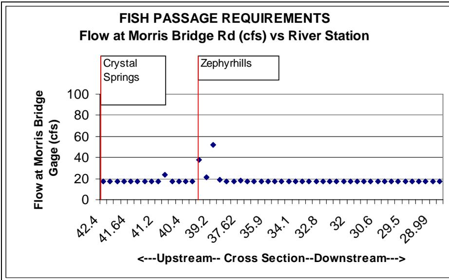
Figure 5-1. Plot of flow required at the Hillsborough River at Morris Bridge gage to inundate the deepest part of the channel at each HEC-RAS cross-section in the Hillsborough River to a depth of 0.6 ft.
