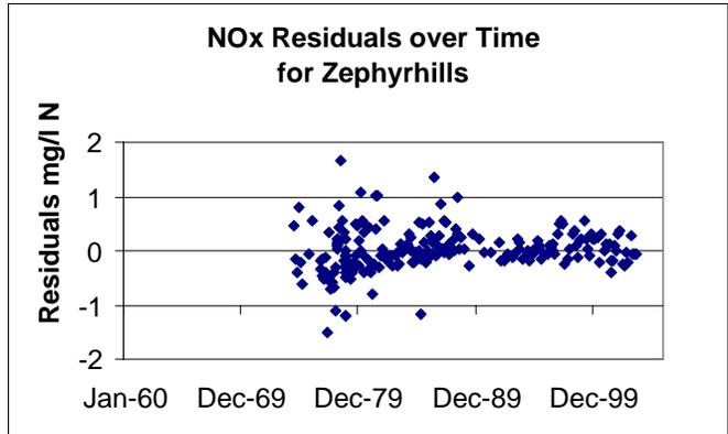
Figure 2-72. Nitrate or nitrate/nitrite concentrations in water samples collected by the USGS at the Hillsborough River near Zephyrhills gage. Upper plot is time series plot; middle plot is concentration versus flow; and the bottom plot is time series plot of residuals of nitrate/nitrite concentration regressed against flow.
