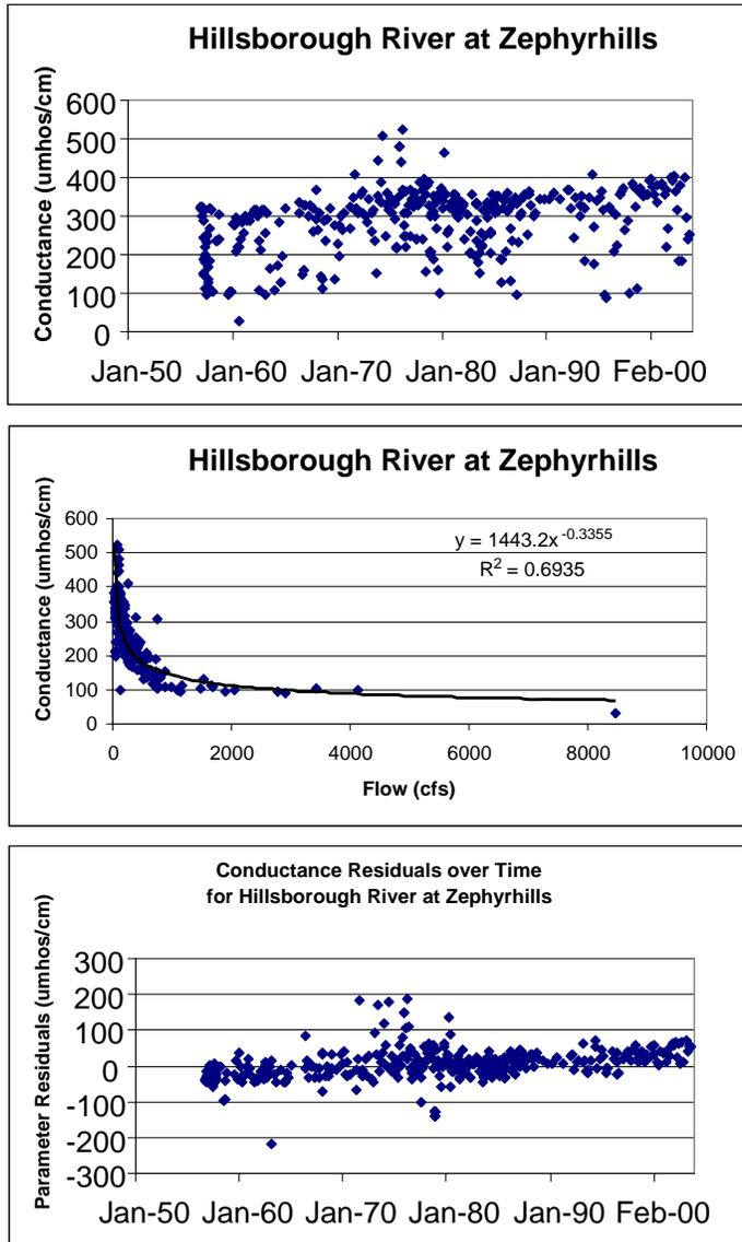
Figure 2-75. Conductance in water samples collected by the USGS at the Hillsborough River near Zephyrhills gage. Upper plot is time series plot; middle plot is conductance versus flow; and the bottom plot is time series plot of residuals of conductance regressed against flow.
