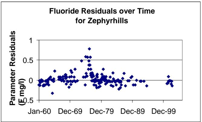
Figure 2-76. Fluoride concentrations in water samples collected by the USGS at the Hillsborough River near Zephyrhills gage. Upper plot is time series plot; middle plot is concentration versus flow; and the bottom plot is time series plot of residuals of fluoride concentrations regressed against flow.
