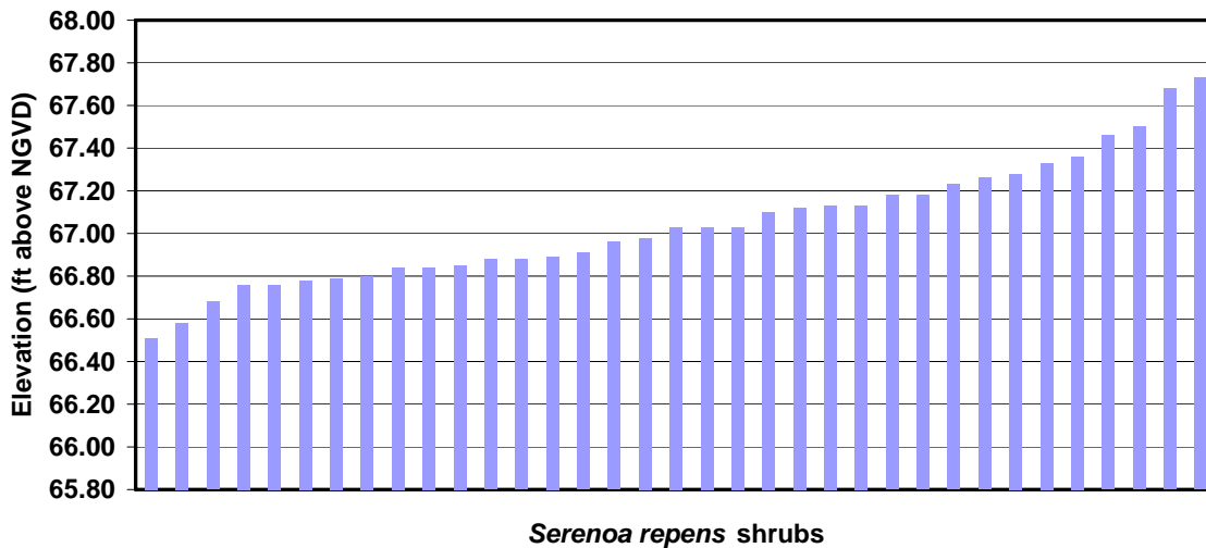
Figure 19. Ground elevations at the base of Serenoa repens shrubs used to establish the Normal Pool elevation for Pasco Lake.
