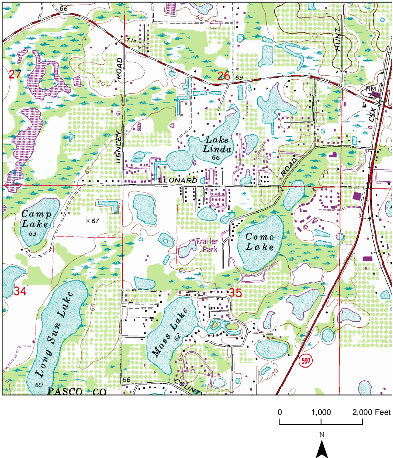
Figure 17. Five-foot elevation contours in the vicinity of Lake Linda. Note that the lake water surface is listed at 66 feet above NGVD 1929 (image source: Southwest Florida Water Management District 2002b).
