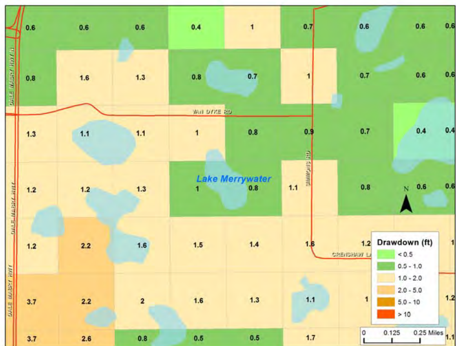
Figure 7. Predicted mean drawdown in the surficial aquifer due to TBW 90 mgd groundwater withdrawals.
