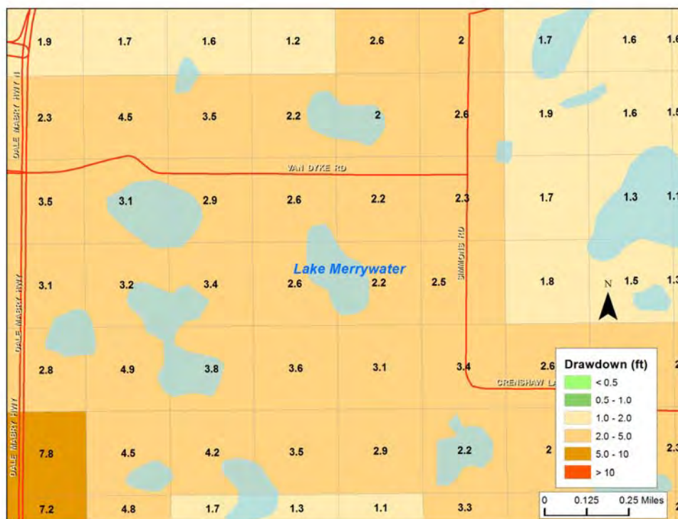
Figure 5. Predicted mean drawdown in the surficial aquifer due to 1989-2000 groundwater withdrawals.
