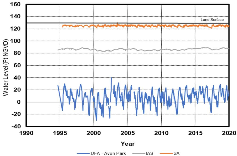
Figure 2-20. Water levels (in ft) from monitor wells installed into the surficial, intermediate, and Upper Floridan aquifers at the District Regional Observation and Monitor-Well Program 39 site. Note 1 ft = 0.3 m.
