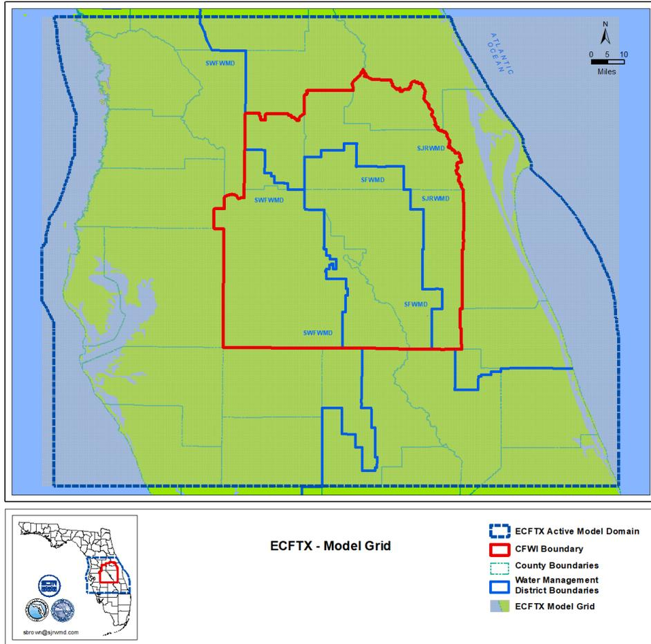
**Figure 2-28. Model grid for the East Central Florida Transient Expanded (ECFTX) model domain.**
