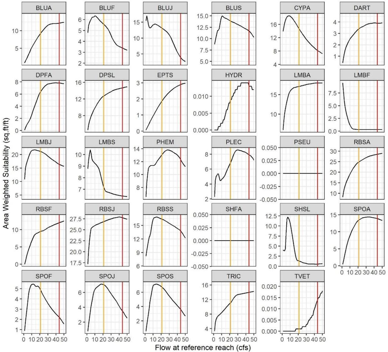
**Figure 5-10. Reach Habitat Curves for 7 Upper Little Manatee River sites combined. Note that block boundary flows are shown for the downstream USGS Little Manatee River at US 301 near Wimauma, FL (No. 02300500) gage, but were scaled proportionally for each reach to account for upstream flow diminution.**
