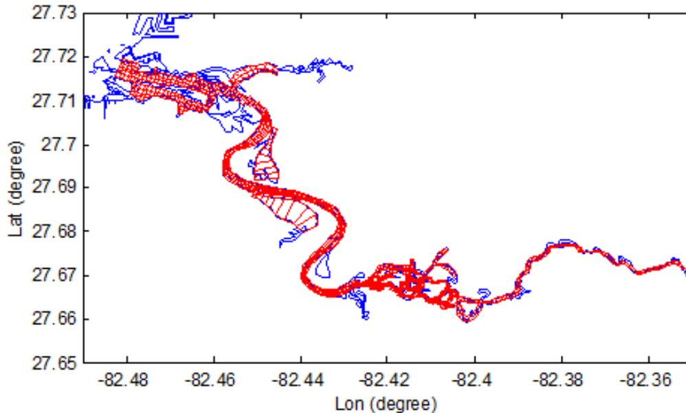
**Figure 5-11. The orthogonal grid system (horizontal view) used by the EFDC model for the Lower Little Manatee River estuary.**
