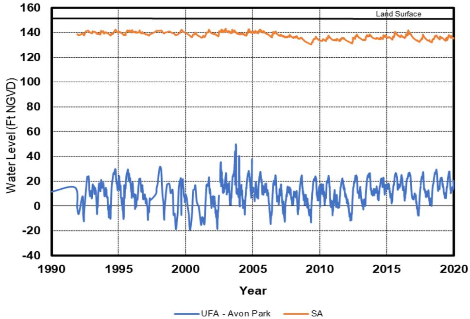
Figure 2-21. Water levels (in ft) from monitor wells installed into the surficial and Upper Floridan aquifers at the District Regional Observation and Monitor-Well Program 49 site. Note 1 ft = 0.3 m.
