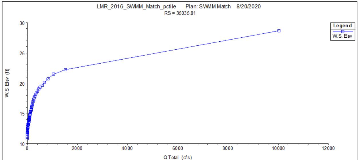
**Figure 5-6. Example rating curve for the Upper Little Manatee River at Cross Section 35035.81 (W.S. Elev = water surface elevation, Q Total = flow rate or discharge).**
