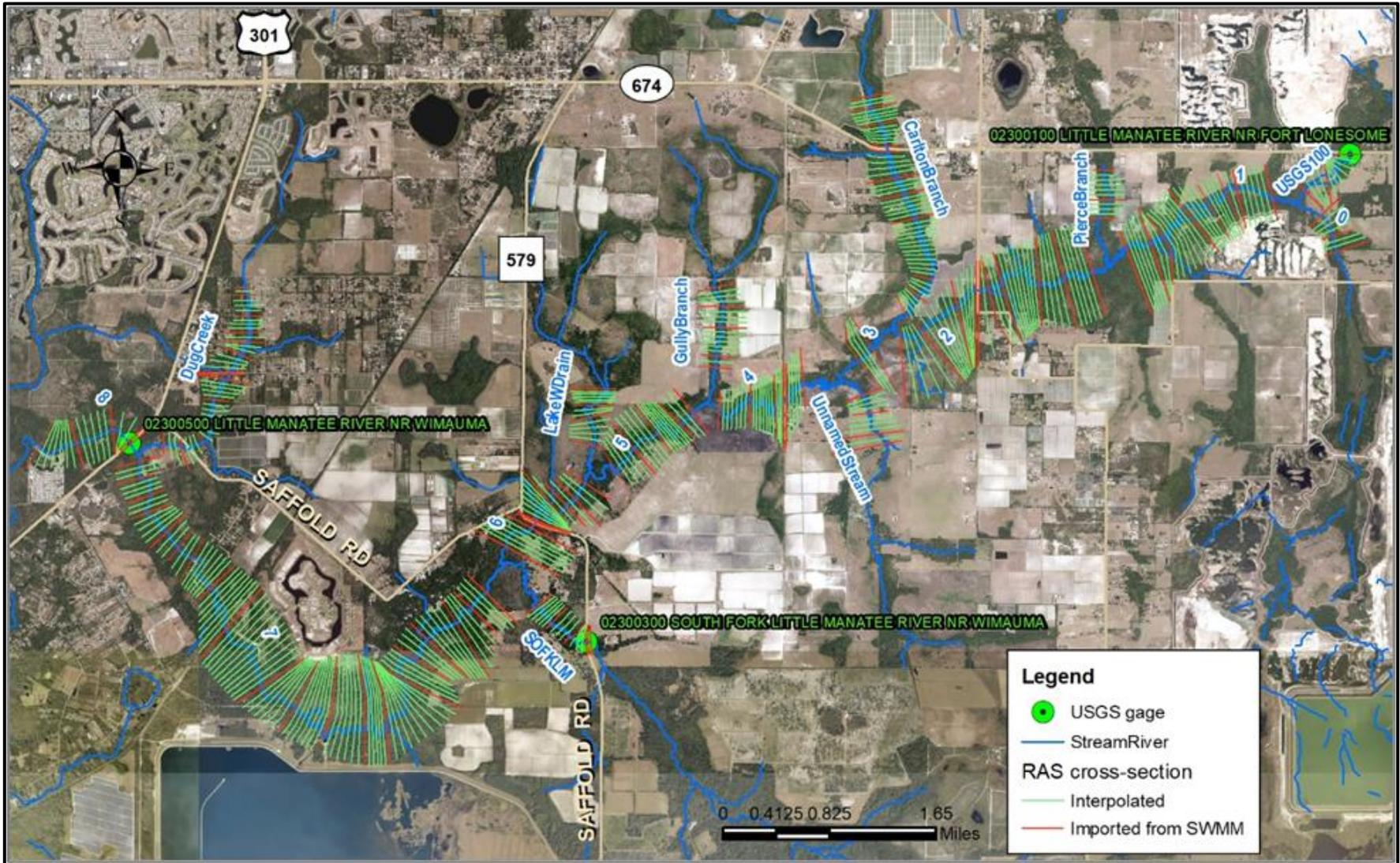
Figure 5-5. Seventeen river reaches (0 to 8 are the reaches for the main stem) and 478 cross sections in the 2018 Upper Little Manatee River HEC-RAS model. Locations of available US Geological Survey gages associated with the Upper Little Manatee River are shown.
