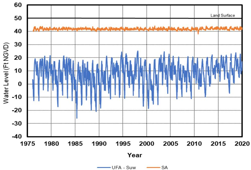
Figure 2-22. Water levels (in ft) from monitor wells (in ft) installed into the surficial and Upper Floridan aquifers at the District Regional Observation and Monitor-Well Program 50 site. Note 1 ft = 0.3 m.
