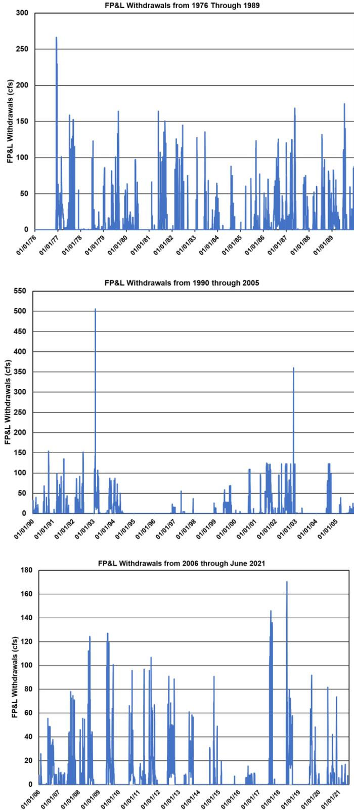
Figure 2-31. Daily surface water withdrawals by FP&L from the Little Manatee River from 1976 through June 2021. Top graph: 1976-1989, middle graph: 1990-2005, lower graph: 2006-June 2021.
