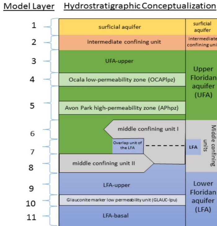
**Figure 2-29. Vertical discretization of the ECFTX Model.**
