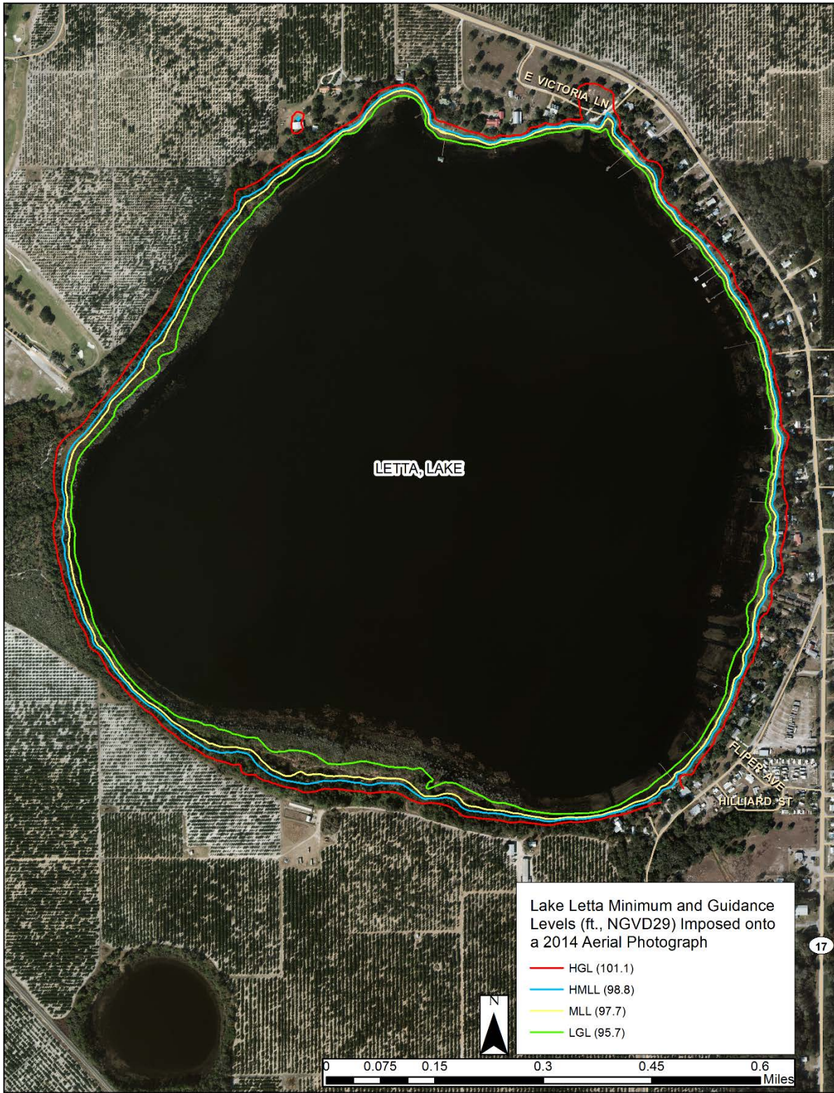
Figure 19: Lake Letta Revised Minimum and Guidance Level Contour Lines Imposed onto a 2014 Natural Color Aerial Photograph.
