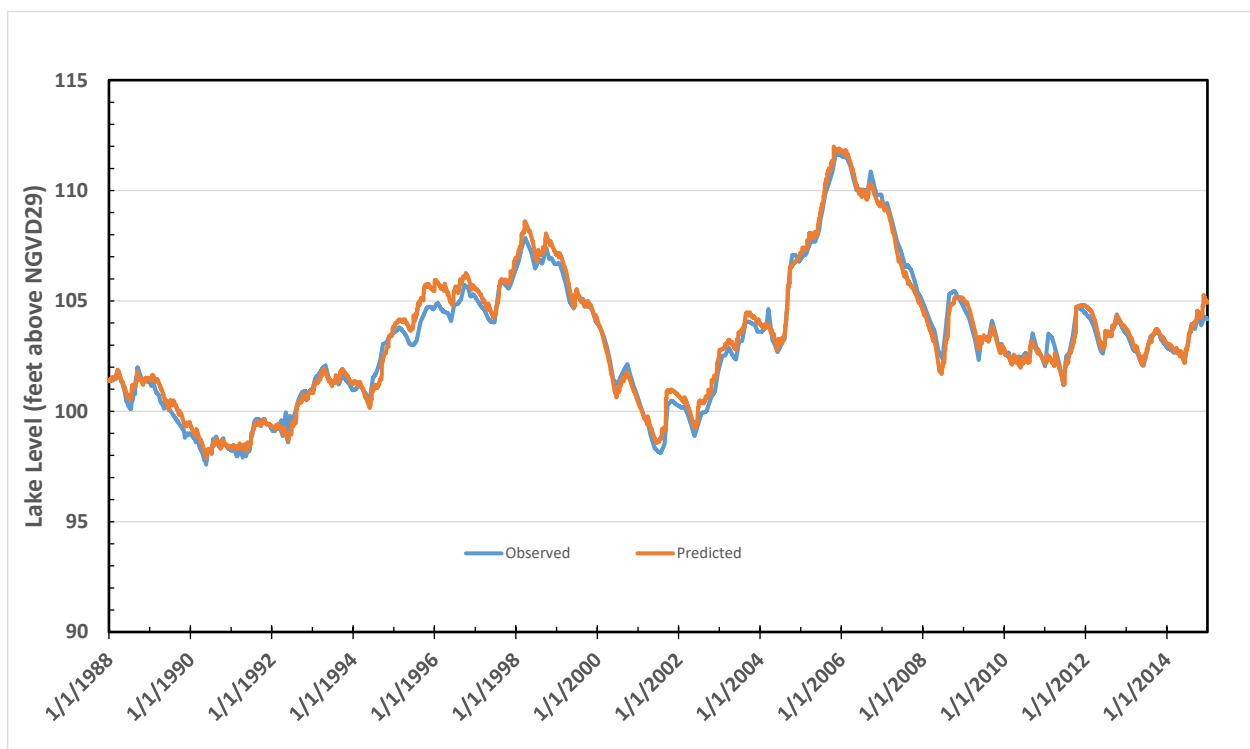
Figure 16. Modeled water levels predicted for the calibrated Lake Wales water budget (Predicted) and measured levels used for the model calibration (Data).
