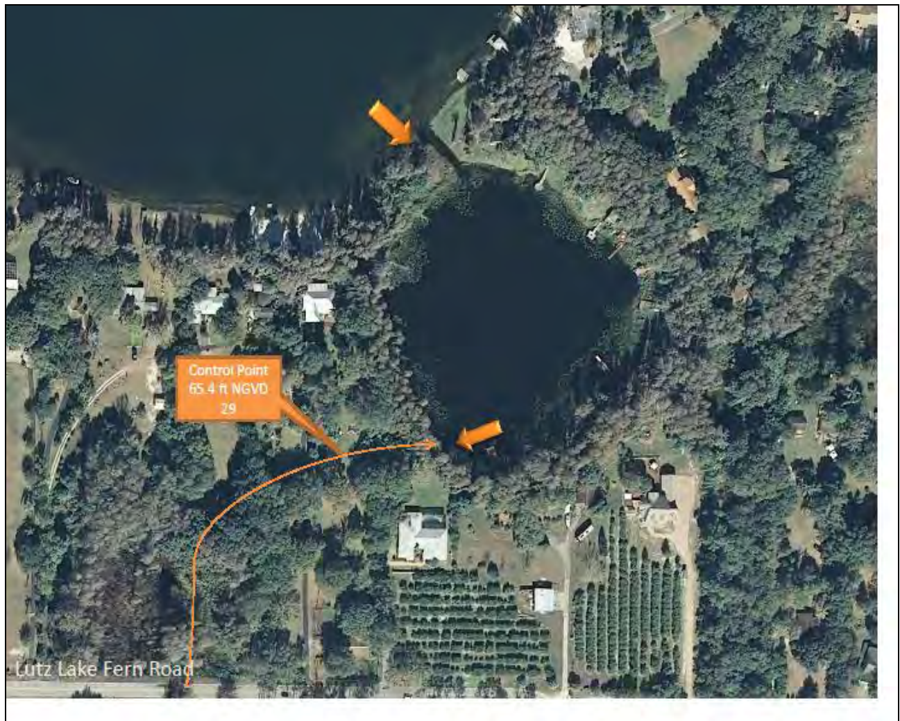
Figure 13 Discharge conveyance system from Lake Hobbs showing location of control point high running to a culvert under Lutz Lake Fern Road.
