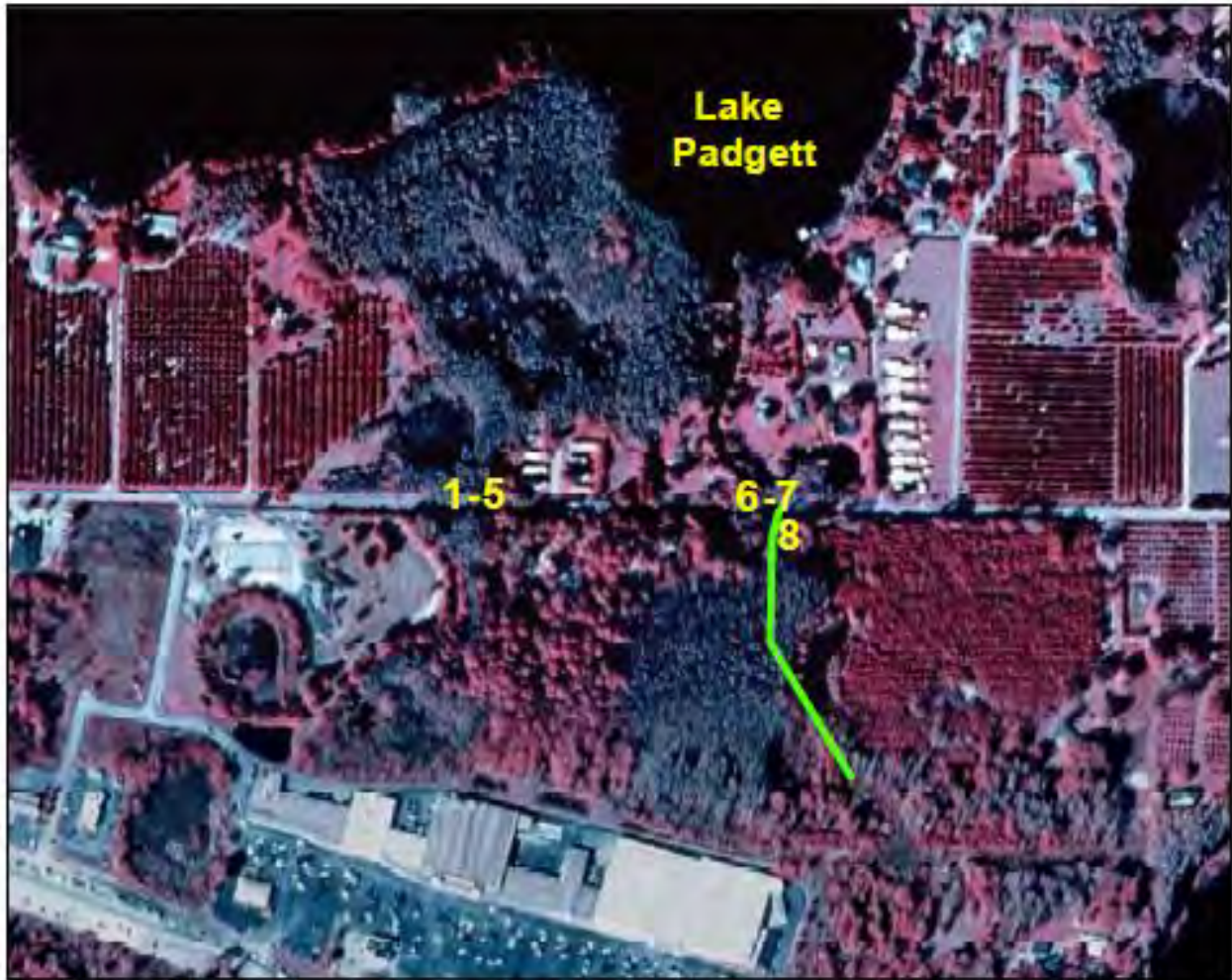
Figure 7. Outlet conveyance system for Lake Padgett in Pasco County, Florida. Numbered sites are described in Table 5.
