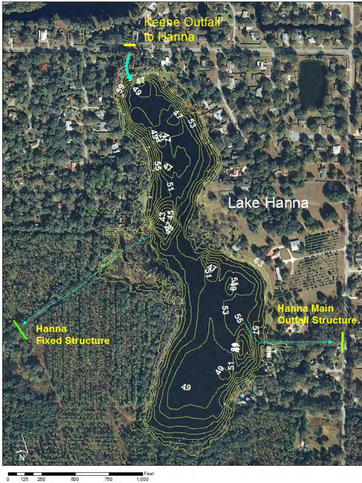
Figure 5. Two-foot contour lines within Lake Hanna. Values shown are elevations in feet as NGVD 29.
