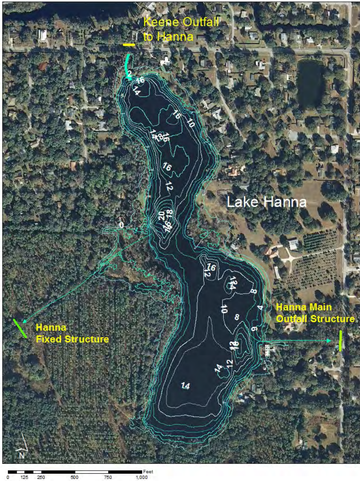
Figure 6. Bathymetric map of Lake Hanna showing approximate bottom depths at a lake stage of 63.0 NGVD 29.
