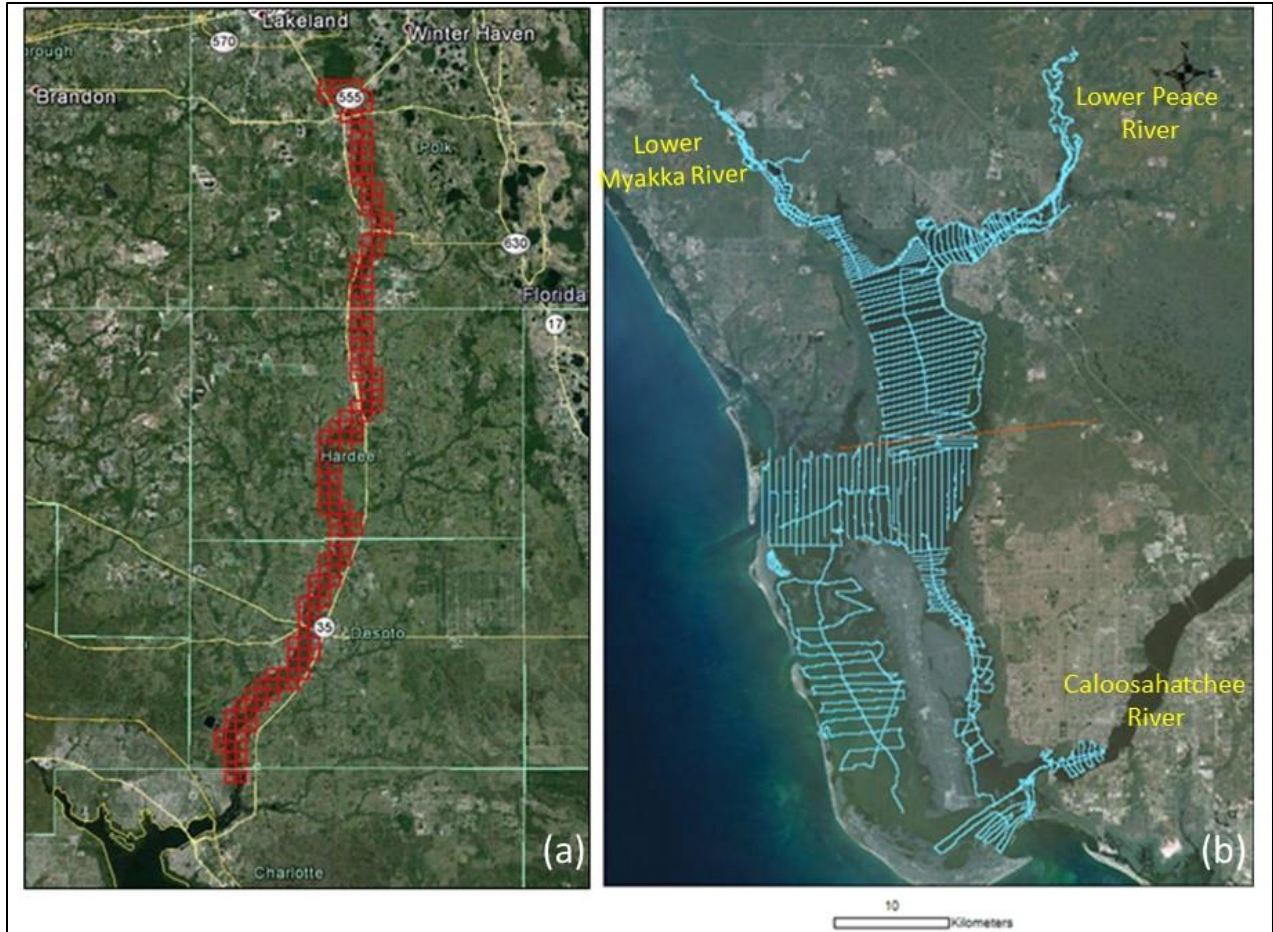
Figure 2-6. (a) LiDAR surveyed area for the Peace River and (b) shoreline and river cross-section bathymetric survey for the Lower Peace River, Myakka River, Caloosahatchee River, and Charlotte Harbor.
