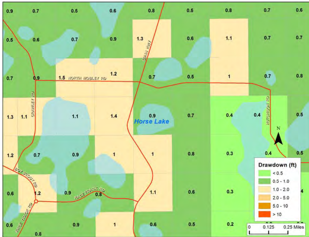
Figure 7. Predicted mean drawdown in the surficial aquifer due to TBW 90 mgd groundwater withdrawals.
