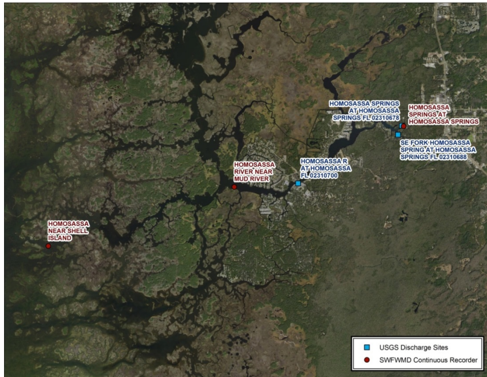
Figure 3-5. Location of the three District continuous recorders (red circles) for water quality on the Homosassa River. Blue squares show the locations of the USGS river discharge gages. The most upstream USGS gage – Homosassa Springs at Homosassa Springs, FL (No. 02310678) – also has a continuous nitrate sensor.
