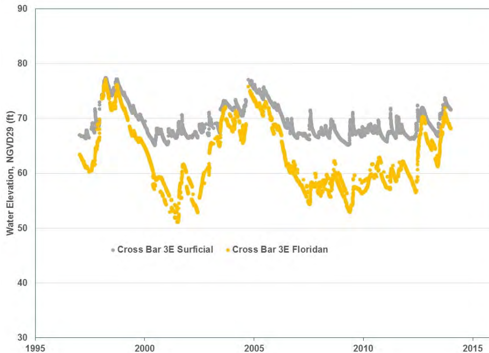
Figure 5. Water levels in the CB-3E Surficial and Floridan aquifer monitor wells.
