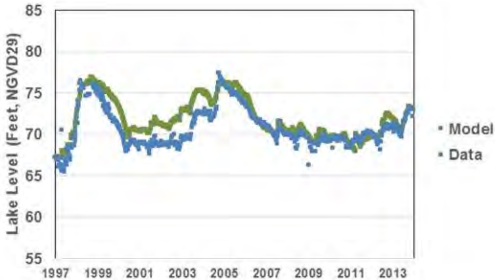
Figure 15. Measured lake levels (Data) and Historic water levels predicted with the calibrated Big Fish Lake model (Model).
