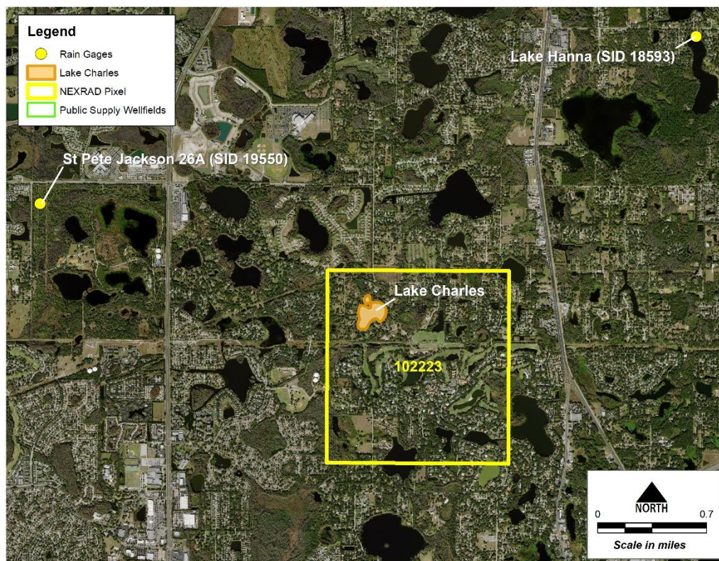
Figure 9. Rain gages and NEXRAD pixel used in the Lake Charles water budget model.
