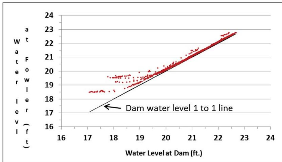
**Figure 12-5. Water levels at USGS gage at Fowler Avenue versus water levels at the USGS gage at the dam for periods with flows at the dam less than or equal to 27 cfs between June 1, 2008 and September 30, 2013. A one-to-one reference line is shown for water levels at the dam.**
