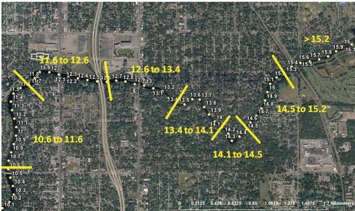
**Figure 4-31. Map of the lower river above kilometer 10 showing the seven segments by which vertical profile salinity data were analyzed.**
