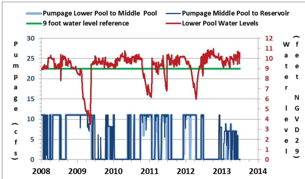
**Figure 12-3. Minimum flow pumpage rates from the lower pool to the middle pool of the TBC, from the middle pool of the TBC to the Hillsborouh River resevoir, water levels in the lower pool of the TBC, and a reference line at 9.0 feet for water levels in the lower pool of the TBC.**
