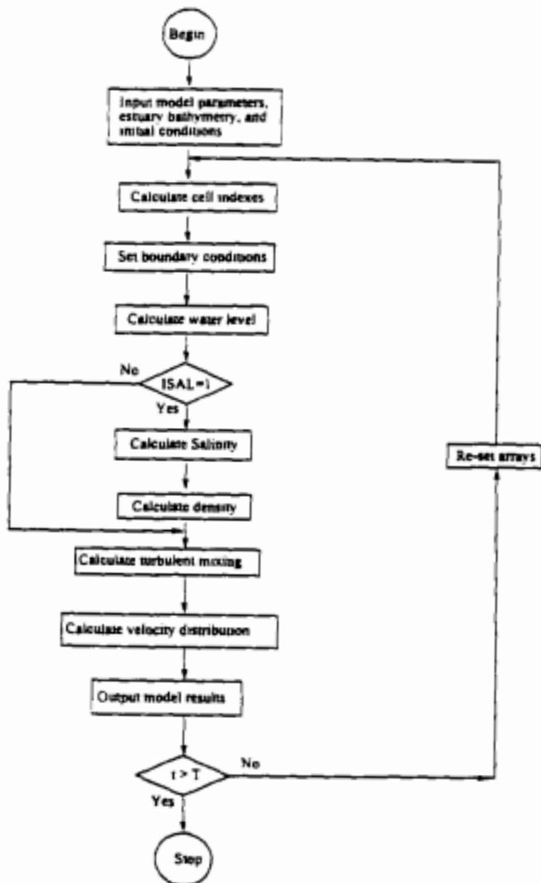
Figure 3 Flowchart of the model system LAMFE.
