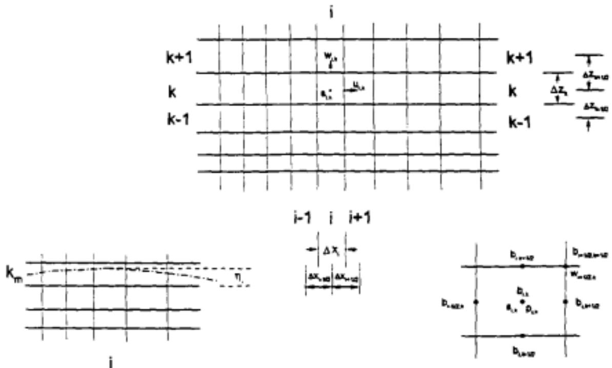
Figure 2 Rectangular, z-level grids for the laterally averaged 2-D model.
