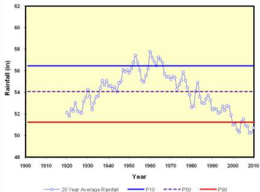
Twenty-year moving average rainfall for the Brooksville, Inverness, and Ocala National Weather Service stations. Horizontal lines represent the tenth, fiftieth and ninetieth exceedance percentiles of the twenty-year average values.
