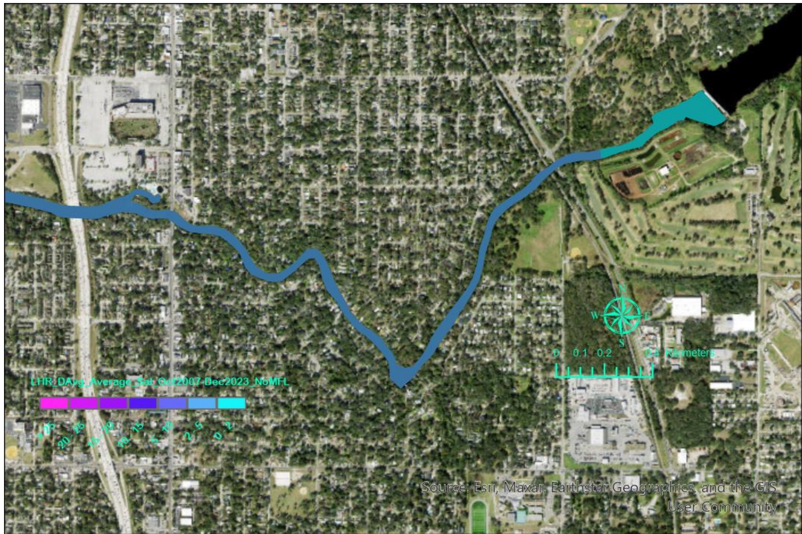
Figure A - 9. Average depth-averaged salinity in the upstream reach of the LHR during October 2007 – December 2023 for the no MFL flow condition.
