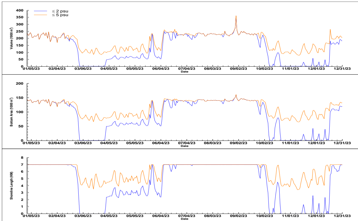
Figure 19. Simulated water volumes (top), bottom areas (middle), and shoreline lengths (bottom) of \leq 2 psu (blue) and \leq 5 psu (orange) between the dam and the confluence of the Sulphur Springs run in the LHR during January – December 2023 for the existing flow condition.
