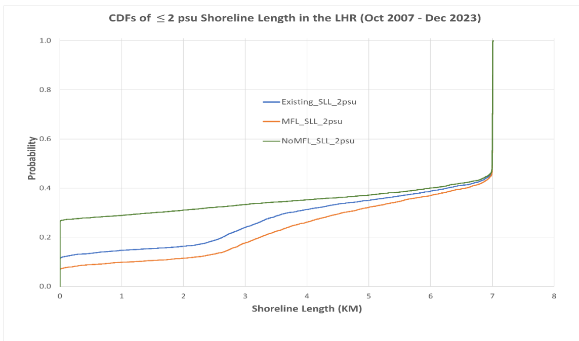
Figure 26. CDFs of simulated \leq 2 psu shoreline length for the existing, MFL, and no MFL flow conditions during Oct 2007 – Dec 2023 in the LHR between the dam and the Sulphur Springs confluence.
