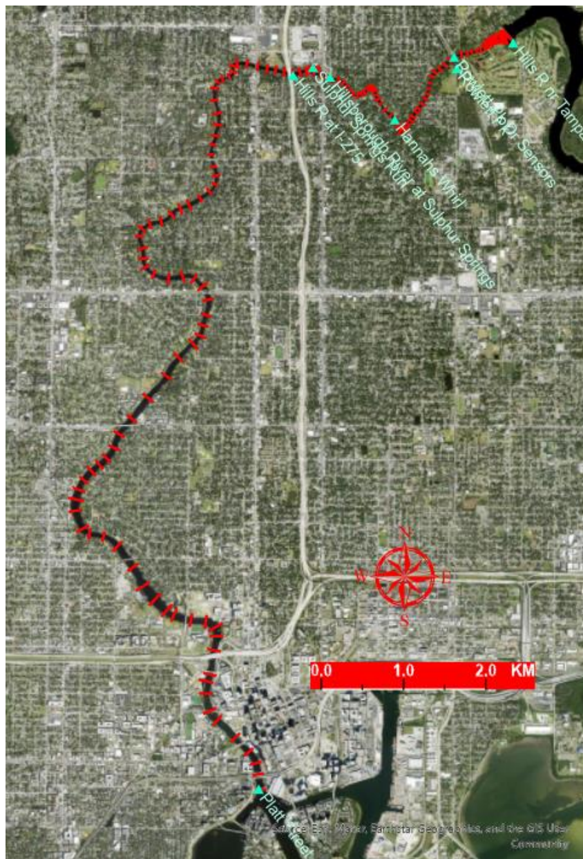
Figure 5. LAMFE model grids for the entire simulation domain, including the lower Hillsborough River and the Sulphur Springs run. Triangles are locations of the CTD data stations.
