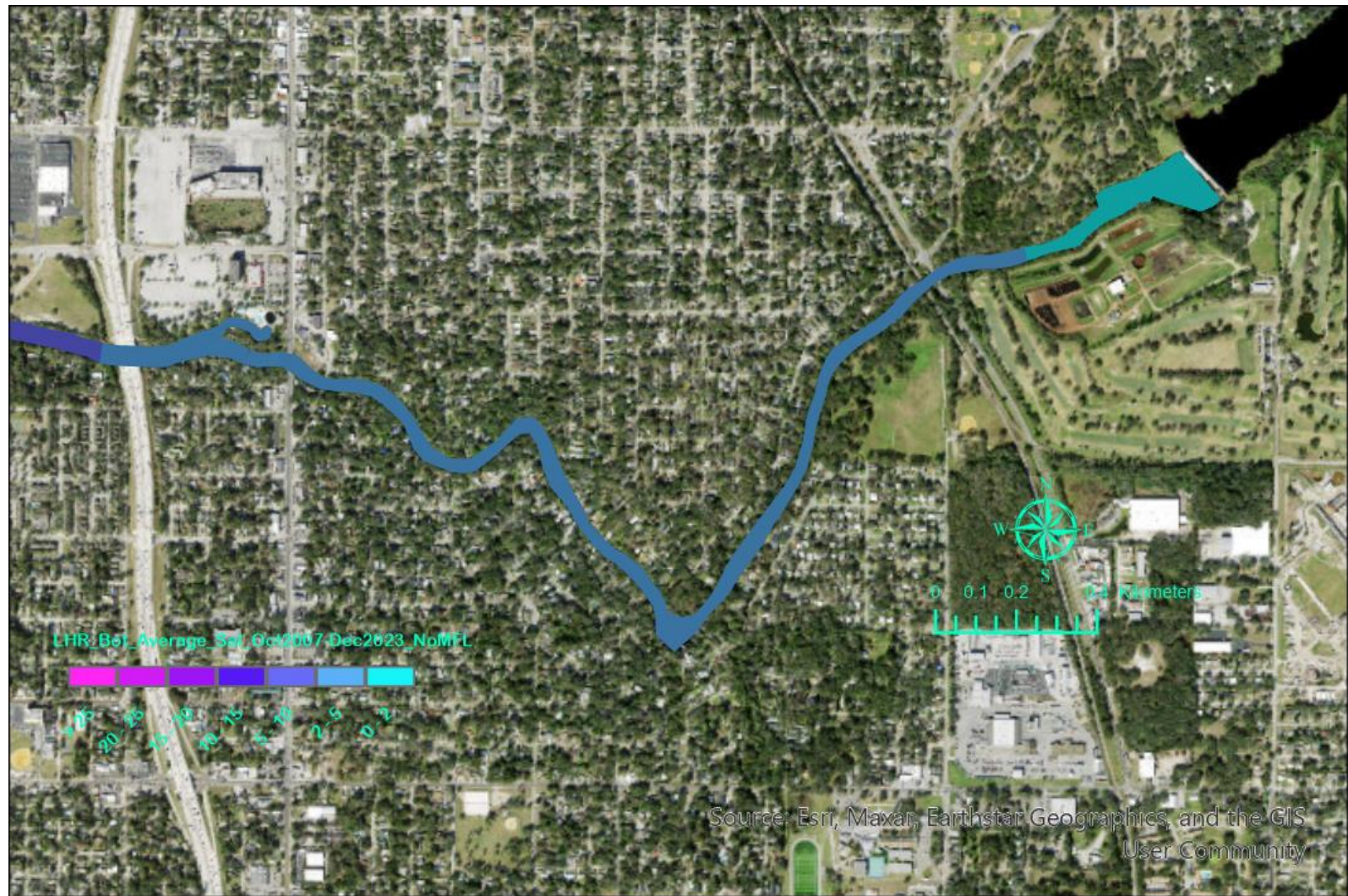
Figure A - 6. Average bottom-layer salinity in the upstream reach of the LHR during October 2007 – December 2023 for the no MFL flow condition.
