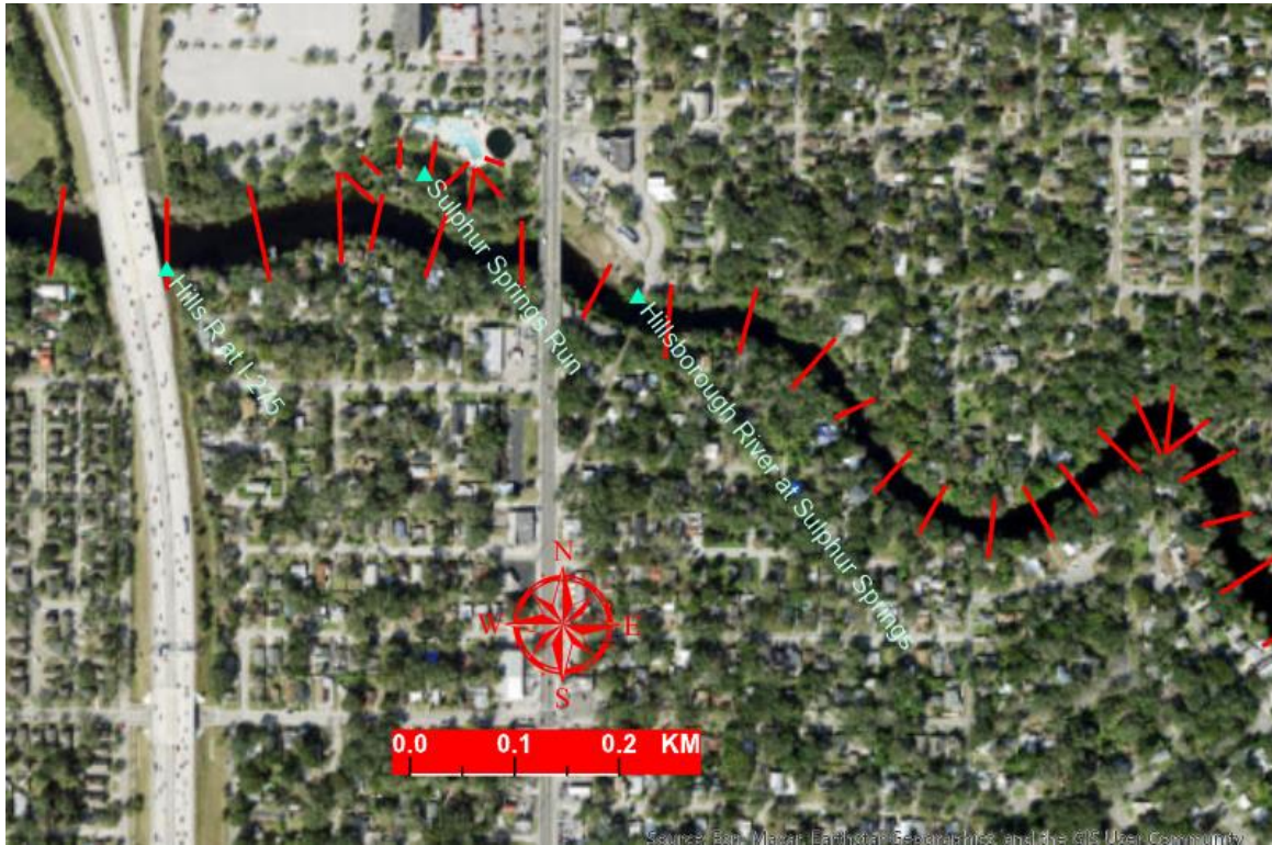
Figure 6. A zoom-in view of the model grids for the Sulphur Springs run and the segment of the LHR near the confluence of the run.
